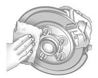
10. Remove any rust or dirt from the wheel bolts, mounting surfaces, and spare wheel.
