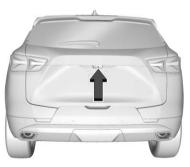
Dirt, snow, or other debris blocks the camera lens. Clean the lens with a soft damp cloth, or if equipped, with the Rear Camera Washer. See Rear Window Wiper/Washer
