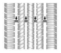
Treadwear indicators are one way to tell when it is time for new tires. Treadwear indicators appear when the tires have only 1.6 mm (1/16 in) or less of tread remaining. See *Tire Inspection* ♀ 293 and *Tire Rotation* ♀ 293.
