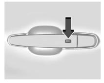
The remote key must be within 1 m (3 ft) of the liftgate or door being opened. Press the button on the door handle to unlock. See "Keyless Access Operation" in *Remote Key Operation*
