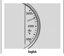
This gauge shows the engine oil temperature.
