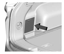
The rear compartment fuse block is behind a trim cover on the driver side of the rear storage compartment. Remove the trim cover to access the fuse block or visit your dealer.
