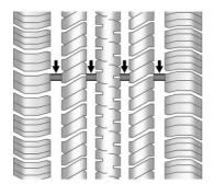
Treadwear indicators are one way to tell when it is time for new tires. Treadwear indicators appear when the tires have only 1.6 mm (1/16 in) or less of tread remaining. See *Tire Inspection* ⇒ 289 and *Tire Rotation* ⇒ 289.
