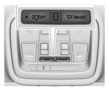
The dome lamp controls are in the overhead console.
