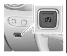
The vehicle has an Electric Parking Brake (EPB). The EPB can always be activated, even if the ignition is off. To prevent draining the battery, avoid repeated cycles of the EPB system when the engine is not running.
