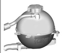
Check to see if coolant is visible in the coolant surge tank. If the coolant inside the coolant surge tank is boiling, do not do anything else until it cools down. See *Engine*Overheating \$ 275.
