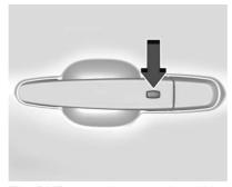
The RKE transmitter must be within 1 m (3 ft) of the liftgate or door being opened. Press the button on the door handle to open. See "Keyless Access Operation" in Remote Keyless Entry (RKE)
