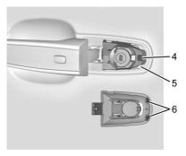
2. Insert the two tabs (6) at the back of the cap between the seal (5) and the metal base (4).
