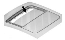
Dirt and debris may collect on the sunroof seal or in the track. This could cause an issue with sunroof operation or noise. It could also plug the water drainage system.
