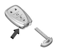
Remove the key by pressing the button on the side of the RKE transmitter near the bottom and pull the key out. Never pull the key out without pressing the button.
