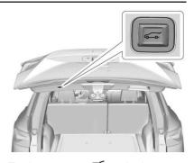
To close, press  $\longrightarrow$  on the bottom of the liftgate.
