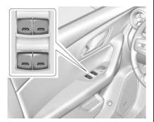
Using the window switch, press to open or pull to close the window.
