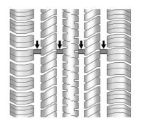
Treadwear indicators are one way to tell when it is time for new tires. Treadwear indicators appear when the tires have only 1.6 mm (1/16 in) or less of tread remaining. See *Tire Inspection* ⇔ 310 and *Tire Rotation* ⇔ 310.
