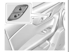
: Press to lock the doors. The indicator light in the switch will illuminate when locked.
