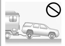
Towing the vehicle from the rear could damage it. Also, repairs would not be covered by the vehicle warranty. Never have the vehicle towed from the rear.
