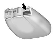
Press the button on the side of the RKE transmitter and pull the key out. Never pull the key out without pressing the button. Separate the two halves of the transmitter using a flat tool inserted into the area near the key slot.
