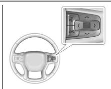
∧ or ∨ : Use the thumbwheel to scroll up or down in a list. Press the thumbwheel to select.
