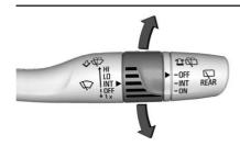
**INT:** Move the windshield wiper lever to INT. Turn the band up for more frequent wipes or down for less frequent wipes.
