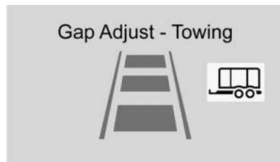
Far Gap Setting with Trailer
