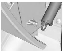
Disconnect the glove box door damper
