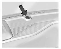
The light sensor is on top of the instrument panel. Do not cover the sensor.
