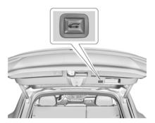
When closing the liftgate, press the button on the bottom of the gate.
