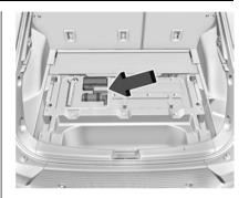
Thetire sealant can ister and compressor are secured with straps. Release the straps and remove the can ister and compressor.
