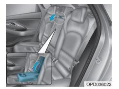
The armrest is located in the center of the rear seat. Use the strap in the center of the armrest to pull it down.
