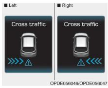
If the vehicle detected by the sensors approaches your vehicle, the warning chime will sound, the warning light on the outer side view mirror will blink and a message will appear on the LCD display.
