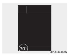
This gauge indicates the current outside air temperatures by 1°F (1°C).
