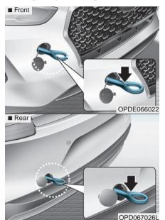
If towing is necessary, we recommend you have it done by an authorized HYUNDAI dealer or a commercial tow truck service If a towing service is not available in an emergency, your vehicle may be temporarily towed using a cable or chain secured to the emergency towing hook at the front (or rear) of the vehicle.
