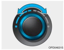
Turn the temperature control knob to the desired temperature. If the temperature is set to the lowest setting (Lo), the air conditioning system will operate continuously. After the interior has cooled sufficiently, adjust the knob to a higher temperature set point whenever possible. To turn the automatic operation off, select any button of the following:
