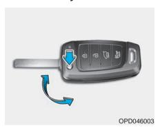
If the remote key does not operate normally, you can lock or unlock the driver's door by using the mechanical key.
