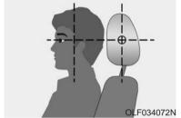
Adjust the head restraints so the middle of the head restraint is at the same height as the height of the top of the eyes.
