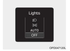
This indicator displays which exterior light is selected using the lighting control.
