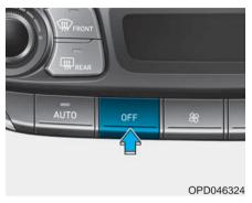
Push the OFF button to turn the climate control system off. You can still operate the mode and air intake buttons as long as the ignition switch is in the ON position.
