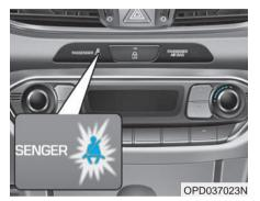
As a reminder to the front passenger, the front passenger's seat belt warning lights will illuminate for approximately 6 seconds each time you place the ignition switch to the ON position regardless of belt fastening.
