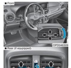
The outlet vents can be opened ( $\circledast$ ) or closed ( $\bigcirc$ ) separately using the thumbwheel.
