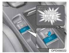
1. With the driver's door, engine hood and liftgate closed, fasten the driver's seat belt or depress the brake pedal and then press the [AUTO HOLD] switch. The white AUTO HOLD indicator will come on and the system will be in the standby position.
