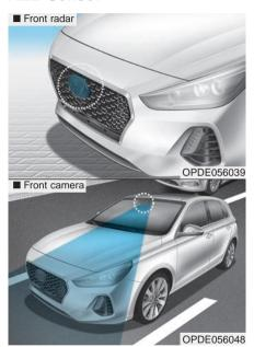
In order for the AEB system to operate properly, always make sure the sensor cover or sensor is clean and free of dirt, snow, and debris. Dirt, snow, or foreign substances on the sensor cover or sensor may adversely affect the sensing performance of the sensor.
