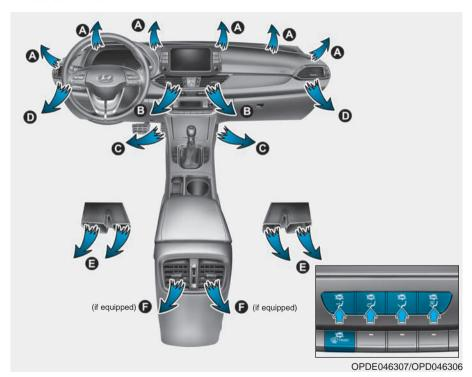
The mode selection button controls the direction of the air flow through the ventilation system. Air can be directed to the floor, dashboard outlets, or windshield. Five symbols are used to represent Face, Bi-Level, Floor, Floor-Defrost and Defrost air position.
