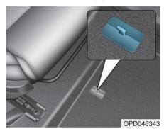
ALWAYS use the Floor Mat Anchors to attach the front floor mats to the vehicle. The anchors on the front floor carpet keep the floor mats from sliding forward.
