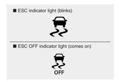
When the ignition switch is placed to the ON position, the ESC indicator light illuminates, then goes off if the ESC system is operating normally.
