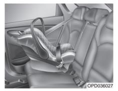
A rear-facing child seat provides restraint with the seating surface against the back of the child. The harness system holds the child in place, and in an accident, acts to keep the child positioned in the seat and reduce the stress to the neck and spinal cord.
