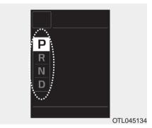
Shift indicator pop-up (if equipped) The pop-up indicates the current gear position displayed in the cluster for about 2 seconds when shifting into other positions (P/R/N/D).
