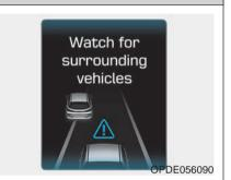
If the vehicle ahead (vehicle speed: less than 20 mph (30 km/h)) disappears to the next lane, the warning chime will sound and a message "Watch for surrounding vehicles" will appear. Adjust your vehicle speed for vehicles or objects that can suddenly appear in front of you by depressing the brake pedal.
