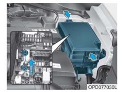
If the main fuse is blown, it must be removed as follows:
