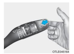
In the OFF position, pull the lever gently toward you to spray washer fluid on the windshield and to run the wipers 1-3 cycles. The spray and wiper operation will continue until you release the lever. If the washer does not work, you may need to add washer fluid to the washer fluid reservoir.
