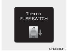
This warning message is displayed if the fuse switch located on the fuse box under the steering wheel is OFF. You should turn the fuse switch on.
