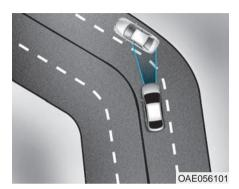
The AEB system may recognize a vehicle in the next lane when driving on a curved road.
