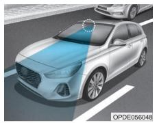
The Lane Keeping Assist System helps detect lane markers on the road with a camera at the front windshield, and assists the driver's steering to help keep the vehicle between lanes.
