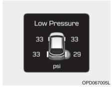
This warning message is displayed if the tire pressure is low. The corresponding tire on the vehicle will be illuminated.
