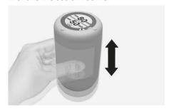
Remove the sealant bottle (2) cap and sealant bottle holder (5) cap and screw the bottle onto the sealant bottle holder.
