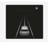
If the vehicle ahead and/or both lane markings are detected and your vehicle speed is below 120 mph (200 km/h), the green (②) indicator light appears on the cluster, and Lane Following Assist helps center the vehicle in the lane by assisting the steering wheel.
