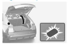
The cargo area lamp turns on when the liftgate is opened and off when the liftgate is closed.
