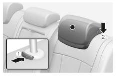
2. Adjust the head restraint to the appropriate height.
