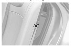
4. Pull up the seatback folding lever (1), then fold the seat toward the front of the vehicle (2).
