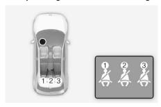
As a reminder to the rear passenger, the rear passenger's seat belt warning lights will illuminate for about 6 seconds each time the Start/Stop button is in the ON position regardless of belt fastening.
