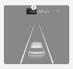
Highway Driving Assist indicator, whether there is a vehicle ahead and the selected distance level are displayed.
