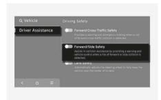
With the vehicle on, select **Setup** > **Vehicle** > **Driver Assistance** > **Driving Safety** > **Forward/Side safety** in the infotainment system to set whether to use each function.
