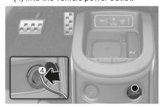
6. With the vehicle on (READY indicator on), switch on the compressor and let it run for about 5-7 minutes to on sealant up on proper pressure (For more information, refer to the "Tires And Wheels" section in chapter 2).
