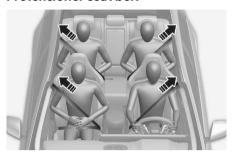
Your vehicle is equipped with driver's, front passenger's and rear passenger's (except rear center seat) pretensioner seat belts (retractor pretensioner). The pretensioner makes sure the seat belts fit tightly against your body in certain frontal or side collision(s). The pretensioner seat belts may be activated in some crashes where the frontal or side collision(s) is severe enough, together with the airbags.
