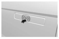
To lock your vehicle using the door handle touch sensor or the Smart Key:
