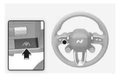
With the vehicle on, tap the Lane Driving Assist button located on the steering wheel to turn on Lane Following Assist. The gray or green (♠) indicator light will illuminate on the instrument cluster.
