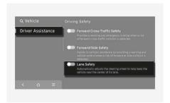
With the vehicle on, select **Setup** > **Vehicle** > **Driver Assistance** > **Driving Safety** > **Lane Safety** in the infotainment system to set whether to use each function.
