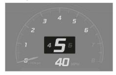
In the manual shift mode, this indicator informs which gear is desired while driving to save energy.
