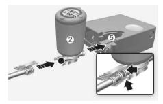
3. Make sure the compressor valve on the filling hose is locked.
