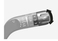
The rear window wiper and washer switch is located at the end of the wiper and washer switch lever. Turn the switch to the desired position to operate the rear wiper and washer.
