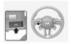
With the vehicle on, press and hold the Lane Driving Assist button (/⊕\) located on the steering wheel to turn on Lane Keeping Assist. The (/ᢛ\) indicator light illuminates on the instrument cluster. The Lane Driving Assist button also controls the Lane Following Assist when tapped (short press instead of a press and hold).
