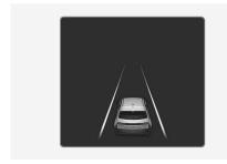
When lane markings (or road edges) are detected, the lane lines on the cluster changes from gray to white.
