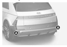
[A] Rear corner radar Refer to the picture above for the detailed location of the detecting sensors.
