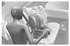
7. Double check that the retractor is in the "Automatic Locking" mode by attempting to pull more of the seat belt out of the retractor. If you cannot, the retractor is in the "Automatic Locking" mode.
