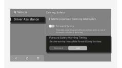
With the vehicle on, select Setup > Vehicle > Driver Assistance > Driving Safety > Forward Safety Warning Timing in the infotainment system to change the initial warning activation time for Forward Collision-Avoidance Assist. The warning time can be set to either "Standard" or "Late"
