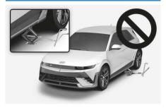
Never start or run the vehicle while an AWD vehicle is raised on a jack. The vehicle can slip or roll off of a jack causing serious injury or death to you or those nearby.
