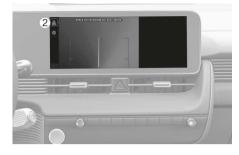
When you touch the icon (2), the top view is displayed on the screen and shows the distance from the vehicle in the back of your vehicle while parking.
