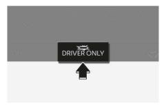
If you press the **DRIVER ONLY** button (indicator light ON), most of the air flow is directed toward the driver's seat.
