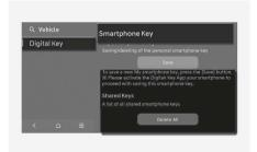
To delete all the registered digital key (smartphone), from the Settings menu select Setup > Vehicle > Digital Keys > Smartphone Key > Delete All in the infotainment system.
