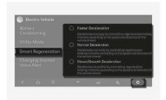
To adjust the regenerative braking level of the smart regeneration system, select Setup > Electric Vehicle > ♥ > Smart Regeneration in the infotainment system.
