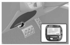
Inside the fuse panel cover, you can find the fuse label describing fuse names and ratings.
