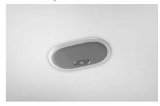
$\mathbf{x}$ : Press the button to turn on and off the rear room lamp.
