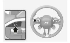
2. Push the + switch up or - switch down, and release it at the desired speed.
