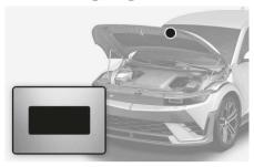
You can find out which air conditioning refrigerant is applied to your vehicle on the label located inside of the hood.
