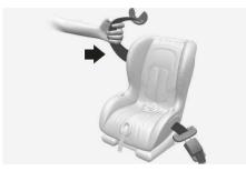
6. Push and pull on the Child Restraint System to confirm that the seat belt is holding it firmly in place. If it is not, release the seat belt and repeat steps 2 through 6.
