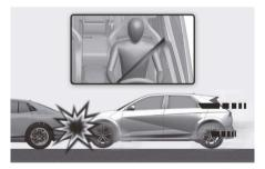
In certain low-speed collisions the airbags may not deploy. The airbags are designed not to deploy in such cases because they may not provide benefits beyond the protection of the seat belts.
