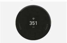
The distance to empty vary depending on many factors such as driving habits, power usage, driving conditions, and high voltage battery. The distance to empty may be increased or decreased than the certified figures as it reflects all the factors comprehensively. Check the distance to empty considering the following:
