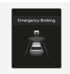
To warn the driver that emergency braking will be assisted, the "Emergency Braking" warning message will appear on the cluster, an audible warning will sound.
