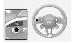
Press the Driving Assist (A) button to turn Manual Speed Limit Assist off. The Speed Limit (S) LIMIT) indicator will go off.
