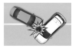
In an angled collision, the force of impact may direct the occupants in a direction where the airbags would not be able to provide any additional benefit, and thus the sensors may not deploy any airbags.
