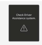
When High Beam Assist is not working properly, the "Check Driver Assistance system." warning message may appear, and the \(\text{\Lambda}\) warning light may illuminate on the instrument cluster. Have the system inspected by an authorized HYUNDAI dealer.
