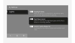
With the Start/Stop button in the ON position, select **Setup > Vehicle > Lights > High Beam Assist** to turn on High Beam Assist and deselect to turn off the function
