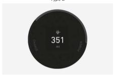
The distance to empty is the estimated distance the vehicle can be driven with the remaining electric energy.
