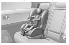
A forward-facing Child Restraint System provides restraint for the child's body with a harness. Keep children in a forward-facing Child Restraint System with a harness until they reach the top height or weight limit allowed by your Child Restraint System's manufacturer.
