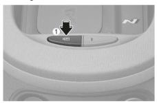
Press the Parking/View button (1) while the gear is in P (Park), D (Drive) or N (Neutral) to turn on the Rear View Monitor.
