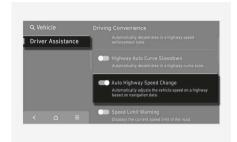
With the vehicle on, select **Setup** > **Vehicle** > **Driver Assistance** > **Driving Convenience** > **Highway Auto Speed Change** from the infotainment system to turn on Navigation based Smart Cruise Control and deselect to turn off the function.
