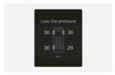
This warning message appears if the tire pressure is low. The corresponding tire on the vehicle is illuminated.
