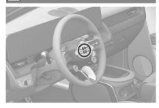
Detach the speed restriction label from the sealant bottle, and place it in a highly visible place inside the vehicle such as on the steering wheel to remind the driver not to drive too fast.
