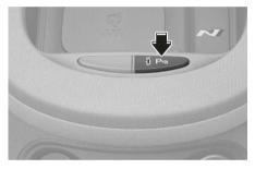
Press and hold the Parking Safety (P<sup>\*/±</sup>) button more than 2 seconds, to turn the Parking Collision-Avoidance Assist on or off.
