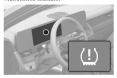
The TPMS Malfunction Indicator ((L)) illuminates after it blinks for about one minute when there is a problem with the Tire Pressure Monitoring System.
