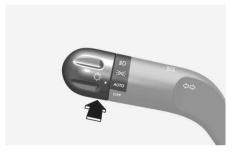
To turn on the high beam headlight, push the lever away from you. The lever returns to its original position.
