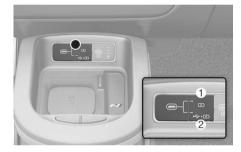
Press the USB port selection button while the vehicle is running. Press the upper portion of the button (1) to charge an electronic device. Press the lower portion of the button (2) to charge and listen to music with a media storage device. The USB port can be used after either indicator light turns on.
