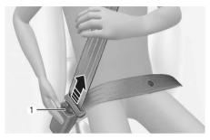
The belt should automatically draw back into the retractor. If this does not happen, check the belt is not twisted, then try again.
