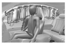
Side and curtain airbags are designed to inflate when an impact is detected by side collision sensors depending on the severity of impact resulting from a side collision.
