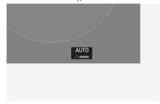
The smart regeneration system turns on and the regenerative braking level is displayed as 'AUTO'.
