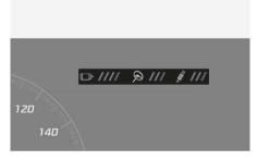
The main settings of CUSTOM mode is displayed at the top of the cluster. The CUSTOM mode can be set on the infotainment system.
