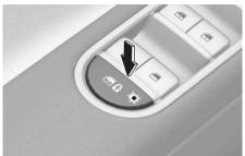
When the electronic child safety lock button is pressed and the indicator light on the button illuminates, the rear doors cannot be opened from inside the vehicle.
