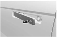
The doors will lock automatically and the handles will slide in after 30 seconds unless a door is opened.
