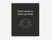
If the driver takes their hands off the steering wheel for several seconds, the "Keep hands on steering wheel" warning message appears on the instrument cluster, and an audible warning sounds in stages.
