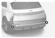
[A] Rear corner radar Refer to the picture above for the detailed location of the detecting sensors.
