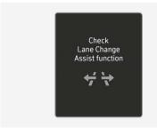
When Highway Driving Assist is not working properly, the "Check Driver Assistance system." or "Check Lane Change Assist function." warning message will appear, and the master (A) warning light appears on the instrument cluster. If this occurs, have your vehicle inspected by an authorized HYUNDAI dealer.
