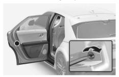
In case of emergency such as when the battery is discharged, the only way to lock the door(s) is with the mechanical key from the outside key hole.
