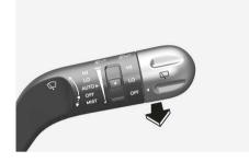
In the **OFF** position, pull the lever gently toward you to spray washer fluid on the windshield and to run the wipers 1-3 cycles. The spray and wiper operation continues until you release the lever. If the washer does not work, you may need to add washer fluid to the washer fluid reservoir.
