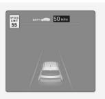
Manual Speed Limit Assist or Smart Cruise Control assists the vehicle to adjust its speed according to the speed limit. When the cruising speed is set as same as the speed limit, the vehicle automatically adjusts its speed if the speed limit changes. The function operates on the road which has a speed limit of 45 mph (70 km/h) or higher. When the function is active, the cruising speed on the instrument cluster appears in green.
