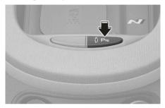
Press the Parking Safety (P<sup>\*\*\*</sup>) button to turn on Forward/Reverse Parking Distance Warning. Press the button again to turn off the function.
