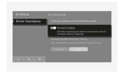
With the vehicle on, select **Setup** > **Vehicle** > **Driver Assistance** > **Driving Safety** in the infotainment system to set whether to use each function.
