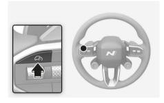
To turn Smart Cruise Control off, press the Driving Assist (A) button.
