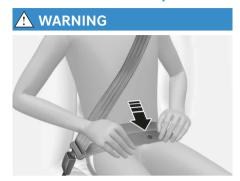
Improperly positioned seat belts may increase the risk of serious injury in an accident or sudden stop. Take the following precautions when adjusting the seat belt:
