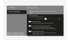
With the vehicle on, select **Setup** > **Vehicle** > **Driver Assistance** > **Warning Methods** in the infotainment system to select following:
