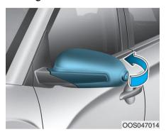
To fold the side view mirrors, grasp the housing of the mirror and then fold it inwards.
