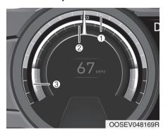
When ECO mode or ECO+ mode (if equipped) is enabled, the speedometer display includes a Smart ECO Pedal Indicator. The indicator encourages efficient driving by displaying the desired acceleration to achieve optimum range efficiency.
