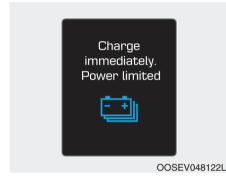
When the high voltage battery level reaches below 3%, this warning message is displayed.
