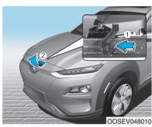
3. Go to the front of the vehicle, raise the hood slightly, push the secondary latch (1) inside of the hood center and lift the hood (2).
