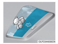
If the sunroof senses any obstacle while it is closing automatically, it will reverse direction then stop to allow the object to be cleared.
