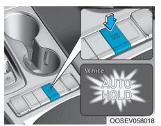
With the driver's door, hood and liftgate closed, depress the brake pedal and then press the [AUTO HOLD] switch. The white AUTO HOLD indicator will come on and the system will be in the standby position.
