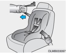
4. Pull the shoulder portion of the seat belt all the way out. When the shoulder portion of the seat belt is fully extended, it will shift the retractor to the "Automatic Locking" (child restraint) mode.
