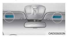
Air bag warning labels, required by the U.S. National Highway Traffic Safety Administration (NHTSA), are attached to alert the driver and passengers of potential risks of the air bag system. Be sure to read all of the information about the air bags that are installed on your vehicle in this Owners Manual.
