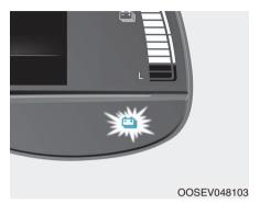
When there are only 2 bars remaining on the gauge, the SOC level is low. The warning lamp turns ON to alert you that the battery must be charged soon.
