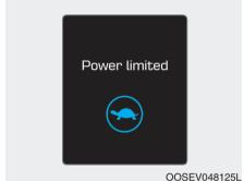
In the following cases, this warning message is displayed when the vehicle's power is limited for safety.
