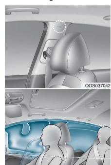
Curtain air bags are located along both sides of the roof rails above the front and rear doors.
