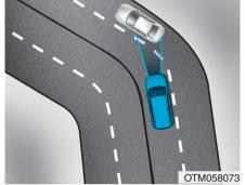
Your vehicle speed can be reduced due to a vehicle in the adjacent lane. Apply the accelerator pedal and select the appropriate speed. Check to be sure that the road conditions permit safe operation of the Smart Regeneration System.
