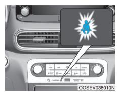
Front passenger's seat belt warning As a reminder to the front passenger, the front passenger's seat belt warning lights will illuminate for approximately 6 seconds each time you place the POWER button to the ON position regardless of belt fastening.
