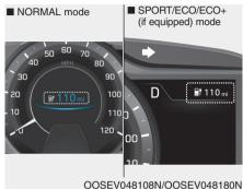
The EV range is the estimated distance the vehicle can be driven with remaining level of the high voltage battery.
