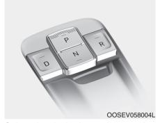
Select the desired gear by pressing one of the buttons on the Gear Shift Selector.
