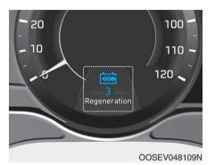
The selected regenerative braking level is displayed on the instrument cluster.
