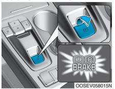
To apply the EPB (Electronic Parking Brake):
