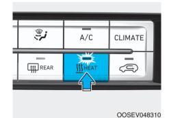
Push the HEAT button to turn the heater on (indicator light will illuminate).
