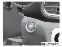
Whenever the front door is opened, the POWER button will illuminate and will go off 30 seconds after the door is closed.
