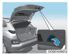
Lower the liftgate lid and press down until it locks. To be sure the liftgate lid is securely fastened, always check by trying to pull it up again without pressing the liftgate handle switch.
