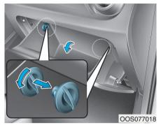
1. With the glove box open, remove the stoppers on both sides to allow the glove box to hang freely on the hinges.
