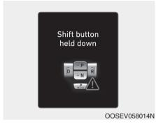
The message appears on the LCD display when the shift button is continuously pressed or there is problem with the button.
