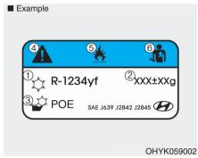
Each symbols and specification on the air conditioning refrigerant label is represented as below:
