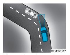
When coasting on the curve, the system may not detect the vehicle in your lane and the regenerative braking level will reduce automatically, making you feel that the vehicle is accelerating.
