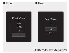
This indicator displays the windshield wiper mode when selected using the windshield wiper stalk.
