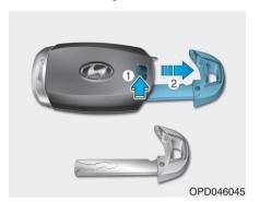
If the Smart Key does not operate normally, you can lock or unlock the driver's door by using the mechanical key. To remove the mechanical key from the smart key FOB, slide the release lever in the direction of the arrow (1) and then pull the mechanical key (2) outward.
