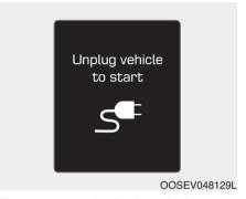
This message is displayed when you start the vehicle without unplugging the charging cable. Unplug the charging cable, and then turn on the vehicle.
