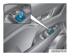
The driver can disable the power window switches on the rear passenger doors by pressing the power window lock switch.
