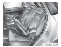
A rearward-facing child seat provides restraint with the seating surface against the back of the child. The harness system holds the child in place, and in an accident, acts to keep the child positioned in the seat and reduce the stress to the neck and spinal cord.
