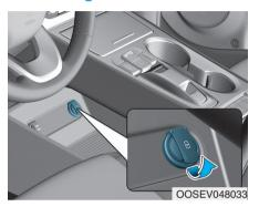
The USB charger is designed to recharge batteries of small size electrical devices using a USB cable.
