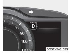
The indicator in the instrument cluster displays the gear position when the POWER button is in the ON position.
