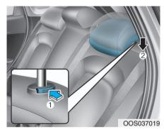
2. Lower the rear head restraints to the lowest position by pushing and holding the release button (1) and pushing down on the head restraint (2).
