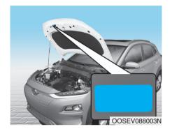
Air Conditioning refrigerant label You can find out which air conditioning refrigerant is applied to your vehicle on the label located inside of the hood.
