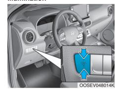
When the vehicle's position lights or headlights are on, press the illumination control button to adjust the brightness of the instrument panel illumination.
