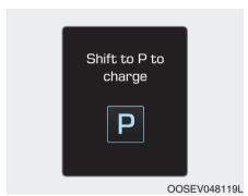
This message is displayed if you connect the charging cable without the gear in the P (Park) position.
