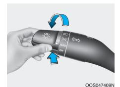
The High Beam Assist is a system that automatically adjusts the head-lamp range (switches between high beam and low beam) according to the brightness of other vehicles and
