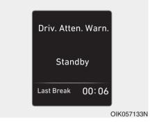
Driver Attention Warning system enters the ready status and displays the 'Standby' screen in the following situations.
