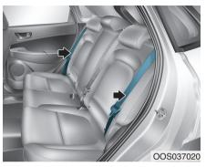
Locate the seatbelt toward the outboard position before folding down the seatback. If not, the seatbelt system may be interfered by the seatback.
