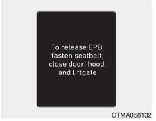
To release EPB, fasten seatbelt, close door, hood and liftgate
