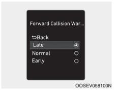
The driver can select the initial warning activation time on the LCD display.
