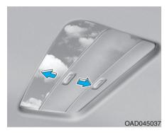
The sunshade can be open and closed manually using the sunshade handle. In addition, when you open the sunroof, if the sunshade is still closed, the sunshade will open automatically with the glass when the sunroof opens. When you close the sunroof, you must close the sunshade manually using the sunshade handle.
