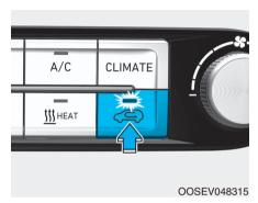
The air intake control button is used to select either Fresh mode (outside air) or Recirculation mode (cabin air).
