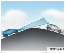
When coasting on an uphill or downhill, the system may not detect the vehicle in your lane and the regenerative braking level will reduce automatically, making you feel that the vehicle is accelerating.
