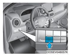
Use the button on the left hand side of the dash panel to activate/deactivate the Head-up display when the the POWER button is in the ON position or when the vehicle is in the ready ( ) mode.
