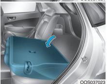
Remove the belt from the guide (1) and pull up the seatback folding lever (2), then fold the seat toward the front of the vehicle.
