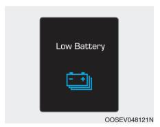
When the high voltage battery level reaches below 8%, this warning message is displayed.
