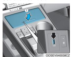
You can use an USB cable to connect audio devices to the vehicle USB port.
