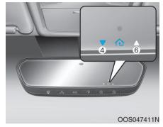
If both indicator (4) and (6) are flashing rapidly for about 5 seconds, the two way synchronization is completed.
