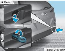
2. Remove the hole cover by pressing the lower part of the cover on the front or rear bumper.
