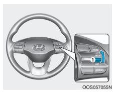
Push the switch (1) up (RES+). If the vehicle speed is over 20 mph (30 km/h), the vehicle will resume the preset speed.
