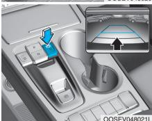
The Rear View Monitor will activate when the vehicle is in the ready ( ) mode and the gear is in the R (Reverse) position.
