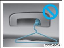
Do not hang other objects such as hangers or hard objects except clothes. Also, do not put heavy, sharp or breakable objects in the clothes pockets. In an accident or when the curtain air bag is inflated, it may cause vehicle damage or personal injury.
