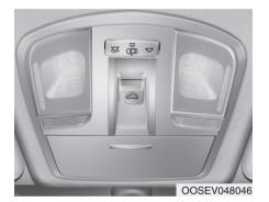
The sunroof can be opened, closed, or tilted when the POWER button is in the ON position.
