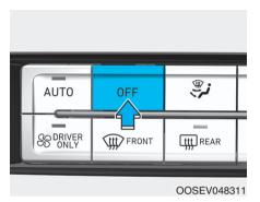
Push the OFF button to turn the climate control system off. You can still operate the mode and air intake buttons as long as the POWER button is in the ON position.
