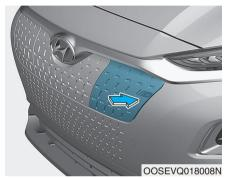
The charging door is located on the front of the vehicle and can be opened when the vehicle doors are unlocked.
