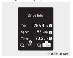
At the end of each driving cycle, the Driving Info message is displayed. This display shows the trip distance (1), average vehicle speed (2), driving time (3), charging time status (4) and climate time status (5).
