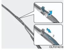
2. Lift up the wiper blade clip (1). Then pull down the blade assembly and remove it (2).
