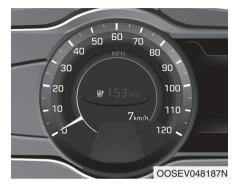
The sub speedometer is displayed on the cluster when you select 'Other features → Speedometer subscale' in the User Settings mode. The sub speedometer is not displayed if you deselect it in the User Setting mode.
