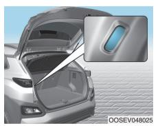
The luggage compartment lamp comes on when the liftgate is opened.
