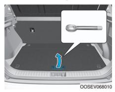
1. Open the liftgate, and remove the towing hook from the tool case.
