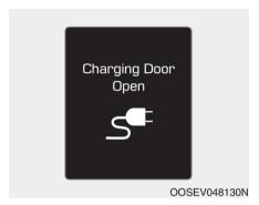
This message is displayed when you attempt to shift the vehicle out of P (Park) with the charging door open. You must close the charging door before driving the vehicle.
