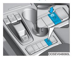
Push the button to turn OFF Reverse Parking Distance Warning system. The indicator light on the button will turn on.
