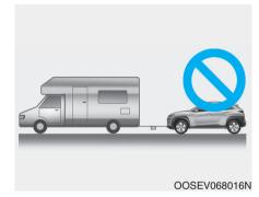
Your vehicle is not designed to be flat-towed behind a motor home. To avoid serious damage to your vehicle, do not flat-tow your vehicle.
