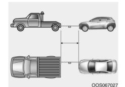
Use a towing cable or chain less than 16 feet (5 m) long. Attach a white or red cloth (about 12 inch (30 cm) wide) in the middle of the cable or chain for easy visibility.
