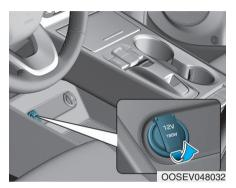
The power outlet is designed to provide power for 12V accessories or other devices designed to operate with vehicle electrical systems. The devices should draw less than 180 W with the vehicle in the ready ()
