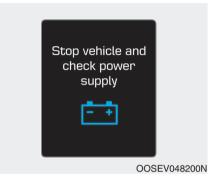
This warning message is displayed when a failure occurs in the power supply system.
