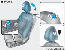
To reinstall the head restraint:
