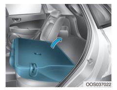
5. To use the rear seat, lift and unfold the seatback to the upright position. Push the seatback firmly until it clicks into place. Make sure the seatback is locked in place. Return the belt in the guide.
