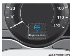
The level of regenerative braking can be selected by using the paddle shifters on the steering wheel. The level (0 to 3) is displayed in the lower portion of the cluster LCD display.
