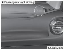
The purpose of the SRS is to provide the vehicle's driver and front passengers with additional protection than that offered by the seat belt system alone. The advanced SRS offers the ability to control the air bag inflation within two levels. A first stage level is provided for moderate-severity impacts. A second stage level is provided for more severe impacts.
