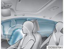
Your vehicle is equipped with a side air bag in each front seat.
