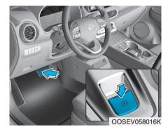
To release the EPB (Electronic Parking Brake), press the EPB switch in the following condition:
