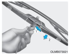
2. Press the clip (1) and slide the blade assembly downward (2).
