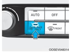
If you press the DRIVER ONLY (\$\mathbb{G}^{\text{priver}}\_{\text{ONLY}}\$) button, the indicator light will illuminate. In this mode the climate control system blows air primarily through the two left-most vents (nearest the driver).
