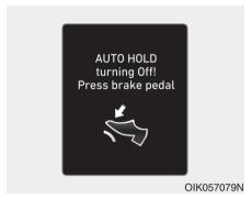
**AUTO HOLD turning Off! Press brake pedal**
