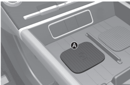
[A] Vehicle authentication pad (Wireless charging pad)
