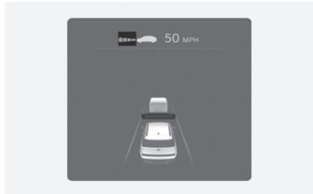
When Based on driving style is operating, the vehicle distance level and target distance will be displayed white based on the driving style.
