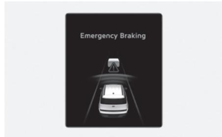
To warn the driver that emergency braking will be assisted, Forward Safety warning light (⚠️) blinking, the **"Emergency Braking"** warning message will appear on the cluster, an audible warning will sound, and the steering wheel will vibrate.
