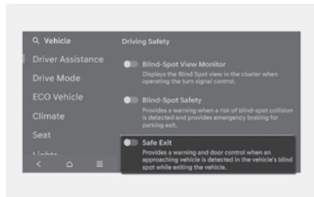
With the engine on, select **Setup** > **Vehicle** > **Driver assistance** > **Driving Safety** > **Safe Exit** from the Settings menu to turn on Safe Exit Assist and deselect to turn off the function.
