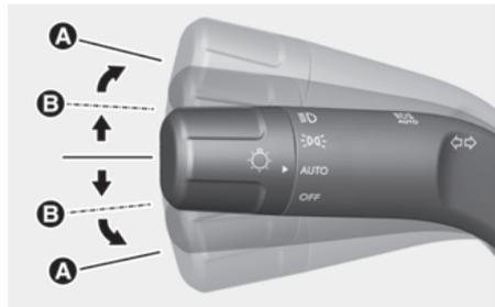
To signal a turn, push down on the lever for a left turn or up for a right turn in position (A).
