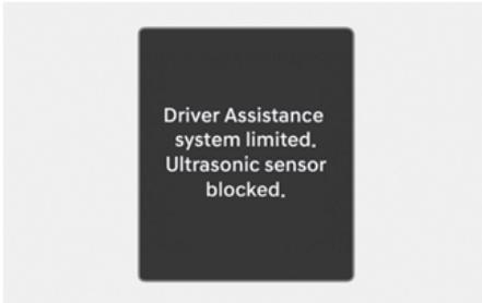
If this occurs the **"Driver Assistance system limited. Ultrasonic sensor blocked."** warning message appears on the instrument cluster. Parking Distance Warning operates properly when snow, rain or foreign material is removed. If Parking Distance Warning does not operate properly after obstruction (snow, rain, or foreign material) is removed (including trailer, carrier, etc., from the rear bumper), have your vehicle inspected by an authorized HYUNDAI dealer.
