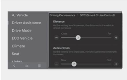
With the engine on, select **Setup > Vehicle > Driver Assistance > Driving Convenience > Smart Cruise Control** from the Settings menu in the infotainment system, you can change the vehicle distance, the acceleration, and the reaction speed manually.
