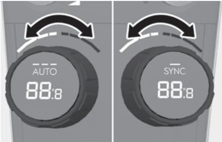
The temperature increases by turning the knob to the right (red side). The temperature decreases by turning the knob to the left (blue side).
