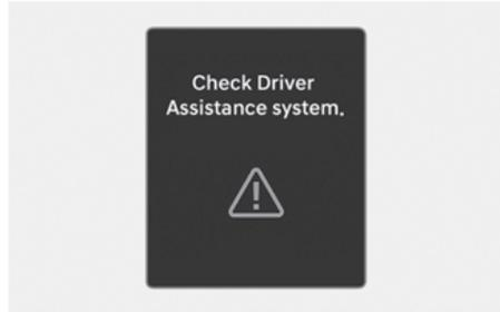
When Smart Cruise Control is not working properly, the "**Check Driver Assistance system.**" warning message will appear, and the "△" warning light will illuminate on the instrument cluster. Have your vehicle inspected by an authorized HYUNDAI dealer.
