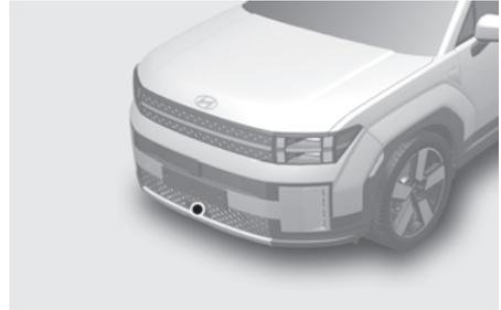
The front radar is mounted behind the front grill.
