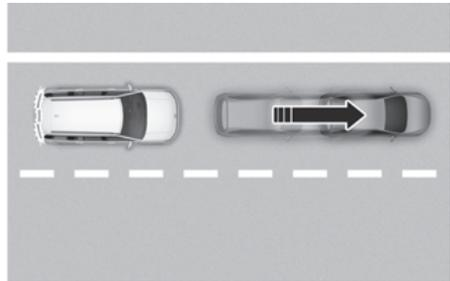
If the vehicle in front abruptly departs, Leading Vehicle Departure Alert may not operate properly.
