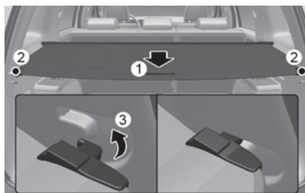
1. Pull the cargo security screen towards the rear of the vehicle by the handle (1).
