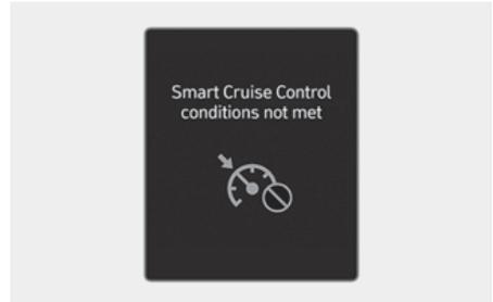
If the Driving Assist button, + switch, - switch or
