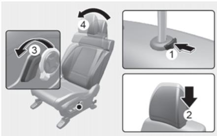
To remove the head restraint:
