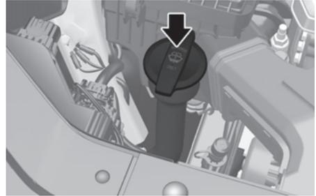
Check the fluid level in the washer fluid reservoir and add fluid if necessary. Plain water can be used during summer months if washer fluid is not available. However, use washer fluid with antifreeze in cold climates to prevent freezing.
