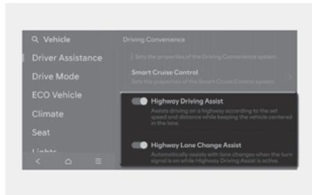
With the engine on, select or deselect **Setup > Vehicle > Driver Assistance > Driving Convenience > Highway Driving Assist** from the infotainment system to set whether to use each function.
