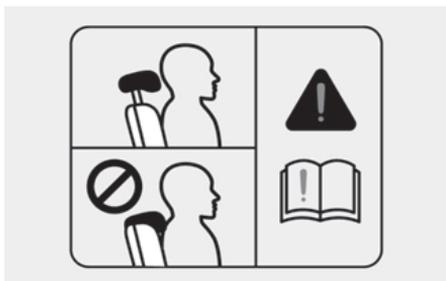
When a passenger is sitting on the 2nd row center seat, always raise the head restraint above the lowest stored position.
