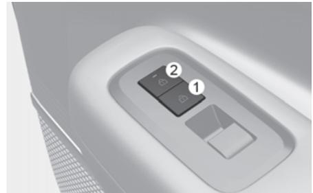
When pressing the (🔒) portion (1) on the switch, all vehicle doors are locked.
