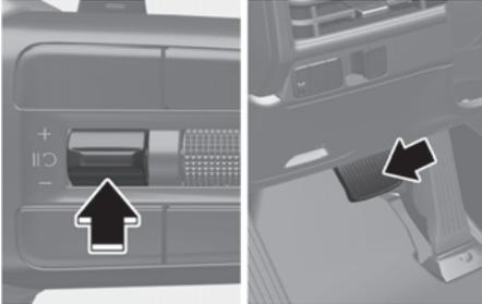
Press the II switch or depress the brake pedal to temporarily cancel Smart Cruise Control.
