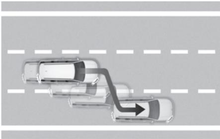
Highway Lane Change Assist function helps change lanes to the direction the driver slightly moves the turn signal switch if the function judges that lane change is possible.
