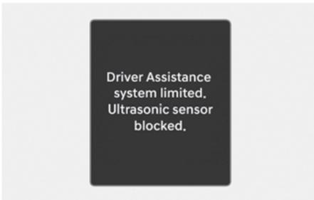
The "**Driver Assistance system limited. Camera obscured.**" or "**Driver Assistance system limited. Ultrasonic sensor blocked.**" warning message appears on the instrument cluster if the following situations occur:
