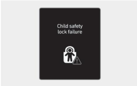
When electronic child safety lock does not work even though the button is pressed, the message will be displayed and an alarm will sound. If this occurs, have your vehicle inspected by an authorized HYUNDAI dealer.
