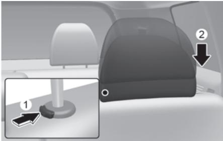
To reinstall the head restraint:
