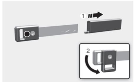
Turn the knob (2) of the mechanical key after removing the key protector (1).
