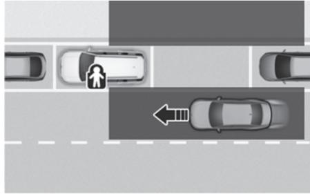
While your vehicle is stopped, if Safe Exit Assist detects a vehicle approaching the rear corner of your vehicle and a passenger opens a door, Safe Exit Assist may warn you with a warning message and a warning sound to help avoid a collision.
