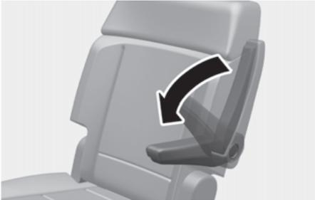
To adjust the armrest to a desired angle: Lift the armrest to slightly above the highest position, then lower it to the lowest position, then lift the armrest to position it to the desired angle.
