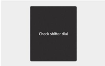
This message appears when there is a malfunction with the rotary gear shift dial. Have your vehicle inspected by an authorized HYUNDAI dealer.
