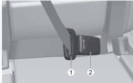
Insert the tongue plate (1) into the buckle (2) until an audible "click" is heard, indicating the latch is locked. Pull the shoulder portion of the belt to snug the belt across your hips and remove slack. Make sure the seat belt is not twisted.
