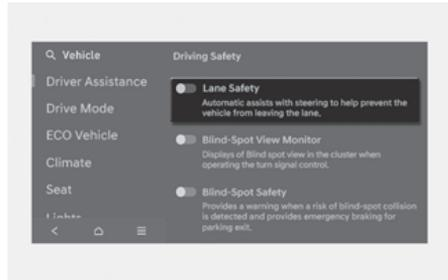
With the engine on, select **Setup** > **Vehicle** > **Driver Assistance** > **Driving Safety** > **Lane Safety** in the infotainment system to set whether to use each function.
