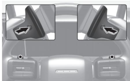
The paddle shifter is available when the gear is in the D (Drive) position. Pull the [+] or [-] paddle shifter once to shift up or down one gear and the system changes from automatic shift mode to manual shift mode. To change back to automatic shift mode from manual shift mode, do one of the followings:
