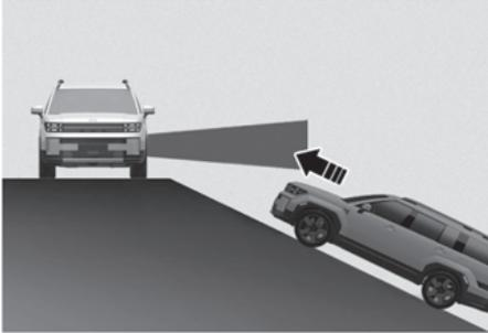
Rear Cross-Traffic Collision-Avoidance Assist may be limited when the vehicle is on an uphill or downhill slope, or near it, and may not detect the vehicle approaching from the left or right. If this occurs, the function may not warn the driver or control the brakes when necessary.
