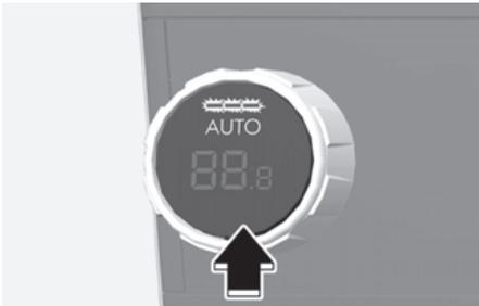
You can control the fan speed in three stages by pressing the **AUTO** button during automatic operation.
