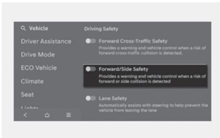
With the engine on, select **Setup** > **Vehicle** > **Driver Assistance** > **Forward/Side Safety** in the infotainment system to set whether to use each function.
