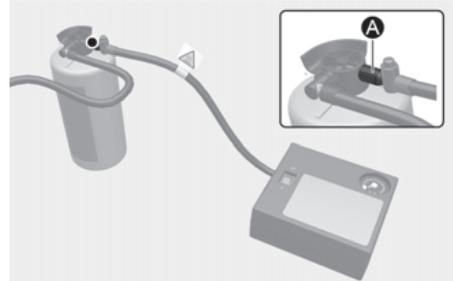
3. Unscrew the valve cap from the valve of the defective wheel and screw the filling hose (3) of the sealant bottle onto the tire valve.
