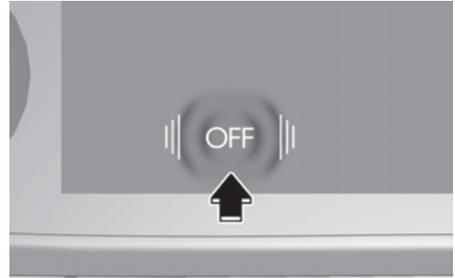
Press the **OFF** button to turn off the climate control system.
