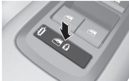
When the electronic child safety lock (ECSL) button is in the LOCK position and an approaching vehicle from the rear area is detected, the electronic child safety lock button will not unlock even if the driver presses the button to prevent the rear doors from opening.
