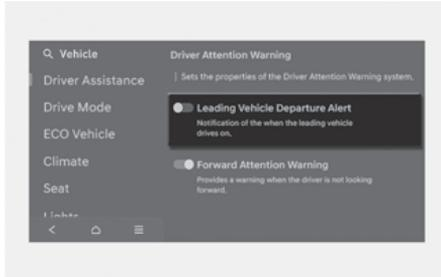
With the engine on, select or deselect **Setup > Vehicle > Driver Assistance > Driver Attention Warning** and then enable **Leading Vehicle Departure alert** in the infotainment system to set whether to use each function.
