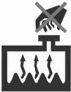
Never remove the engine coolant reservoir cap, radiator cap, or drain plug while the engine and radiator are hot. Hot coolant and steam may blow out under pressure, causing serious injury.
