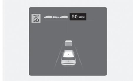
Manual Speed Limit Assist or Smart Cruise Control assists the vehicle to adjust its speed according to the speed limit. When the cruising speed is set as same as the speed limit, the vehicle automatically adjusts its speed if the speed limit changes. The function operates on the road which has a speed limit of 45 mph (70 km/h) or higher. When the function is active, the cruising speed on the instrument cluster appears in green.
