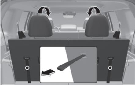
2. When using it as a seat, pull the seatback folding/unfolding strap to fully raise the seatback. Adjust the seatback to the desired angle, and release the upper angle adjustment strap to lock in place. Make sure the seatback is locked in place.
