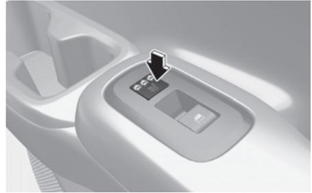
While the engine is running, press the seat warmer button to warm the rear seat. Press the button repeatedly to cycle through the seat warmer temperature from high, medium, low, and off.
