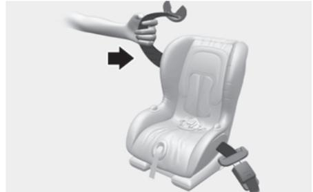
5. Remove as much slack from the belt as possible by pushing down on the Child Restraint System while feeding the shoulder belt back into the retractor.
