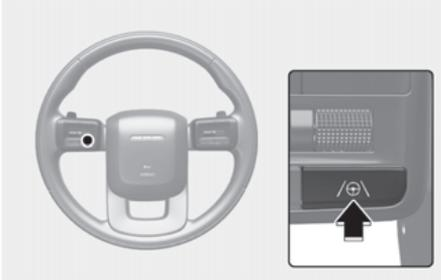
With the engine on, shortly press the Lane Driving Assist button located on the steering wheel to turn on Lane Following Assist. The gray or green (⊕) indicator light will illuminate on the instrument cluster.
