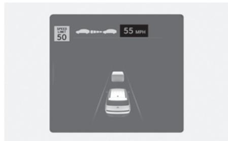
When driving at a speed higher than the displayed speed limit, the speed limit is displayed in red.
