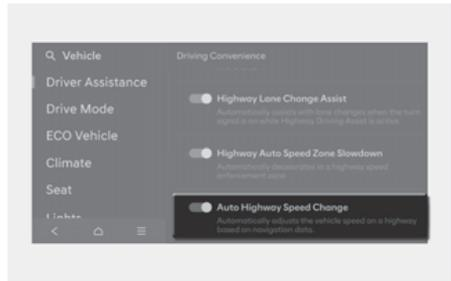
With the engine on, select **Setup > Vehicle > Driver Assistance > Driving Convenience > Highway Auto Speed Change** from the infotainment system to turn on Navigation based Smart Cruise Control and deselect to turn off the function.
