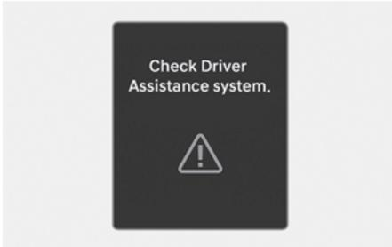
When Lane Following Assist is not working properly, the "**Check Driver Assistance system.**" warning message will appear on the instrument cluster for several seconds, and the master (⚠) warning light appears on the instrument cluster. If this occurs, have your vehicle inspected by an authorized HYUNDAI dealer.
