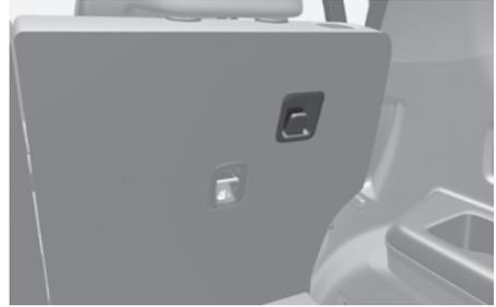
Hooks are located on the back of the 1st and 2nd row seatbacks.
