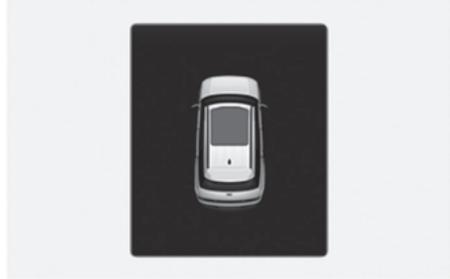
If the driver turns off the engine when the sunroof is not fully closed, the warning chime will sound for several seconds and the sunroof open warning will appear on the cluster display.
