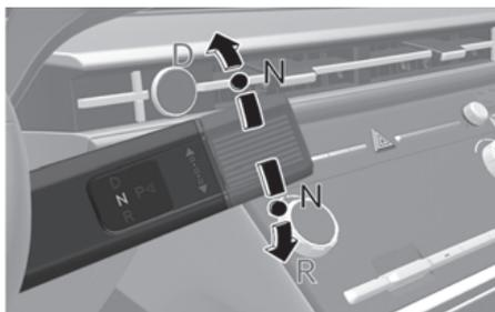
The wheels and transmission are not engaged.
