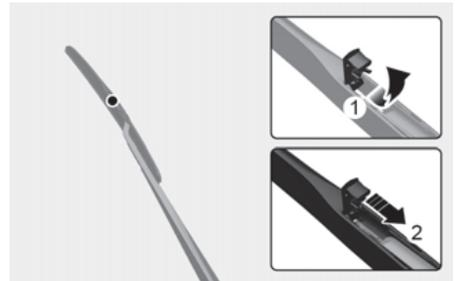
4. Install a new wiper blade assembly in the reverse order of removal.
