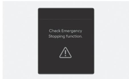
When Emergency Stop is not working properly, the "**Check Emergency Stopping function.**" warning message appears, and the master (⚠) warning light illuminates on the instrument cluster. If this occurs, have your vehicle inspected by an authorized HYUNDAI dealer.
