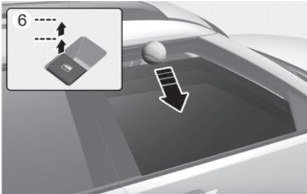
If a window senses any obstacle while it is closing automatically, it stops and lowers approximately 12 in. (30 cm) to allow the object to be cleared.
