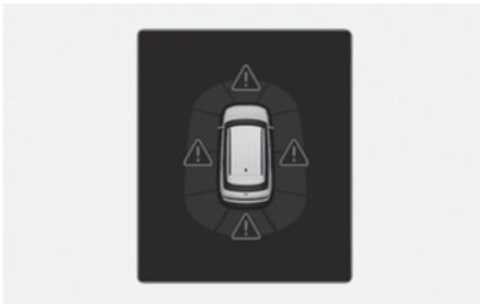
When the Parking Distance Warning is operating, if the function is not working normally or the ultrasonic sensor is blocked, the master warning light (
