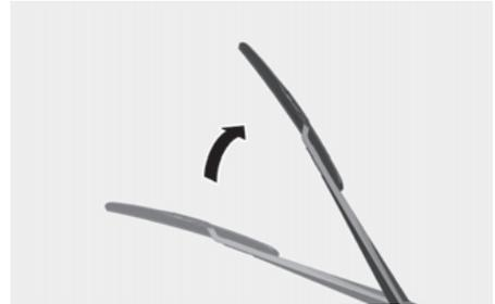
3. Lift up the wiper blade clip (1). Then pull down the wiper blade (2).
