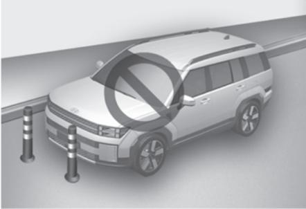
Remote Smart Parking Assist performance may reduce or collision with an obstacle may occur when there is a narrow object, circular pillar, square pillar, or a pillar surrounded by objects such as a fire extinguisher, etc., near the parking space. The driver should park the vehicle manually.
