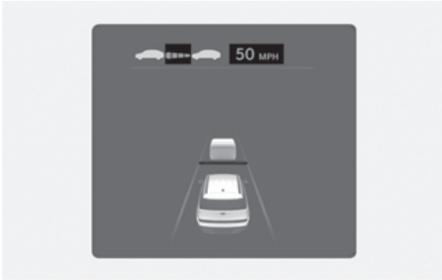
If you want to speed up temporarily without altering the set speed while Smart Cruise Control is operating, depress the accelerator pedal. While the accelerator pedal is depressed, the set speed, distance level and target distance will blink on the instrument cluster.
