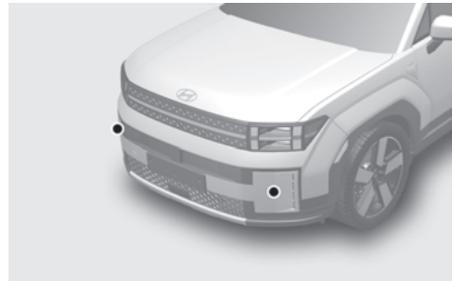
The front corner radars are mounted near the front corners of your vehicle above.
