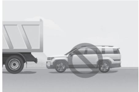
Do not use Remote Smart Parking Assist around vehicles with higher ground clearance, such as a bus, truck, etc. It may lead to a collision.
