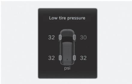
**TPMS is not a substitute for manually checking the tire pressure with a tire gauge. Changes in temperature affect tire pressure. Refer to "Check tire inflation pressure" in the Maintenance chapter for proper tire inflation and tire pressure measurement procedure.**
