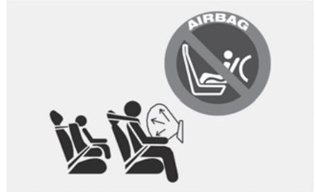
Even though your vehicle is equipped with the OCS, never install a Child Restraint System in the front passenger's seat. An inflating airbag may forcefully strike a child or child restraint resulting in serious or fatal injury.
