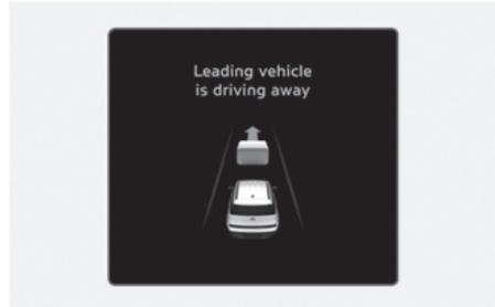
When a detected vehicle in front departs from a stop, Leading Vehicle Departure Alert will inform the driver by displaying the "**Leading vehicle is driving away**" message on the instrument cluster and an audible warning will sound.
