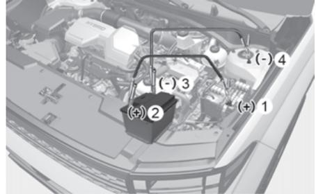
5. Connect the jumper cables in the exact sequence shown in the illustration. First connect one jumper cable to the red, positive (+) battery terminal of your vehicle (1).
