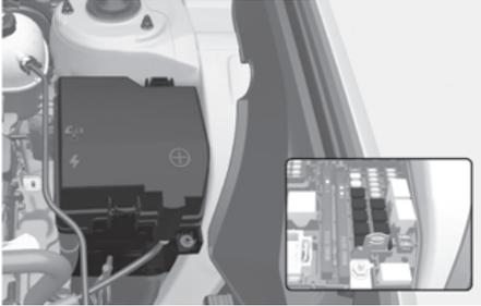
6. Check the removed fuse and replace it if it is blown. To remove or insert the fuse, use the fuse puller in the engine compartment fuse panel.
