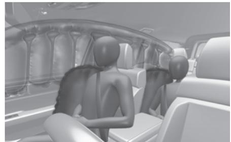
The side airbags are designed to deploy during certain side impact collisions, depending on the crash severity.
