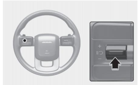
Press the **II** switch to temporarily pause the set speed limit. The set speed limit will turn off but the Speed Limit (**LIMIT**) indicator will stay on.
