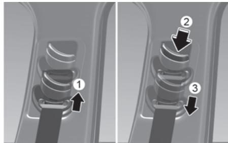
To adjust the height of the seat belt anchor:
