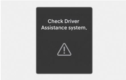
When High Beam Assist is not working properly, the "**Check Driver Assistance system**" warning message may appear, and the
