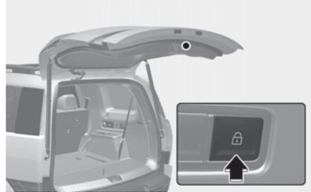
Press the power liftgate lock button while carrying the smart key. The liftgate closes and locks automatically. Additionally, all doors will lock.
