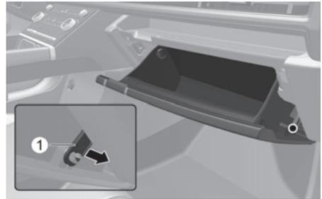
2. Push in both sides of the glove box to release the glove box stopper pins and allow the glove box to hang open.
