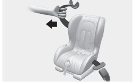
4. Slowly allow the shoulder portion of the seat belt to retract and listen for an audible "clicking" or "ratcheting" sound. This indicates that the retractor is in the Automatic Locking mode. If no distinct sound is heard, repeat Step 3 and 4.
