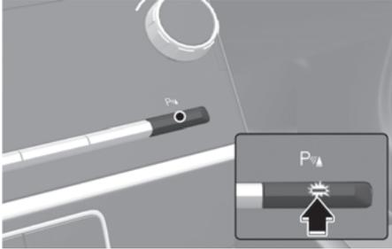
Press and hold the Parking Safety (P $\blacktriangle$ ) button more than 2 seconds, to turn the Parking Collision-Avoidance Assist on or off.
