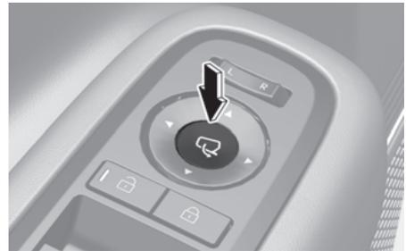
The side view mirrors can be folded or unfolded by pressing the button.
