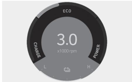
The hybrid system gauge indicates whether the current driving condition is fuel efficient or not.
