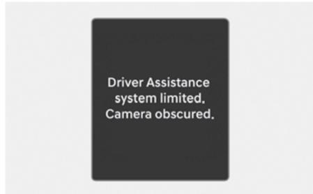
When the front windshield where the front view camera is located is covered with foreign material, such as snow or rain, it can reduce the detecting performance and temporarily limit or disable Intelligent Speed Limit Assist. If this occurs, the "**Driver Assistance system limited. Camera obscured.**" warning message, the (⚠) and (☒) warning lights will appear on the instrument cluster.
