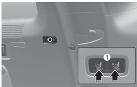
With the liftgate open, this feature allows you to conveniently fold the 2nd row seatback forward.
