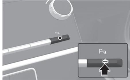
Press the Parking Safety (P<sub>▲</sub>) button to turn on Forward/Reverse Parking Distance Warning. Press the button again to turn off the function.
