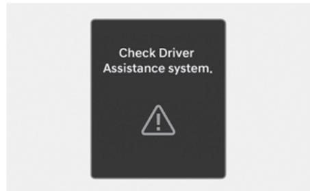
When Lane Keeping Assist is not working properly, the "**Check Driver Assistance system.**" warning message appears, the master (△) warning light and the yellow Lane Safety (LKA) indicator light illuminates on the instrument cluster. If this occurs, have your vehicle inspected by an authorized HYUNDAI dealer.
