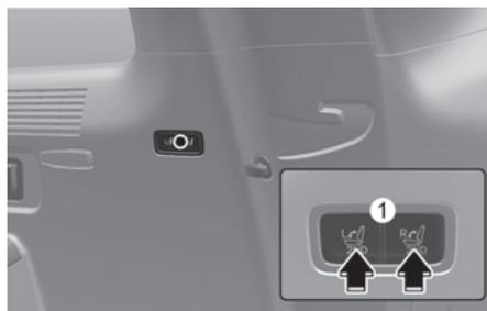
With the liftgate open, this feature allows you to conveniently fold or unfold the 2nd row seatback forward or rearward.
