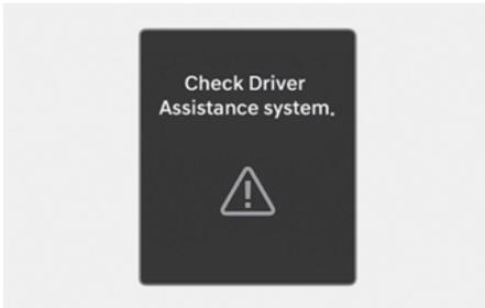
When Driver Attention Warning is not working properly, the "**Check Driver Assistance system.**" warning message will appear on the cluster for several seconds, and the master (⚠) warning light and the driver's attention (🚦) warning light will appear on the instrument cluster. If this occurs, have your vehicle inspected by an authorized HYUNDAI dealer.
