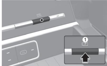
Press the Parking/View button (1) while the gear is in P (Park), D (Drive) or N (Neutral) to turn on the Rear View Monitor.
