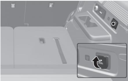
The AC inverter supplies 220 volts/200 watts (or 115 volts/150 watts) electric power to operate electric accessories or equipment.
