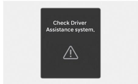
When Reverse Parking Collision-Avoidance Assist or other related functions are not working properly, the "**Check Driver Assistance system.**" warning message appears on the instrument cluster, and Reverse Parking Collision-Avoidance Assist turns off automatically. Have your vehicle inspected by an authorized HYUNDAI dealer.
