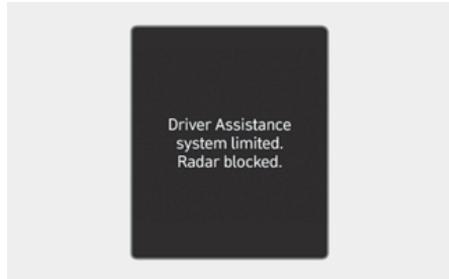
When the rear bumper around the rear corner radar or sensor is covered with foreign material, such as snow or rain, or installing a trailer or carrier, it can reduce the detecting performance and temporarily limit or disable Safe Exit Assist.
