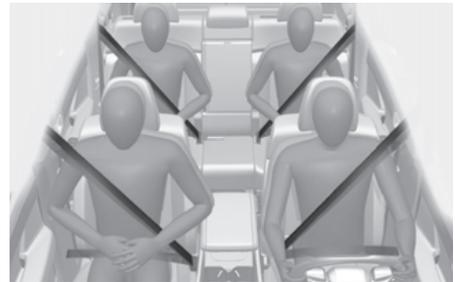
Your vehicle is equipped with driver's and front passenger's and rear passengers pretensioner seat belts (retractor pretensioner). The pretensioner makes sure the seat belts fit tightly against your body in certain frontal or side collision(s). The pretensioner seat belts may be activated in some crashes where the frontal or side collision(s) is severe enough, together with the airbags.
