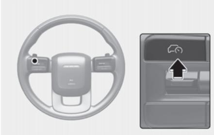
Press the Driving Assist (🚗) button to turn Manual Speed Limit Assist off. The Speed Limit (🚗LIMIT) indicator will go off. Always press the Driving Assist (🚗) button to turn Manual Speed Limit Assist off when not in use.
