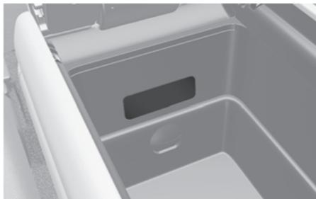
The two-way multi console lamp turns on when you turn on the interior button lights while the Engine Start/Stop button is in the ON position.
