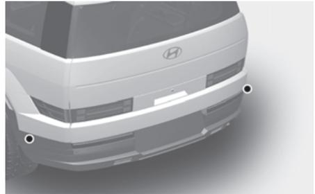
These ultrasonic sensors are mounted near the rear wheels outside your vehicle.
