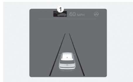
1. Highway Driving Assist indicator, whether there is a vehicle ahead and the selected distance level are displayed.
