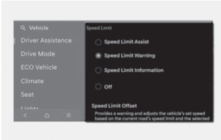
With the engine on, select or deselect **Setup > Vehicle > Driver Assistance > Speed Limit** from the infotainment system to set whether to use each function.
