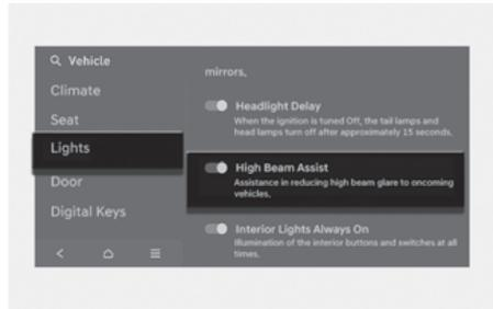
With the Engine Start/Stop button ON, go to the Settings menu to turn on High Beam Assist and deselect to turn off the function in the infotainment system. Select:
