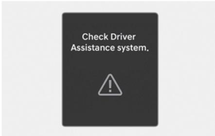
When Safe Exit Assist is not working properly, the "**Check Driver Assistance system.**" warning message appears on the instrument cluster for several seconds, and the master (⚠) warning light illuminates on the instrument cluster. If this occurs, have your vehicle inspected by an authorized HYUNDAI dealer.
