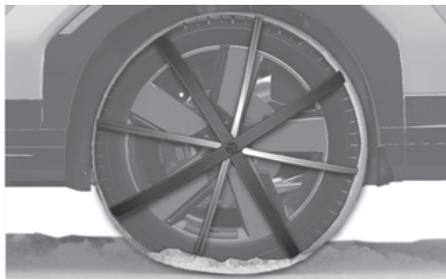
Since the sidewalls of radial tires are thinner than other types of tires, they may be damaged by mounting some types of tire chains on them. Therefore, the use of snow tires is recommended
