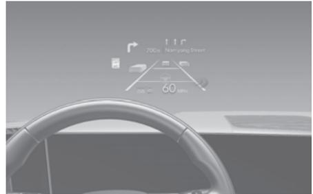
The Head-Up Display is an optional feature that allows the driver to view information projected onto a transparent screen while still keeping your eyes on the road ahead while driving.
