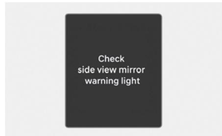
When the side view mirror warning light is not working properly, the "**Check side view mirror warning light**" warning message appears on the instrument cluster for several seconds, and the master (
