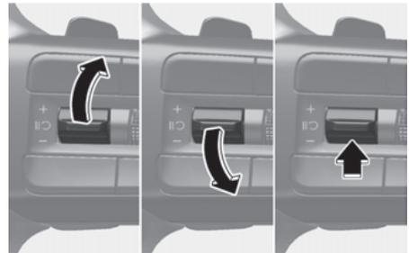
To resume Manual Speed Limit Assist after the function was paused, operate the **+**, **-**, **II** switch.
