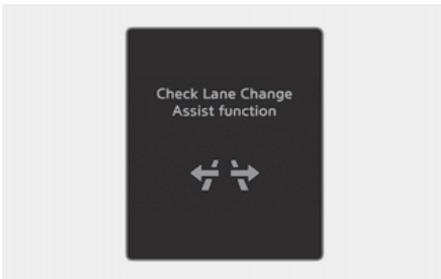
When Highway Driving Assist is not working properly, the "**Check Driver Assistance system.**" or "**Check Lane Change Assist function**" warning message and Master (⚠) warning light appears on the instrument cluster. If this occurs, have your vehicle inspected by an authorized HYUNDAI dealer.
