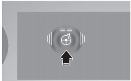
When the Engine Start/Stop button is in the ON position or when the engine is running, press the steering wheel heater button to warm the steering wheel.
