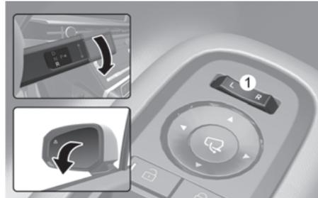
When the gear is shifted to the R (Reverse) position, the side view mirrors rotate downwards to aid with driving in reverse.
