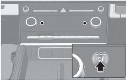
While the engine is running, touch the icon to warm the driver's seat or front passenger's seat.
