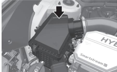
The air cleaner filter can be cleaned for inspection using compressed air. Do not attempt to wash or rinse it, because water can damage the filter. If soiled, replace the air cleaner filter.
