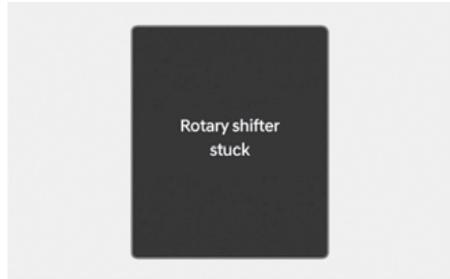
This message appears when the rotary gear shift dial does not return back to its normal position after rotating it. Have your vehicle inspected by an authorized HYUNDAI dealer.
