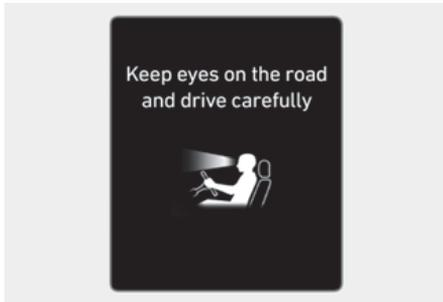
Forward Attention Warning determines whether the driver is focused on the road depending on information, such as the amount of time the driver is looking elsewhere, the amount of time the eyes are closed, how frequently the driver yawns, etc. If Forward Attention Warning judges the driver is not focused, the **"Keep eyes on the road and drive carefully"** warning message will appear on the cluster, and an audible warning will sound.
