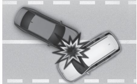
In an angled collision, the force of impact may position the occupants in a direction where the airbags would not be able to provide any additional benefit, and thus the sensors may not deploy any airbags.
