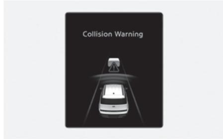
While Smart Cruise Control is operating, when the collision risk with the vehicle ahead is high, the "**Collision Warning**" warning message will appear on the instrument cluster, an audible warning will sound, and the steering wheel will vibrate to warn the driver. Always have your eyes on the road while driving, and if necessary, depress the brake pedal to reduce your driving speed in order to maintain a safe distance.
