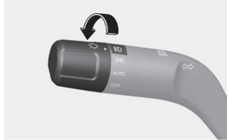
The headlight, parking light, license plate light, and instrument panel light are turned ON.
