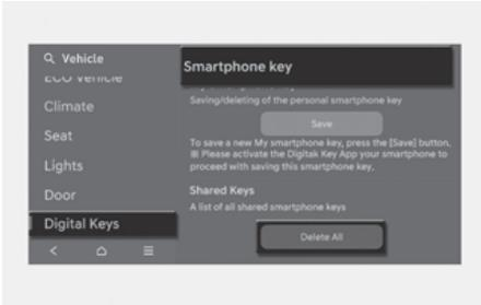
To delete all the registered digital key (smartphone), select **Setup > Vehicle > Digital Keys > Smartphone key > Delete all** from the infotainment system.
