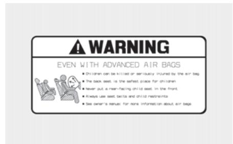
Airbag warning labels, required by the U.S. National Highway Traffic Safety Administration (NHTSA), are attached to alert the driver and passengers of potential risks of the airbag system. Be sure to read all of the information about the airbags that are installed on your vehicle in this Owners Manual.
