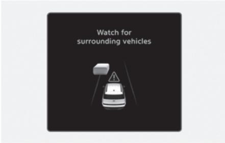
In the following situation, the "**Watch for surrounding vehicles**" warning message will appear on the instrument cluster, and an audible warning will sound to warn the driver of road conditions ahead.
