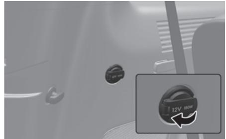
The power outlet is designed to provide power for mobile phones or other devices designed to operate with vehicle electrical systems. The devices should draw less than 12 V, 180 W with the engine running.
