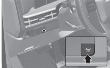
Press the Tow mode button to turn on or off the function.
