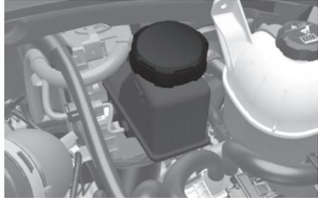
Check the fluid level in the reservoir periodically. The fluid level must be between the MAX and the MIN marks on the side of the reservoir.
