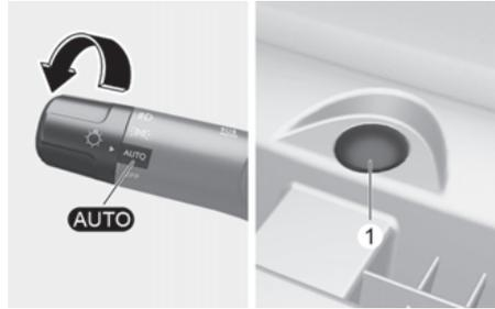
The headlights and parking lights are turned ON or OFF automatically depending on the amount of daylight as measured by the ambient light sensor (1) in front of the instrument panel.
