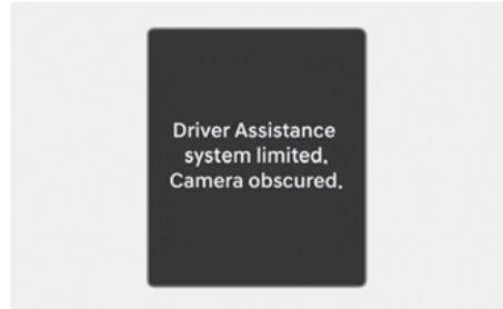
When the front windshield where the front view camera is located is covered with foreign material, such as snow or rain, it can reduce the detecting performance and temporarily limit or disable Driver Attention Warning.
