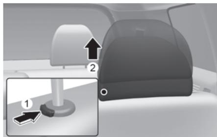
To remove the head restraint:
