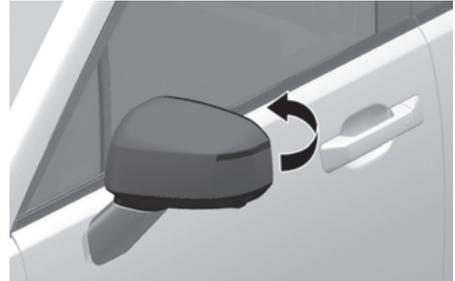
To fold the side view mirror, grasp the housing of the mirror and then fold it toward the rear of the vehicle.
