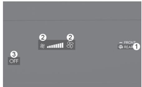
1. Press the 3rd row air conditioning FRONT/REAR button (1) located on the front climate control panel and set the fan speed to the desired speed with the fan speed button (2). (indicator light on the REAR button will illuminate).
