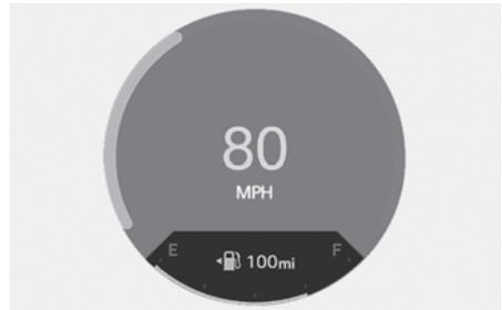
The fuel gauge indicates the approximate amount of fuel remaining in the fuel tank.
