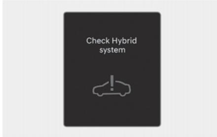
This message appears when there is a problem with the hybrid control system. Refrain from driving when the warning message appears.
