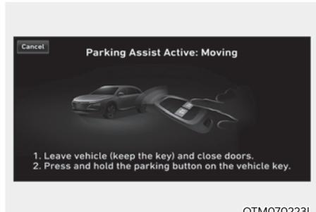
Method (2) Using the function with engine on
