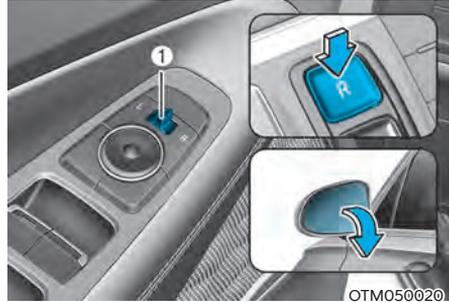
When the gear is shifted to the R (Reverse) position, the side view mirror(s) will rotate downwards to aid with driving in reverse.
