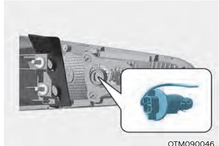
5. Remove the bulb from the socket by pressing it in and rotating it counterclockwise until the tabs on the bulb align with the slots in the socket. Pull the bulb out of the socket.
