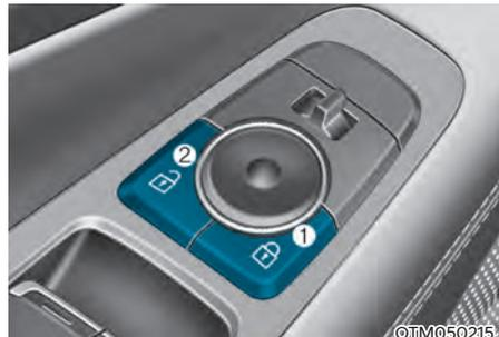
When pressing the (🔒) portion (1) on the switch, all vehicle doors will lock.
