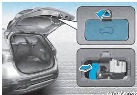
Your vehicle is equipped with the emergency liftgate safety release lever located on the bottom of the liftgate. When someone is inadvertently locked in the luggage compartment. The liftgate can be opened by doing as follows:
