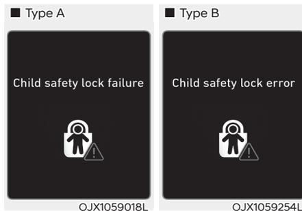
When electronic child safety lock does not work even though the button is pressed, the message will be displayed and an alarm will sound. If this occurs, we recommend that the vehicle be inspected by an authorized HYUNDAI dealer.
