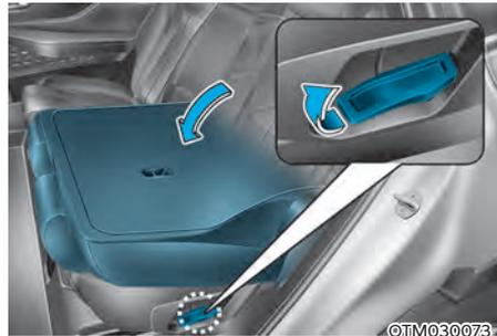
4. Pull on the seatback folding lever (2nd row seat), then fold the seat toward the front of the vehicle. When you return the seatback to its upright position, always be sure it has locked into position by pushing on the top of the seatback.
