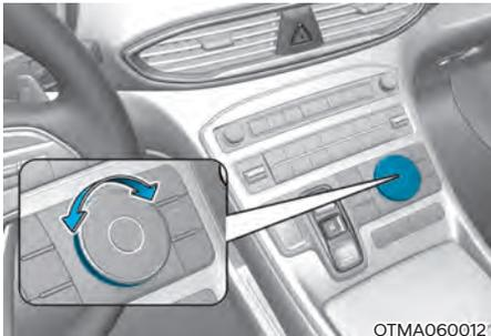
Press the DRIVE/TERRAIN button to change from normal driving mode to multi terrain mode. After the button is pressed, rotate the knob within 4 seconds to select SNOW, MUD or SAND.
