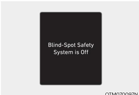
When the engine is restarted with the system off, the 'Blind-spot safety system is Off' message will appear on the cluster.
