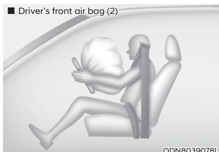
Upon deployment, tear seams molded directly into the pad covers will separate under pressure from the expansion of the air bags. Further opening of the covers allows full inflation of the air bags.
