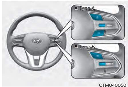
To change the trip mode, toggle the "∧, ∨" switch on the steering wheel
