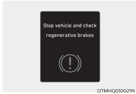
This message is displayed when a failure occurs in the brake system.
