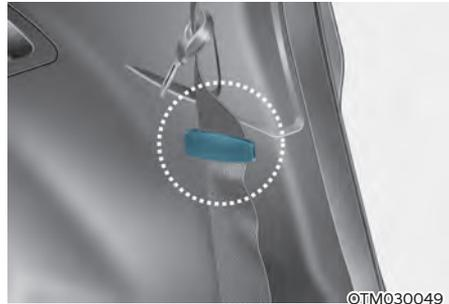
3. Route the seat belt webbing through the rear seat belt guides to prevent the belts from being trapped behind or under the seats.
