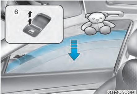
If a window senses any obstacle while it is closing automatically, it will stop and lower approximately 12 in. (30 cm) to allow the object to be cleared.
