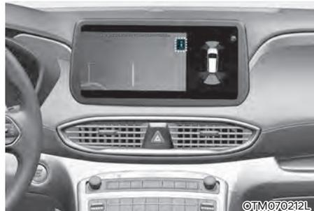
When you touch the **i** icon, the top view is displayed on the screen and shows the distance from the vehicle in the back of your vehicle while parking.
