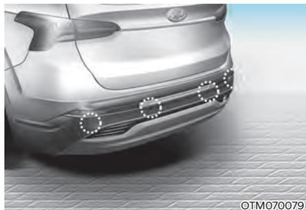
The rear ultrasonic sensors are located inside the rear bumper to detect objects in the rear area. If the sensors are covered with foreign material, such as snow or rain, it may adversely affect sensor performance and Reverse Parking Collision-Avoidance Assist may not operate normally. Always keep the rear bumper clean.
