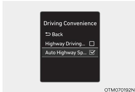
With the engine on, select 'Driver assistance → Driving Convenience → Auto motorway speed control' from the Settings menu to turn on Navigation-based Smart Cruise Control and deselect to turn off the system.
