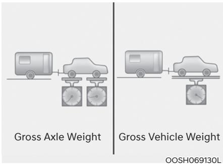
The tongue load is an important weight to measure because it affects the total Gross Vehicle Weight (GVW) of your vehicle. The trailer tongue should weigh a maximum of 10% of the total loaded trailer weight, within the limits of the maximum trailer tongue load permissible.
