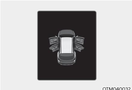
This warning is displayed if any door or the hood or the liftgate is left open. The warning will indicate which door is open in the display.
