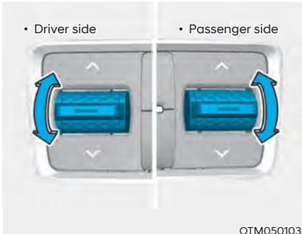
The temperature will increase by pushing the knob upward. The temperature will decrease by pushing the knob downward.
