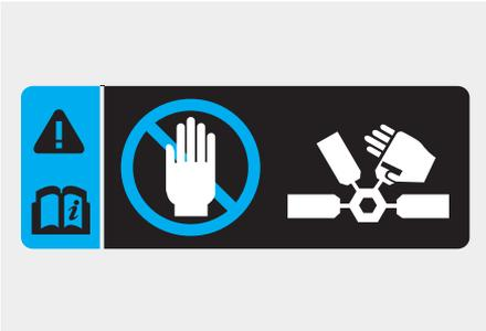
The electric motor for the cooling fan may continue to operate or start up when the engine is not running and can cause serious injury. Keep hands, clothing and tools away from the rotating fan blades of the cooling fan. Always turn off the vehicle unless the vehicle has to be inspected with the engine on. Be cautious as the cooling fan may operate if the negative (-) battery terminal is not disconnected.
