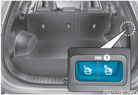
Push the 2nd row seat back folding switch (1) located in the right side in the liftgate. (L : Left seatback folding, R : Right seatback folding)
