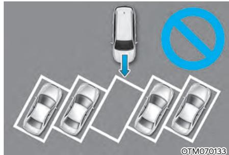
Remote Smart Parking Assist does not provide diagonal parking. Even if your vehicle was able to enter the parking space, do not use the system because the system cannot operate normally.
