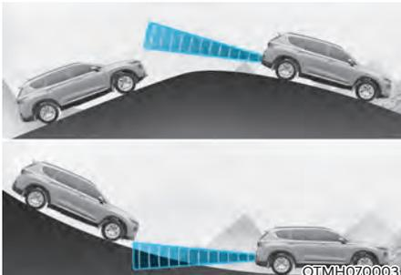
Blind-Spot Safety system may not operate properly when driving on a slope. The system may not detect the vehicle in the next lane or may incorrectly detect the ground or structure.
