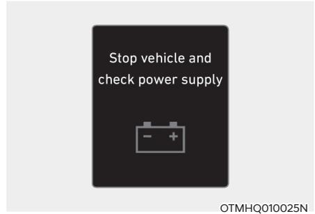
This message is displayed when a failure occurs in the power supply system. If this occurs, park the vehicle in a safe location and tow your vehicle to the nearest authorized HYUNDAI dealer and have the vehicle inspected.
