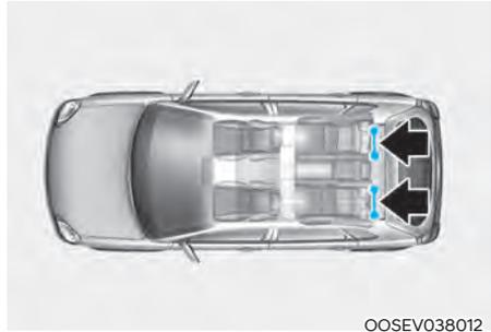
Lower anchors have been provided in the left and right outboard rear seating positions. Their locations are shown in the illustration. There are not lower anchors provided for the center rear seating position.
