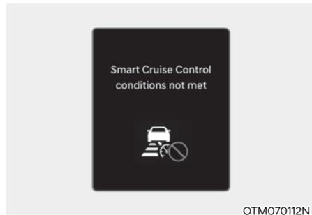
If the Driving Assist button, + switch, - switch or
