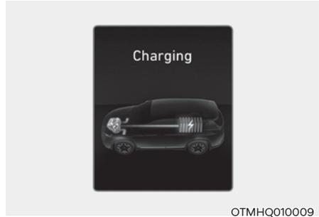
The engine is simultaneously used to drive the vehicle and to charge up the high-voltage battery.
