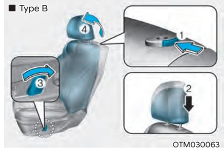
To reinstall the head restraint :
