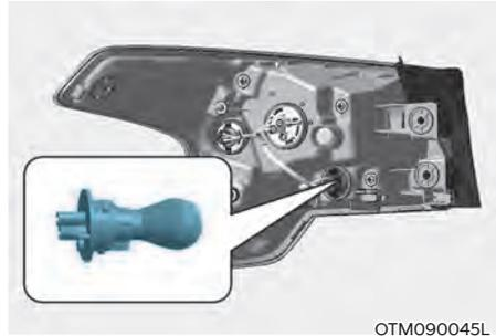
6. Remove the bulb from the socket by pressing it in and rotating it counterclockwise until the tabs on the bulb align with the slots in the socket. Pull the bulb out of the socket.
