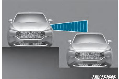
Blind-Spot Safety system may not operate properly when driving where the heights of the lanes are different. The system may not detect the vehicle on a road with different lane heights (underpass joining section, grade separated intersections, etc.).
