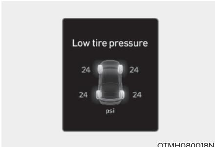
When the tire pressure monitoring system warning indicators are illuminated and a warning message displayed on the cluster LCD display, one or more of your tires is significantly under-inflated. The Low Tire Pressure Position Telltale will indicate which tire is significantly underinflated by illuminating the corresponding position light.
