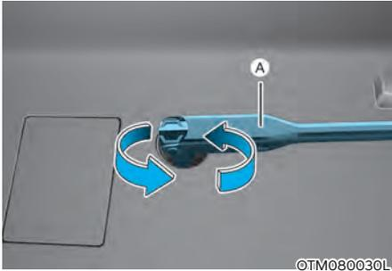
3. Connect the wheel lug nut wrench (A) to the bolt.
