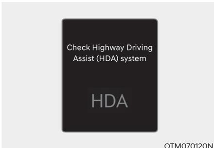
When Highway Driving Assist or Highway Lane Change function is not working properly, the 'Check HDA (Motorway Driving Assist) system' warning message will appear, and the
