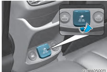
The AC inverter supplies 115V/110W electric power to operate electric accessories or equipments.
