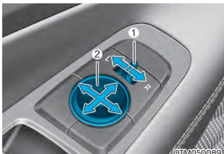
1. Move the lever (1) either to the L (left side) or R (right side) to select the side view mirror you would like to adjust.
