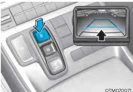
Rear View Monitor will show the area behind the vehicle to assist you when parking or backing up.
