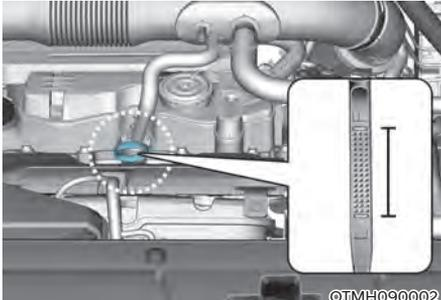
6. Pull the dipstick out again and check the level. The level should be between F (Full) and L (Low).
