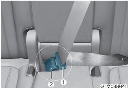
1. Insert the tongue plate (1) into the buckle (2) until an audible “click” is heard, indicating the latch is locked. Make sure the belt is not twisted.
