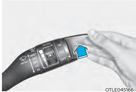
Push the lever away from you to spray rear washer fluid and to run the rear wipers 1-3 cycles. The spray and wiper operation will continue until you release the lever.
