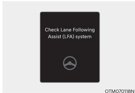
When Lane Following Assist is not working properly, the 'Check LFA (Lane Following Assist) system' warning message will appear on the cluster. If this occurs, we recommend that the system be inspected by an authorized HYUNDAI dealer.
