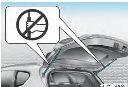
Do not hold the part (gas lifter) that supports the liftgate. Be aware that the deformation of the part may cause vehicle damage and a risk of injury.
