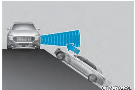
Rear Cross-Traffic Safety system may be limited when the vehicle is on a uphill or downhill slope, or near it, and may not detect the vehicle approaching from the left or right. If this occurs, the system may not warn the driver or control the brakes when necessary.
