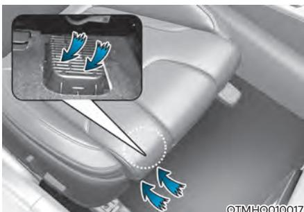
The hybrid battery cooling duct is located under the Passenger's seat. The cooling duct cools down the hybrid battery. When the hybrid battery cooling duct is blocked, the hybrid battery may be overheated.
