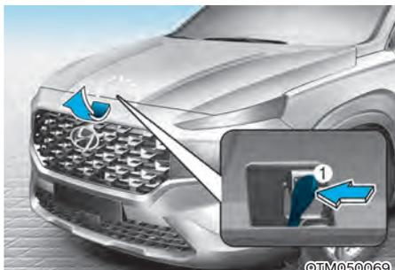
3. Go to the front of the vehicle, raise the hood slightly, push up the secondary latch (1) inside of the hood center and lift the hood.
