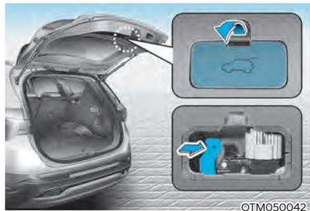
Your vehicle is equipped with the emergency liftgate safety release lever located on the bottom of the liftgate inside the vehicle.
