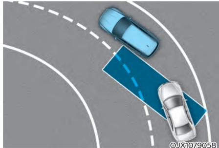
**Blind-Spot Safety system may not operate properly when driving on a curved road. The system may recognize a vehicle in the same lane. Always pay attention to road and driving conditions while driving.**
