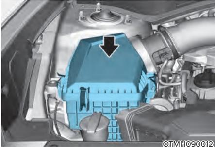
Do not attempt to wash or to rinse it, as water will damage the filter. If soiled, the air cleaner filter must be replaced.
