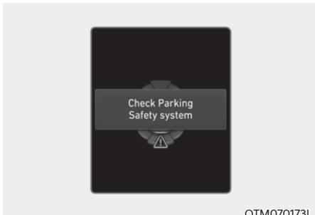
When Reverse Parking Collision-Avoidance Assist or other related systems are not working properly, the 'Check Parking Safety system' warning message will appear on the cluster, and the system will turn off automatically. We recommend that the system be inspected by an authorized HYUNDAI dealer.
