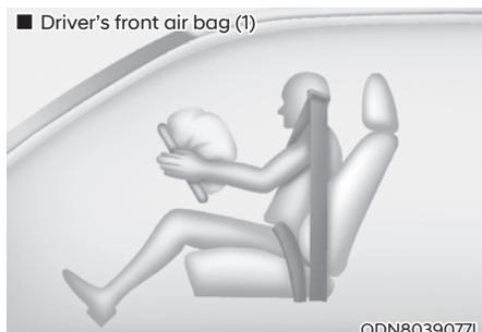
When the SRSCM detects a sufficiently severe impact to the front of the vehicle, it will automatically deploy the front air bags.
