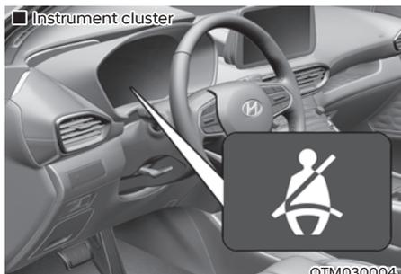
As a reminder to the driver, the seat belt warning light will illuminate for approximately 6 seconds each time you place the ignition switch to the ON position regardless of belt fastening. At this time, if the seat belt is not fastened a warning chime will sound for 6 seconds.
