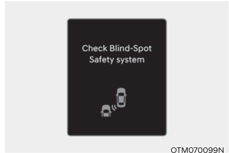
When Safe Exit Assist is not working properly, the 'Check blind-spot safety systems' warning message will appear on the cluster, and the system will turn off automatically or the system will be limited. We recommend that the system be inspected by an authorized HYUNDAI dealer.
