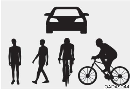
The illustration above shows the image the front view camera will detect as a vehicle, pedestrian and cyclist.
