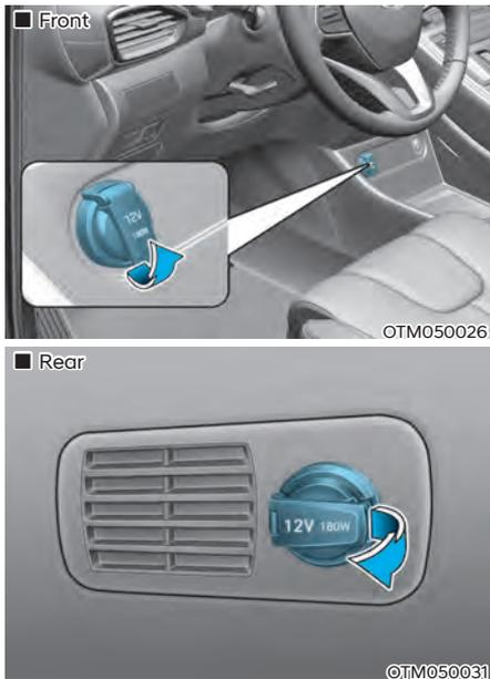
The power outlet is designed to provide power for mobile telephones or other devices designed to operate with vehicle electrical systems. The devices should draw less than 180 watts with the engine running.
