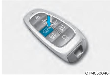
The power liftgate will open automatically by doing one of the following:
