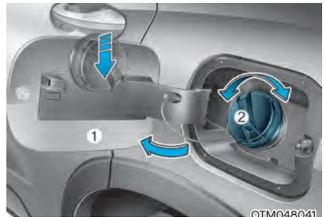
4. Pull the fuel filler door (1) outward to access the fuel tank cap.
