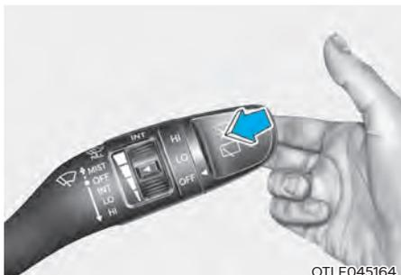
In the OFF (O) position, pull the lever gently toward you to spray washer fluid on the windshield and to run the wipers 1-3 cycles. The spray and wiper operation will continue until you release the lever. If the washer does not work, you may need to add washer fluid to the washer fluid reservoir.
