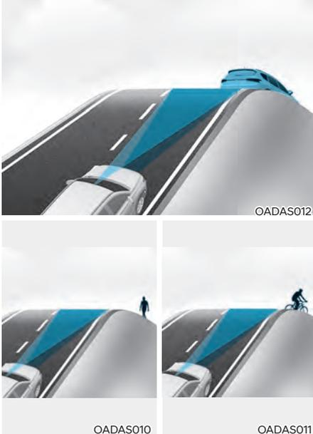
**Forward Collision-Avoidance Assist may not detect the vehicle, pedestrian or cyclist in front of you while driving uphill or downhill adversely affecting the performance of the sensors.**
