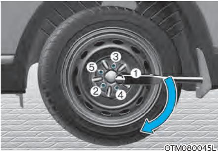
12. Use the wheel lug nut wrench to tighten the lug nuts in the order shown. Double-check each lug nut until they are tight. After changing tires, we recommend that an authorized HYUNDAI dealer tighten the lug nuts to their proper torque as soon as possible. **The wheel lug nut should be tightened to 79~94 lbf.ft (11~13 kgf.m).**
