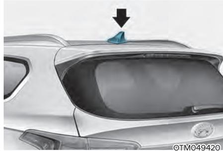
The shark fin antenna receives transmitted data. (for example: AM/FM, DAB, GPS)
