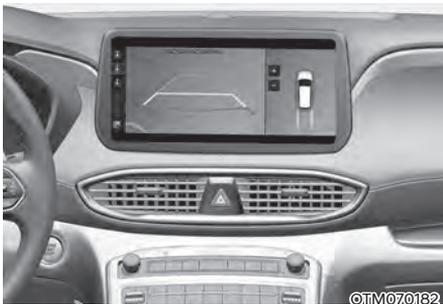
Surround View Monitor will assist in parking using the cameras installed on the vehicle and displays images around the vehicle through the infotainment system screen.
