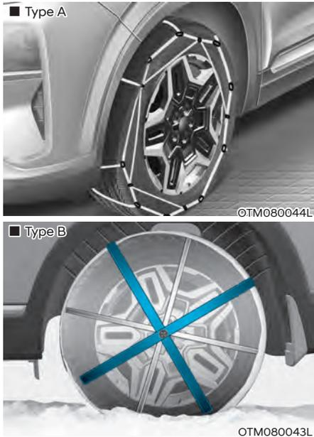
Since the sidewalls of radial tires are thinner than other types of tires, they may be damaged by mounting some types of tire chains on them. Therefore, the use of snow tires is recommended instead of tire chains. If tire chains must be used, use genuine HYUNDAI parts if available and install the tire chain after reviewing the instructions provided with the tire chains. Damage to your vehicle caused by improper tire chain use is not covered by your vehicle manufacturer's warranty.
