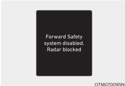
When the front windshield where the front view camera is located, front radar Cover, or sensor is covered with foreign material, such as snow or rain, it can reduce the detecting performance and temporarily limit or disable Forward Collision-Avoidance Assist.
