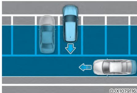
Rear Cross-Traffic Safety system may detect vehicles passing by behind you when parking in reverse into a parking space. If this occurs, the system may unnecessarily warn the driver and control the brake.
