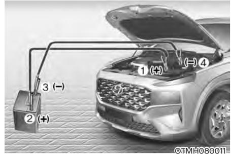
5. Connect the jumper cables in the exact sequence shown in the illustration. First connect one jumper cable to the red, positive (+) jumper terminal of your vehicle (1).
