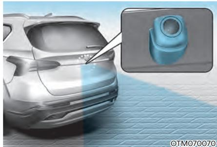
The rear view camera is used as a detecting sensor to help detect pedestrians. If the camera lens is covered with foreign material, such as snow or rain, it may adversely affect camera performance and Reverse Parking Collision-Avoidance Assist may not operate normally. Always keep the camera lens clean.
