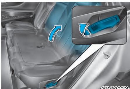
5. To use the rear seat, lift and pull the seatback backward by pulling the folding lever or the strap. Pull the seatback firmly until it clicks into place. Make sure the seatback is locked in place.
