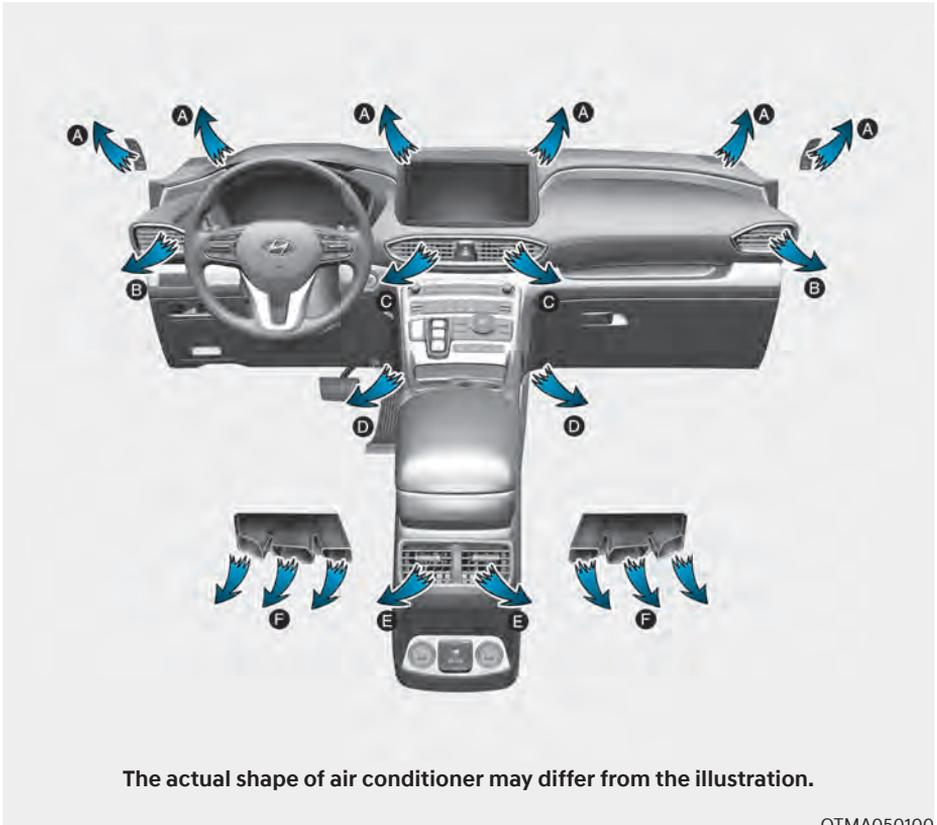
The mode selection button controls the direction of the air flow through the ventilation system.
