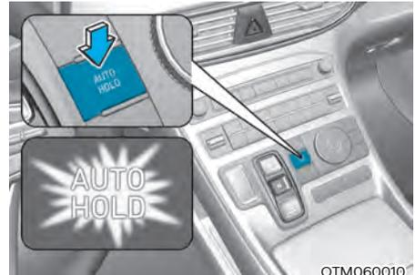
1. With the driver's door, engine hood and liftgate closed, then press the [AUTO HOLD] switch. The white AUTO HOLD indicator will come on and the system will be in the standby position.
