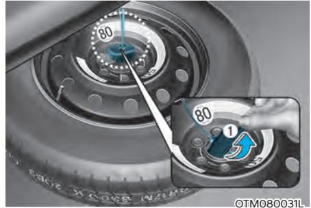
6. Draw out the retainer guide (1) the through the center hole of spare tire.
