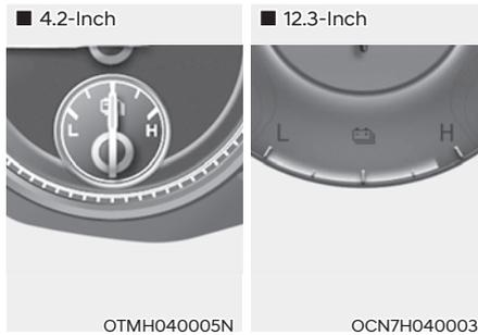
This gauge indicates the remaining hybrid battery power. If the SOC is near the “O or L (Low)” level, the vehicle automatically operates the engine to charge the battery.
