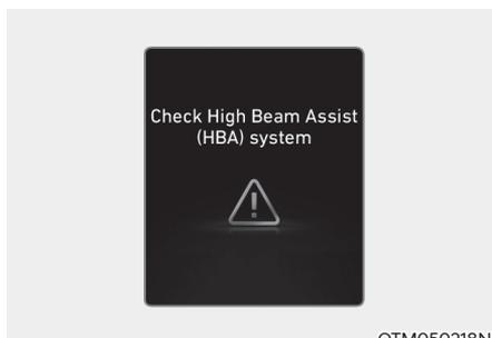
When High Beam Assist is not working properly, the 'Check High Beam Assist (HBA) system' or 'Check HBA (High Beam Assist system)' warning message will appear and
