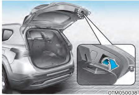
Lower the liftgate lid and press down until it locks. To be sure the liftgate lid is securely fastened, always check by trying to pull it up again without pressing the liftgate handle button.
