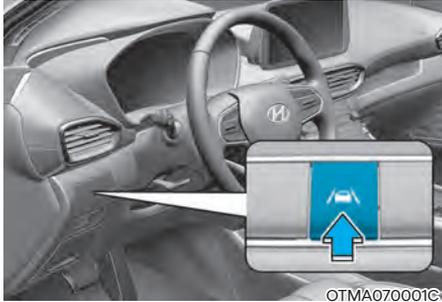
With the engine on, press and hold the Lane Safety button located on the instrument panel to turn on Lane Keeping Assist. The white
