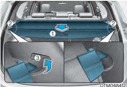
1. Pull the cargo security screen towards the rear of the vehicle by the handle (1).
