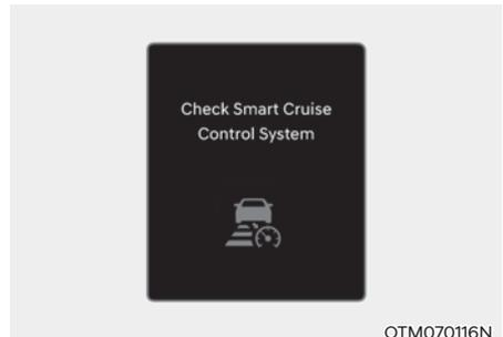
When Smart Cruise Control is not working properly, the 'Check SCC (Smart Cruise Control) system' warning message will appear, and the
