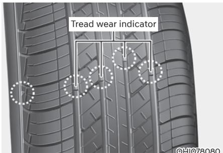
If the tire is worn evenly, a tread wear indicator will appear as a solid band across the tread. This shows there is less than 1/16 in. (1.6 mm) of tread left on the tire. Replace the tire when this happens.
