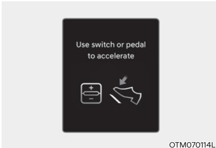
In traffic, your vehicle will stop if the vehicle ahead of you stops. Also, if the vehicle ahead of you starts moving, your vehicle will start as well. In addition, after the vehicle has stopped and a certain time have passed, the 'Use switch or pedal to accelerate' message will appear on the cluster. Depress the accelerator pedal or push the + switch, - switch or II switch to start driving.
