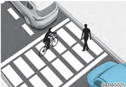
If there is a pedestrian(s) or bicycle(s) in between you and the vehicle in front, Leading Vehicle Departure Alert may not operate properly.
