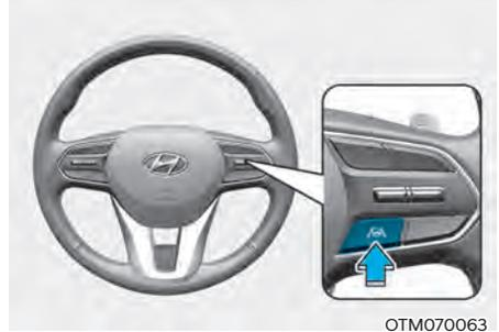
With the engine on, press and hold the Lane Driving Assist button located on the steering wheel to turn on Lane Keeping Assist. The white
