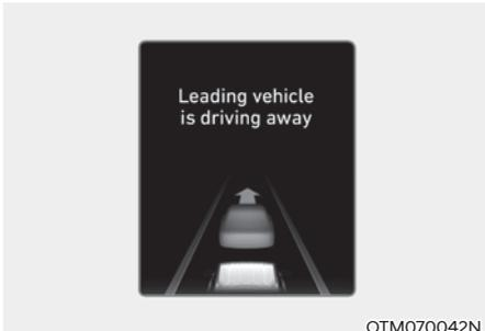
When a detected vehicle in front departs from a stop, Leading Vehicle Departure Alert will inform the driver by displaying the 'Leading vehicle is driving on' message on the cluster and an audible warning will sound.
