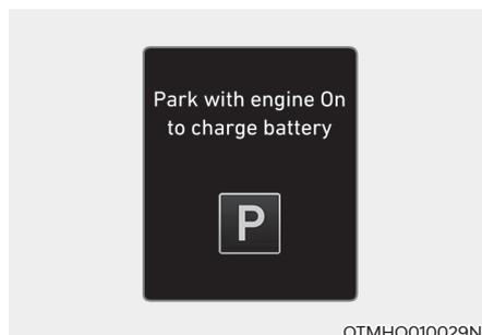
This message is displayed when the hybrid battery power (SOC) level is low. If this occurs, park the vehicle in a safe location and wait until the hybrid battery is charged.
