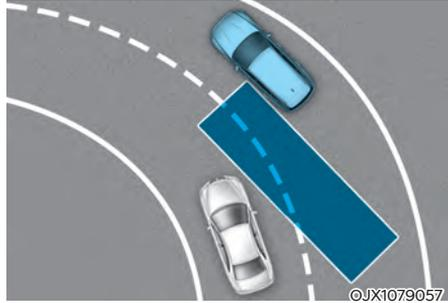
**Blind-Spot Safety system may not operate properly when driving on a curved road. The system may not detect the vehicle in the next lane. Always pay attention to road and driving conditions while driving.**
