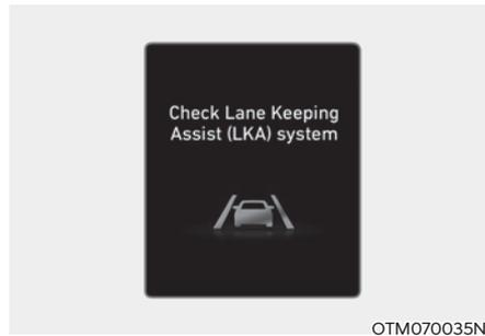
When Lane Keeping Assist is not working properly, the 'Check LKA (Lane Keeping Assist) system' warning message will appear and the yellow
