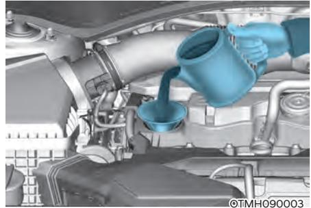
7. Check if the oil level is between the F-L line and refill it if the oil level is near the L line.
