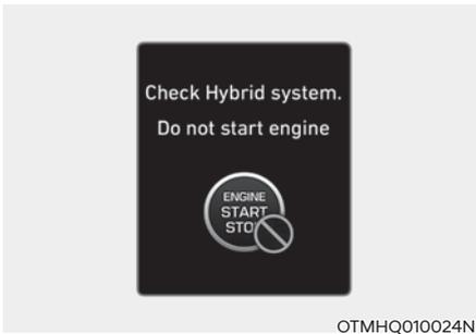
This message is displayed when the hybrid battery power (SOC) level is low. A warning chime will sound until the problem is solved. Refrain from driving when the warning message is displayed. If this occurs, we recommend that you have the vehicle inspected by an authorized HYUNDAI dealer.
