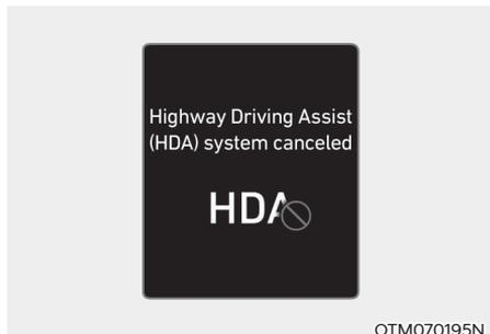
If the driver still does not have their hands on the steering wheel after the hands-off warning, the 'HDA (Motorway Driving Assist) cancelled' warning message will appear and Highway Driving Assist and Lane Change Assist will be automatically canceled.
