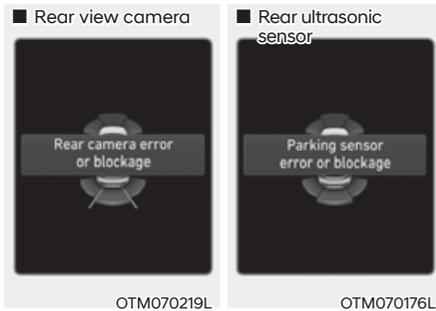
The 'Rear camera error or blockage' or 'Parking sensor error or blockage' warning message will appear on the cluster if the following situations occur:
