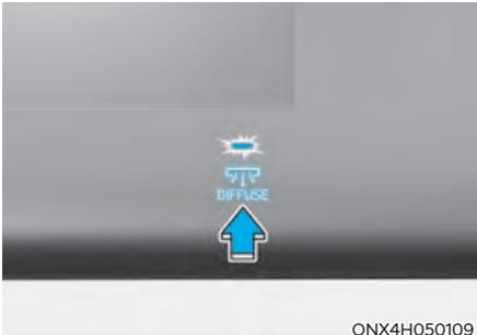
When the Multi-Air mode button is pressed, air flow is directed to the face level and floor level and through perforated sections along the instrument panel for the driver and passenger. The multi-air mode LED indicator will be illuminated.
