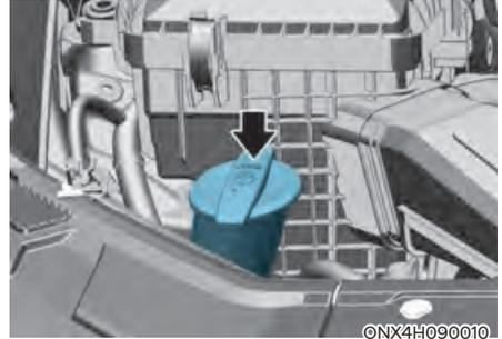
Check the fluid level in the washer fluid reservoir and add fluid if necessary. Plain water may be used during summer months if washer fluid is not available. However, use washer solvent with antifreeze characteristics in cold climates to prevent freezing.
