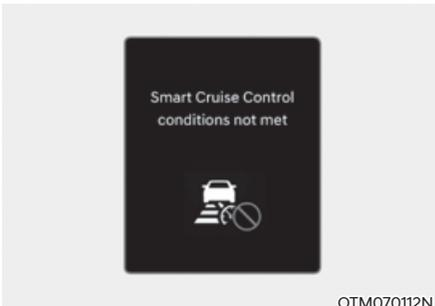
If the Driving Assist button, + switch, - switch or
