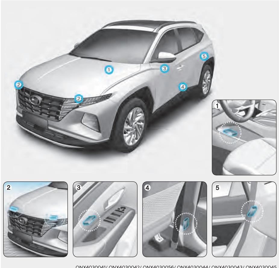
1. SRS control module / Rollover sensor
