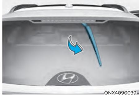
1. Within 20 seconds after the vehicle ignition is OFF, pull down the wiper lever to MIST position for over 2 seconds until the wiper moves down to the bottom middle part.
