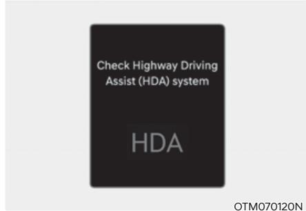
When Highway Driving Assist is not working properly, the 'Check HDA (Motorway Driving Assist) system' warning message will appear, and the
