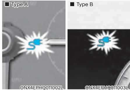
9. Check if the charging indicator light of the high voltage battery on the instrument cluster is turned ON. Charging is not done when the charging indicator lamp is OFF.
