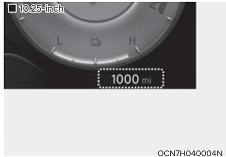
The odometer indicates the total distance that the vehicle has been driven and should be used to determine when periodic maintenance is required.
