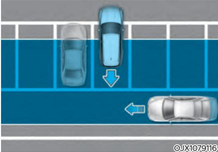
Rear Cross-Traffic Collision-Avoidance Assist may detect vehicles passing by behind you when parking in reverse into a parking space. If this occurs, the function may unnecessarily warn the driver and control the brake.
