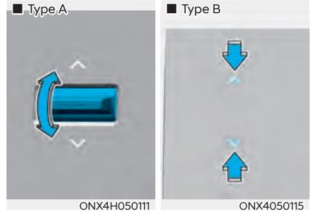
The temperature setting will increase when you toggle up or touch the UP arrow on the touchscreen (if equipped). The temperature setting will decrease when you toggle down or touch the DOWN arrow on the touchscreen (if equipped).
