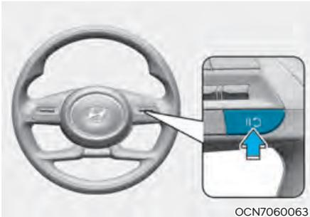
Push the **||** switch to temporarily pause the set speed limit. The set speed limit will turn off but the Manual Speed Limit Assist enabled (**LIMIT**) indicator will stay on.
