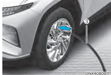
2. Connect the connection hose (3) of the compressor and tire into the tire valve.
