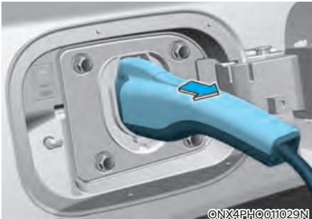
2. Hold the charging connector handle and pull it while pressing the release button (1).
