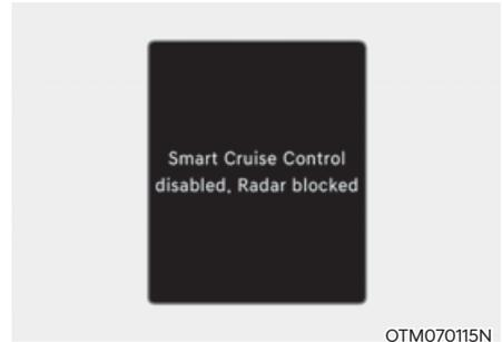
When the front radar cover or sensor is covered with snow, rain, or foreign material, it can reduce the detecting performance and temporarily limit or disable Smart Cruise Control.
