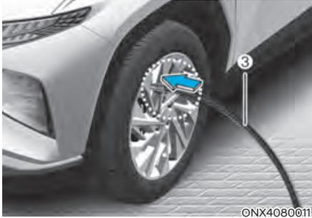
14. Connect the connection hose (3) of the compressor and tire into the tire valve.
