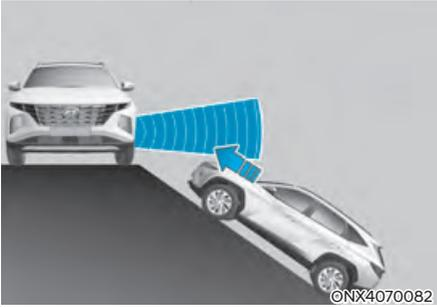
**Rear Cross-Traffic Collision-Avoidance Assist** may be limited when the vehicle is on an uphill or downhill slope, or near it, and may not detect the vehicle approaching from the left or right. If this occurs, the function may not warn the driver or control the brakes when necessary.
