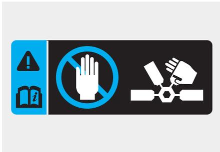
The electric motor for the cooling fan may continue to operate or start up when the engine is not running and can cause serious injury. Keep hands, clothing and tools away from the rotating fan blades of the cooling fan. Always turn off the vehicle unless the vehicle has to be inspected with the engine on. Be cautious as the cooling fan may operate if the negative (-) battery terminal is not disconnected.
