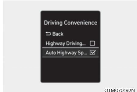
With the engine on, select 'Driver Assistance → Driving Convenience → Auto motorway speed control' from the Settings menu to turn on Navigation-based Smart Cruise Control and deselect to turn off the function.
