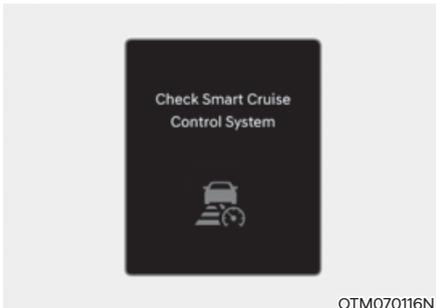
When Smart Cruise Control is not working properly, the 'Check Smart Cruise Control system' warning message will appear, and the
