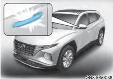
The welcome system will illuminate the vehicle door handles when the driver approaches with the smart key.
