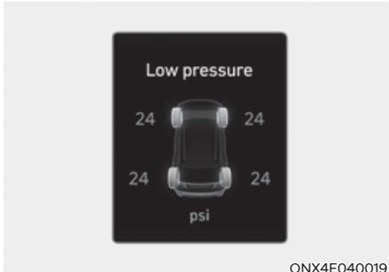
When the tire pressure monitoring system warning indicators are illuminated and a warning message displayed on the cluster LCD display, one or more of your tires is significantly under-inflated. The Low Tire Pressure Position Telltale will indicate which tire is significantly underinflated by illuminating the corresponding position light.
