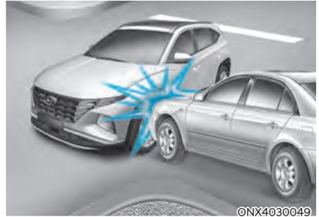
Front air bags may not inflate in side impact collisions, because occupants move in the direction of the collision, and thus in side impacts, front air bag deployment would not provide additional occupant protection.
