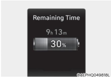
8. After charging has started, the estimated charging time is displayed on the instrument cluster for about 1 minute.
