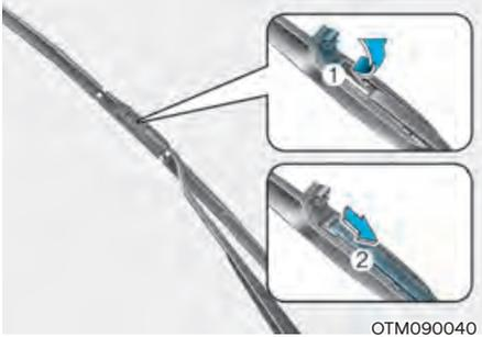
2. Lift up the wiper blade clip. Then pull down the blade assembly and remove it.
