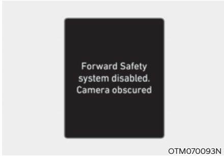
When the front windshield where the front view camera is located or the sensor is covered with foreign material, such as snow or rain, it can reduce the detecting performance and temporarily limit or disable Forward Collision-Avoidance Assist.
