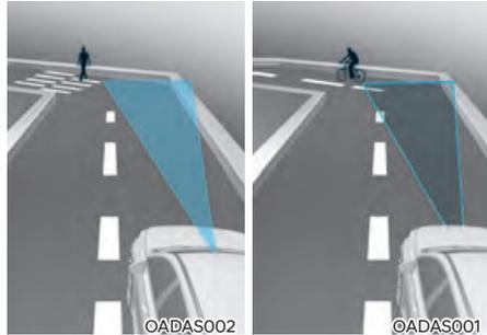
**Forward Collision-Avoidance Assist may not detect other vehicles or pedestrians in front of you on curved roads adversely affecting the performance of the sensors. This may result in no warning or braking assist when necessary.**
