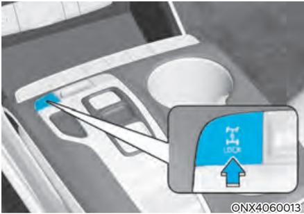
All Wheel Drive (AWD) delivers engine power to front and rear wheels for maximum traction. AWD is useful when extra traction is required, such as when driving on, muddy, wet, or snow-covered roads.
