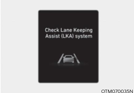
When Lane Keeping Assist is not working properly, the 'Check Lane Keeping Assist (LKA) system' warning message will appear and the yellow
