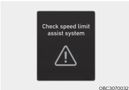
When Intelligent Speed Limit Assist is not working properly, the ‘Check Speed Limit Assist System’ warning message will appear on the cluster for several seconds, and the master (⚠) warning light will illuminate on the cluster. If this occurs, have the vehicle inspected by an authorized HYUNDAI dealer.
