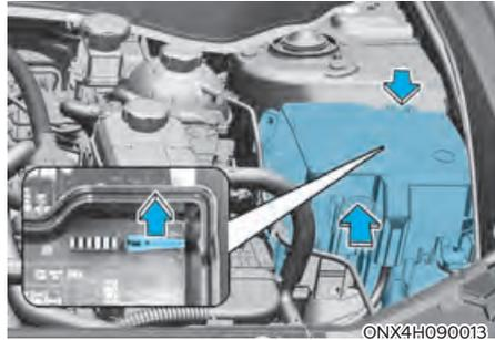
5. Pull the suspected fuse straight out. Use the removal tool provided in the engine compartment fuses panel cover.
