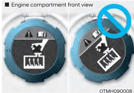
1. Check if the coolant cap label is straight in front.
