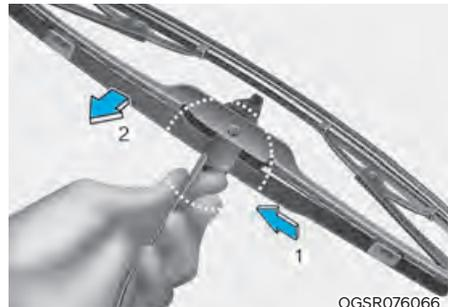
1. Lift up the wiper blade clip. Then lift up the wiper blade.
