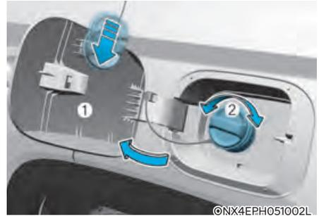
4. Pull the fuel filler door (1) out to fully open.
