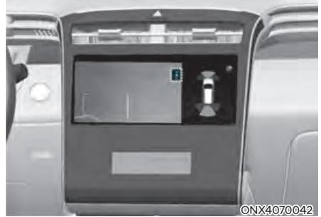
When you touch the
