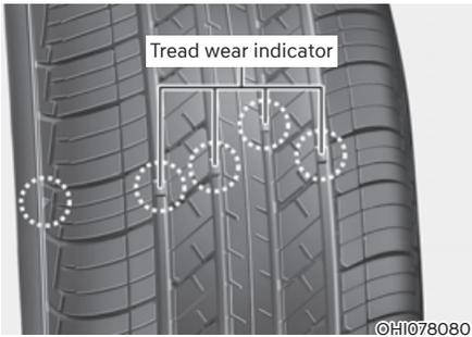
If the tire is worn evenly, a tread wear indicator will appear as a solid band across the tread. This shows there is less than 1/16 in. (1.6 mm) of tread left on the tire. Replace the tire when this happens.
