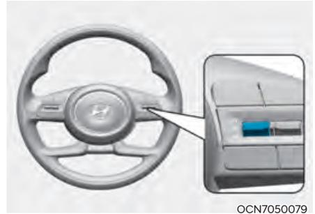
To change the trip mode, toggle the " $\wedge$ ,  $\vee$ " switch on the steering wheel
