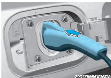
7. Hold the charging connector handle and connect it to the vehicle AC charging inlet. Push the connector until you hear a “clicking” sound. If the charging connector and charging terminal are not connected properly, this may cause a fire.
