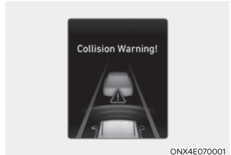
While Smart Cruise Control is operating, when the collision risk with the vehicle ahead is high, the 'Collision Warning' warning message will appear on the cluster, and an audible warning will sound to warn the driver. Always have your eyes on the road while driving, and if necessary, depress the brake pedal to reduce your driving speed in order to maintain a safe distance.
