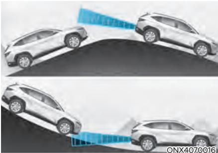
Blind-Spot Collision-Avoidance Assist may not operate properly when driving on a sloped road. The function may not detect the vehicle in the next lane or may incorrectly detect the ground or structure. Always pay attention to road and driving conditions while driving.
