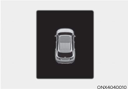
If the driver turns off the engine when the sunroof is not fully closed, the warning chime will sound for several seconds and the sunroof open warning will appear on the cluster LCD display. Close the sunroof securely when leaving your vehicle.
