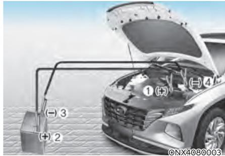
3. Connect the jumper cables in the exact sequence shown in the illustration. First connect one jumper cable to the red, positive (+) jumper terminal of your vehicle (1).
