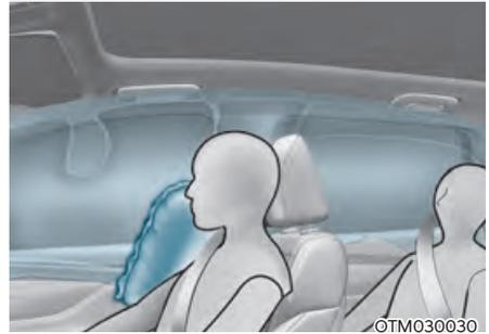
Your vehicle is equipped with a side air bag in each front seat. The purpose of the air bag is to provide the vehicle's driver and the front passenger with additional protection than that offered by the seat belt alone.
