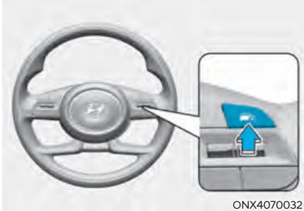
Press the Driving Assist (
