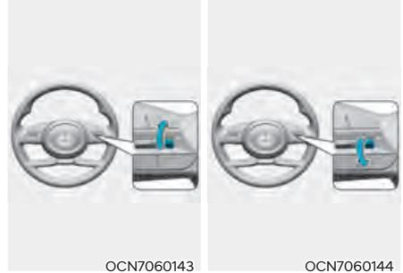
To resume Manual Speed Limit Assist after the function was paused, push the +, -, **||** switch.
