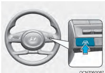
With the engine on, press and hold the Lane Driving Assist button located on the steering wheel to turn on Lane Keeping Assist. The white
