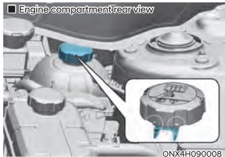
2. Make sure that the tiny protrusions inside the coolant cap is securely interlocked.
