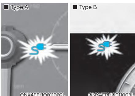
7. Check if the charging indicator light of the high voltage battery on the instrument cluster is turned ON. Charging is not done when the charging indicator lamp is OFF.
