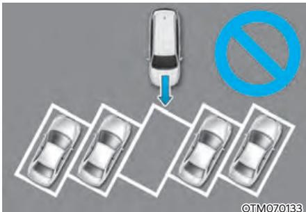
Remote Smart Parking Assist does not provide diagonal parking. Even if your vehicle was able to enter the parking space, do not use Remote Smart Parking Assist because the function cannot operate normally.
