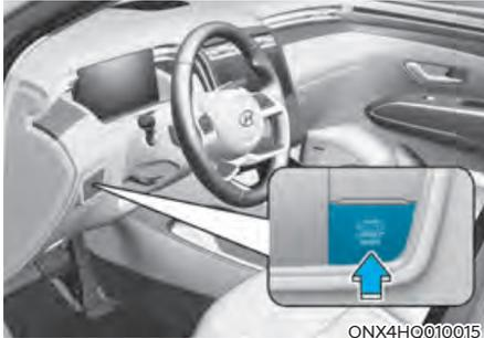
1. Press the 12V Battery Reset switch to reconnect the 12V battery.
