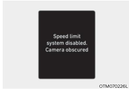
When the front windshield where the front view camera is located is covered with foreign material, such as snow or rain, it can reduce the detecting performance and temporarily limit or disable Intelligent Speed Limit Assist. If this occurs, the ‘Speed Limit Assist system disabled. Camera obscured’ warning message will appear on the cluster.
