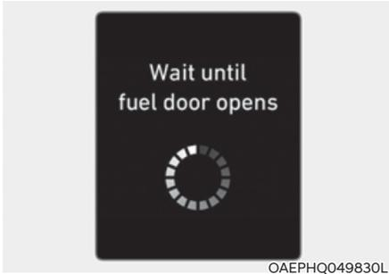
3. Wait until the fuel tank is depressurized. This message may appear in the LCD cluster display while the fuel system is depressurizing. The fuel door will open after a few seconds.
