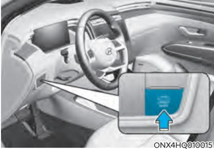
7. Press the 12V Battery Reset switch.
