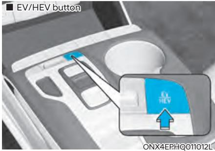
Pressing the [EV/HEV] button changes the plug-in hybrid system modes, between Electric (CD) mode and Hybrid (CS) mode.
