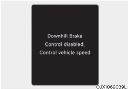
**Downhill Brake Control disabled. Control vehicle speed (manually)**
