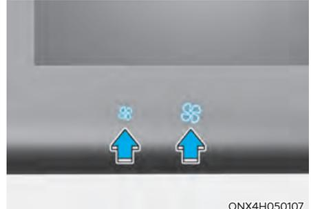
The fan speed can be set as desired by pushing the fan speed control button. Increased air flow is delivered with higher fan speeds. Pressing the OFF button turns off the fan.
