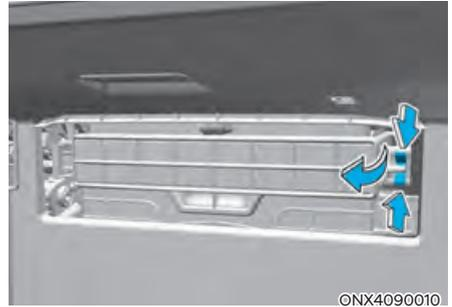
3. Remove the climate control air filter case while pressing the lock on the right side of the cover.
