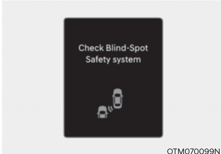
When Blind-Spot Collision-Avoidance Assist is not working properly, the 'Check Blind-Spot Safety system' warning message will appear on the cluster, and the function will turn off automatically or the function will be limited. Have the vehicle inspected by an authorized HYUNDAI dealer.
