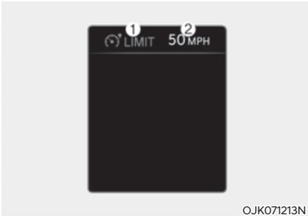
(1) Manual Speed Limit Assist enabled indicator
