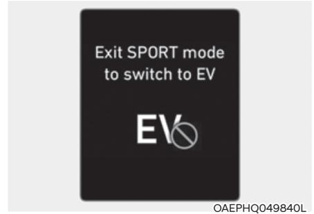
This message is displayed when [HEV] button is pressed but it is impossible to switch from the HEV mode to EV mode because the SPORT mode is engaged.
