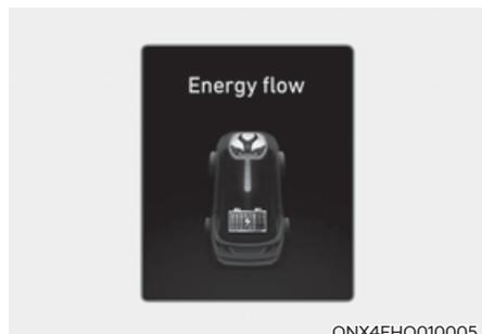
When the vehicle is stopped, the high-voltage battery is charged up by the engine.
