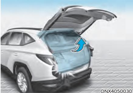
During automatic opening and closing if the power liftgate is blocked by an object or part of the body, the power liftgate will detect the resistance.
