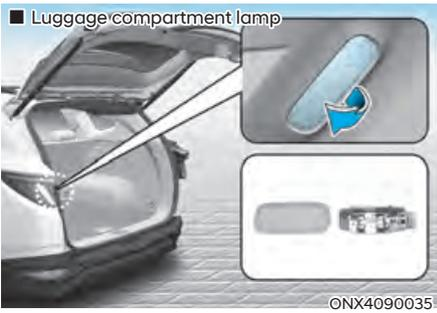
1. Using a flat-head screwdriver, gently pry the lens from the interior light housing.
