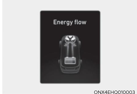
Both the motor and the engine power are used to drive the vehicle.
