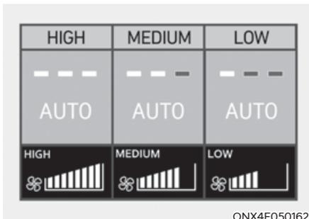
You can control the fan speed in three stages by pushing the AUTO button during automatic operation.
