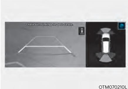
You can change Rear View Monitor 'Display Contents' by touching the setup icon (1) on the screen while Rear View Monitor is operating, or selecting 'Driver Assistance → Parking Safety → Camera settings' from the Settings menu while the engine is on.
