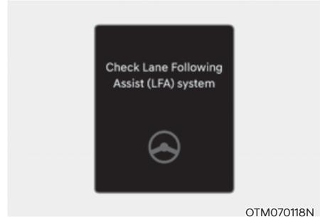
When Lane Following Assist is not working properly, the 'Check Lane Following Assist (LFA) system' warning message will appear on the cluster. If this occurs, have the vehicle inspected by an authorized HYUNDAI dealer.
