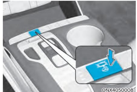
When the ignition switch is in the ON position or when the engine is running, press the heated steering wheel button to warm the steering wheel.
