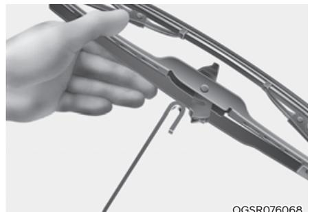
3. Remove the wiper blade from the wiper arm.
