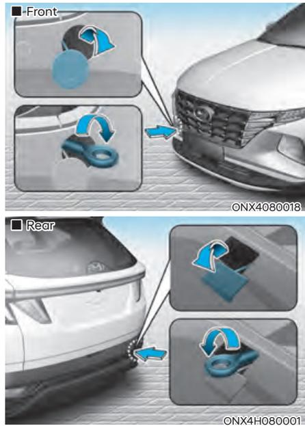
2. Remove the hole cover by pressing the lower part of the cover on the bumper.
