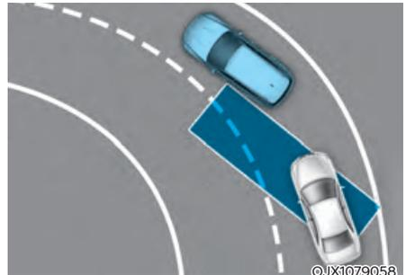
**Blind-Spot Collision-Avoidance Assist may not operate properly when driving on a curved road. The function may not recognize a vehicle in the same lane.**
