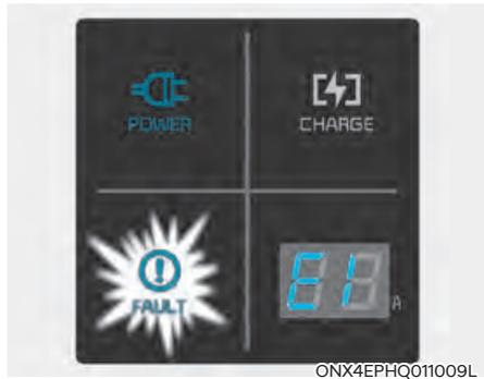
Before plugging charging connector into vehicle (Power indicator : green ON, Fault indicator : red blink)
