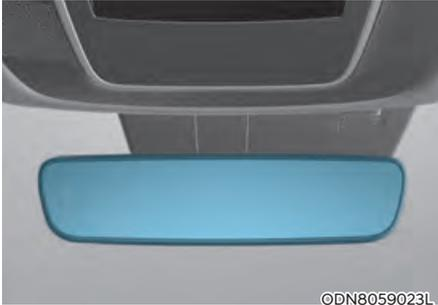
The electrochromic rearview mirror automatically controls the glare from the headlamp of the vehicle behind you in nighttime or low light driving conditions. When the engine is running, the glare is automatically controlled by the sensor mounted in the rearview mirror. The sensor detects the light level around the vehicle, and automatically adjusts to control the headlamp glare from vehicles behind you.
