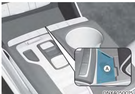
[A] : Wireless Charging Pad (In-vehicle Authentication Pad)
