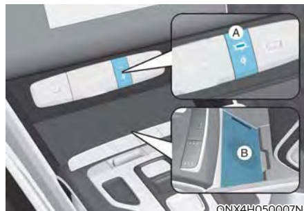
[A] : Indicator light, [B] : Charging pad
