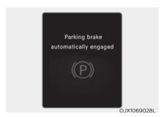
Parking brake automatically engaged If EPB is applied while Auto Hold is activated, a warning will sound and a message will appear.
