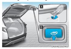
If the battery has been discharged or disconnected, or if the power liftgate fuse has been replaced or removed, reset the power liftgate by performing the following procedure:
