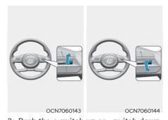
2. Push the + switch up or - switch down, and release it at the desired speed. Push the + switch up or - switch down and hold it. The speed will increase or decrease to the nearest multiple of five (multiple of ten in km/h) at first.
