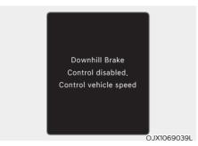
Downhill Brake Control disabled. Control vehicle speed (manually)
