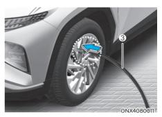
5. Unscrew the valve cap from the valve of the defective and screw the connection hose (3) of the compressor and tire.
