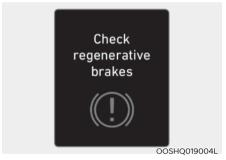
This message is displayed when the brake performance is low or the regenerative brake does not work properly due to a failure in the brake system.
