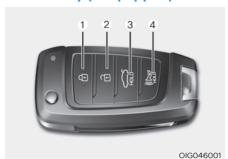
Your HYUNDAI uses a remote key, which you can use to lock or unlock the driver and passenger doors or the liftgate.
