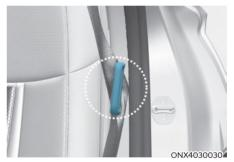
Routing the seat belt webbing through the rear seat belt guides will help keep the belts from being trapped behind or under the seats.
