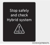
This message is displayed when there is a problem with the hybrid control system. The "\(\frac{1}{2}\)" indicator will blink and a warning chime will sound for approximately 10 seconds until the problem is solved. Refrain from driving when the warning message is displayed.
