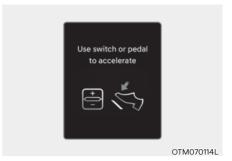
In traffic, your vehicle will stop if the vehicle ahead of you stops. Also, if the vehicle ahead of you starts moving, your vehicle will start as well. In addition, after the vehicle has stopped and a certain time have passed, the 'Use switch or pedal to accelerate' message will appear on the cluster. Depress the accelerator pedal or push the + switch, - switch or IID switch to start driving.
