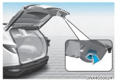
Lower the liftgate lid and press down until it locks. To be sure the liftgate lid is securely fastened, always check by trying to pull it up again without pressing the liftgate handle button.
