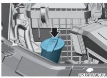
Check the fluid level in the washer fluid reservoir and add fluid if necessary. Plain water may be used during summer months if washer fluid is not available. However, use washer solvent with antifreeze characteristics in cold climates to prevent freezing.
