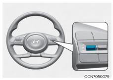
To change the trip mode, toggle the "\,, \rightarrow" switch on the steering wheel
