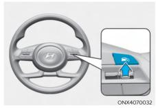
Press the Driving Assist button to turn Cruise Control off. The Cruise (GCRUISE) indicator will go off.
