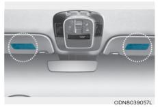
Air bag warning labels, required by the U.S. National Highway Traffic Safety Administration (NHTSA), are attached to alert the driver and passengers of potential risks of the air bag system.
