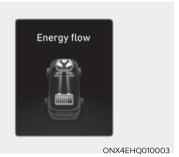
Both the motor and the engine power are used to drive the vehicle.
