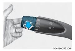
To flash the high beam headlamp, pull the lever towards you, then release the lever. The high beams will remain ON as long as you hold the lever towards you.
