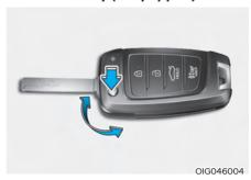
If the remote key does not operate normally, you can lock or unlock the door by using the mechanical key.
