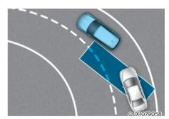
Blind-Spot Safety system may not operate properly when driving on a curved road. The function may recognize a vehicle in the same lane.
