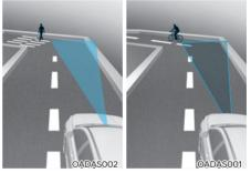
Forward Collision-Avoidance Assist may not detect other vehicles or pedestrians in front of you on curved roads adversely affecting the performance of the sensors. This may result in no warning or braking assist when necessary.
