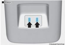
The USB charger is designed to recharge batteries of small size electrical devices using a USB cable.
