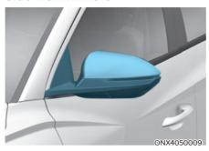
Your vehicle is equipped with both lefthand and right-hand Side view mirrors. The mirrors can be adjusted remotely with the mirror adjustment control switch. The side view mirrors can be folded manually to help prevent damage when going through an automatic car wash or when passing through a narrow street.
