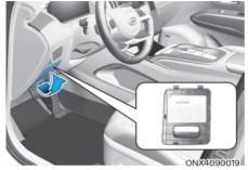
Inside the fuse/relay box cover, you can find the fuse/relay label describing fuse/relay names and ratings.
