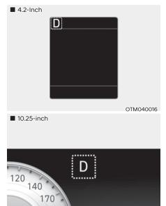
The Transmission Shift Indicator is shown in the upper corner of the LCD display to indicate the current gear or Park(P).
