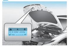
Your HYUNDAI vehicle is filled with R-1234-yf refrigerant. Information regarding the refrigerant designation for your vehicle can be found on the information label located under the hood. Refer to chapter 8 for the location of the air conditioning refrigerant label.
