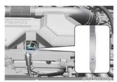
Pull the dipstick out again and check the level. The level should be between F (Full) and L (Low).
