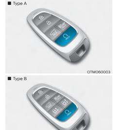
You can start the vehicle using the Remote Start button of the smart key.
