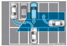
Rear Cross-Traffic Safety system may detect vehicles which are parking or pulling out near your vehicle (for example: a vehicle leaving beside your vehicle, a vehicle parking or pulling out in the rear area, a vehicle approaching your vehicle making a turn, etc.). If this occurs, the function may unnecessarily warn the driver and control the brake.
