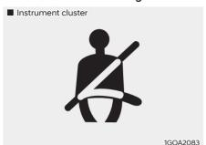
As a reminder to the driver, the seat belt warning light will illuminate for approximately 6 seconds each time the ignition is ON position regardless of belt fastening. At this time, if the seat belt is not fastened a warning chime will sound for 6 seconds.
