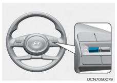
To change the trip mode, toggle the "\,, \righty" switch on the steering wheel
