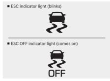
If the ignition switch is placed in the LOCK/OFF position when ESC is off, ESC remains off. Upon restarting the vehicle, ESC will automatically turn on again.
