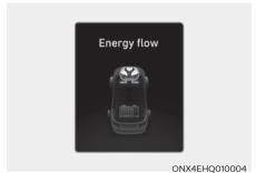
Only the engine power is used to drive
