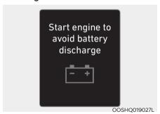
This message is displayed to inform the driver the 12V battery may be discharged if the ignition switch is in ON position (without the  $\rightleftharpoons$  indicator ON).
