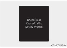
When Rear Cross-Traffic Safety system is not working properly, the 'Check rear cross-traffic safety systems' warning message will appear on the cluster, and the function will turn off automatically or the function will be limited. Have the vehicle inspected by an authorized HYUNDAI dealer.
