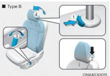
To reinstall the head restraint:
