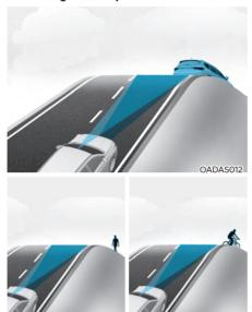
Forward Collision-Avoidance Assist may not detect the vehicle, pedestrian or cyclist in front of you while driving uphill or downhill adversely affecting the performance of the sensors.
