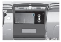
When you touch the icon, the top view is displayed on the screen and shows the distance from the vehicle in the back of your vehicle while parking.
