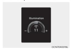
You can adjust the brightness of the instrument panel illumination from the User Settings Mode on the LCD display when the ignition switch is on ('Lights → Illumination'). When the vehicle's parking lights or headlamps are on, interior switch illumination intensity and mood lamps are also adjusted.
