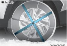
Since the sidewalls of radial tires are thinner than other types of tires, they may be damaged by mounting some types of tire chains on them. Therefore, the use of snow tires is recommended instead of tire chains. If tire chains must be used, use genuine HYUNDAI parts if available and install the tire chain after reviewing the instructions provided with the tire chains. Damage to your vehicle caused by improper tire chain use is not covered by your vehicle manufacturer's warranty.
