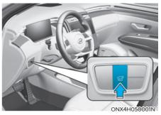
Press the power liftgate button for approximately one second.
