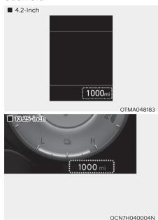
The odometer indicates the total distance that the vehicle has been driven and should be used to determine when periodic maintenance is required.
