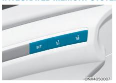
The IMS, or Integrated Memory System, for the driver's seat is equipped on some models. This feature allows the driver to store and recall the following position settings with a simple button operation:
