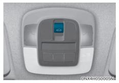
The ignition switch must be in the ON position before you can open or close the sunroof.
