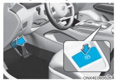
To release EPB (Electronic Parking Brake):
