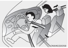
Your vehicle is equipped with driver's and front passenger's Pre-tensioner Seat Belts(Retractor Pretensioner and Emergency Fastening Device System). The purpose of the pre-tensioner is to make sure the seat belts fit tightly against the occupant's body in certain frontal or side collision(s). The Emergency Fastening Device System may be activated in certain crashes where the frontal collision(s) is severe enough, together with the air bags.
