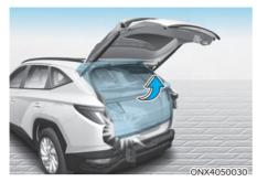
During power opening and closing if the power liftgate is blocked by an object or part of the body, the power liftgate will detect the resistance.
