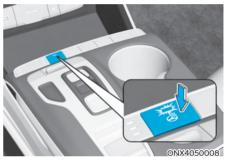
When the ignition switch is in the ON position or when the engine is running, press the heated steering wheel button to warm the steering wheel.
