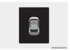
If the driver turns off the engine when the sunroof is not fully closed, the warning chime will sound for a few seconds and the sunroof open warning will appear on the LCD display.
