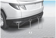
[1]: Rear view camera,[2]: Rear ultrasonic sensors
