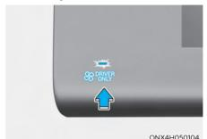
If you press the DRIVER ONLY button and the indicator light illuminates, air mostly blows in the direction of the driver's seat.
