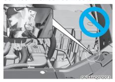
In case of emergency, cut the service interlock connector cable to isolate the high voltage of the battery.
