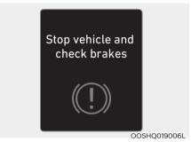
This message is displayed when a failure occurs in the brake system.
