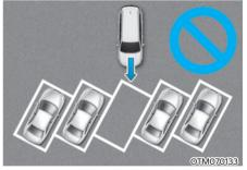
Remote Smart Parking Assist does not provide diagonal parking. Even if your vehicle was able to enter the parking space, do not use Remote Smart Parking Assist because the function cannot operate normally.
