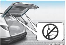
Do not grab or hold on to the liftgate support struts at any time. Damage to the liftgate support struts could result. Deformation of the liftgate support struts may cause vehicle damage and personal injury may occur.
