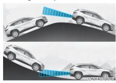
Blind-Spot Safety system may not operate properly when driving on a slope. The function may not detect the vehicle in the next lane or may incorrectly detect the ground or structure.
