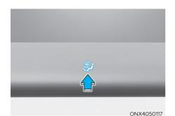
The mode selection button controls the direction of the air flow through the ventilation system.
