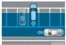
Rear Cross-Traffic Safety system may detect vehicles passing by behind you when parking in reverse into a parking space. If this occurs, the function may unnecessarily warn the driver and control the brake.
