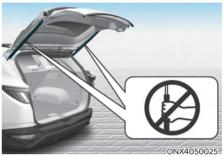
Do not grab or hold on to the liftgate support struts at any time. Damage to the liftgate support struts could result. Deformation of the liftgate support struts may cause vehicle damage and personal injury may occur.
