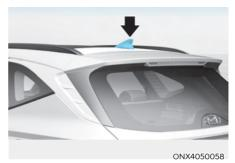
The shark fin antenna receives transmitted data. (for example: AM/FM, DAB, GPS)
