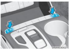
The air ventilation seats are provided to cool the front seats by blowing air through small vent holes on the surface of the seat cushions and seatbacks.
