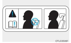
When sitting on the rear seat, do not adjust the height of the head restraint to the lowest position.
