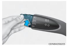
To turn on the high beam headlamp, push the lever away from you. The lever will return to its original position.
