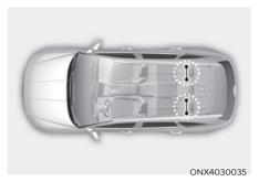
Lower anchors have been provided in the left and right outboard rear seating positions. Their locations are shown in the illustration. There are not lower anchors provided for the center rear seating position.
