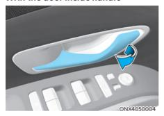
**Driver door & Passenger door**If the inner door handle is pulled when the door is locked, the door will unlock and open.
