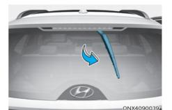
Within 20 seconds after the vehicle ignition is OFF, pull down the wiper lever to MIST position for over 2 seconds until the wiper moves down to the bottom middle part.
