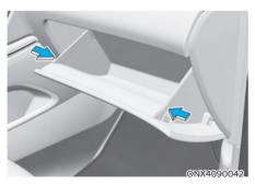
2. Push in both sides of the glove box as shown. This will ensure that the glove box stopper pins will get released from its holding location allowing the glove box to hang.
