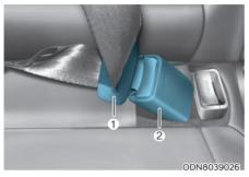
Insert the tongue plate (1) into the buckle (2) until an audible "click" is heard, indicating the latch is locked. Make sure the belt is not twisted.
