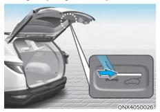
Your vehicle is equipped with the emergency liftgate safety release lever located on the bottom of the liftgate.
