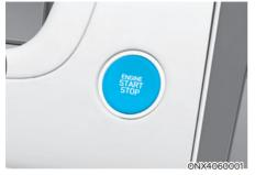
Whenever the front door is opened, the Engine Start/Stop button will illuminate and will go off 30 seconds after the door is closed (if equipped).
