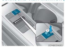
Surround View Monitor system can assist in parking by allowing the driver to see around the vehicle.
