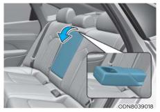
The armrest is located in the center of the rear seat. Pull the armrest down from the seathack to use it
