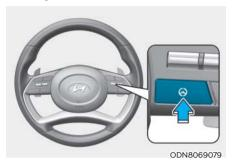
With the Engine Start/Stop button is in the ON or START position, Lane Following Assist can be activated by pressing the button.
