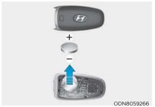
If the Smart Key is not working properly, try replacing the battery with a new one.
