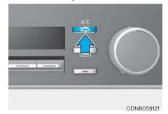
Push the A/C button to manually turn the air conditioning system on (indicator light will illuminate).
