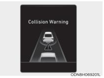
This warning message appears on the LCD display with a warning chime. Additionally, some vehicle system intervention occurs by the engine management system to help decelerate the vehicle.
