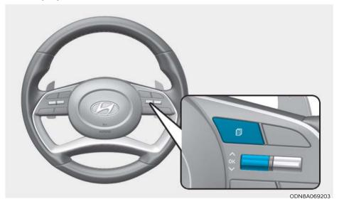
The LCD display modes can be changed by using the control buttons.
