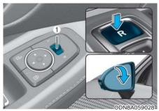
When you press the R (Reverse) button, the side view mirror(s) will rotate downwards to aid with driving in reverse. The position of the side view mirror switch (1) determines whether or not the mirrors will move:
