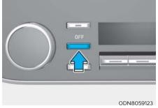
Push the OFF button of the front to turn off the air climate control system. However, you can still operate the mode and air intake buttons as long as the ignition switch is in the ON position.
