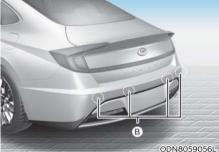
[A]: Front sensor, [B]: Rear sensor
