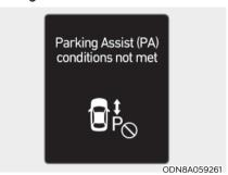
When Remote Smart Parking Assist system is not getting ready for activation, the above message will appear when Remote Smart Parking Assist system button is pressed.
