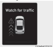
Collision warning when exiting vehicle
