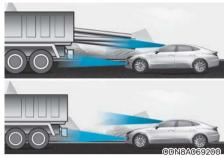
• Detecting the vehicle in front of you If the vehicle in front of you has cargo that extends rearward from the cab, or when the vehicle in front of you has higher ground clearance, additional special attention is required. FCA system may not be able to detect the cargo extending from the vehicle. In these instances, you must maintain a safe braking distance from the rearmost object, and if necessary, depress the brake pedal to reduce your driving speed in order to maintain distance.
