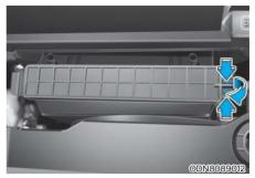
Remove the climate control air filter case while pressing the lock on the right side of the cover.
