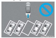
Remote Smart Parking Assist system is not a supplemental for diagonal parking. Even if the vehicle is able to enter the space, do not operate the system.
