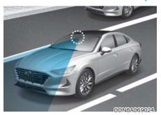
Lane Following Assist system helps detect lane markers on the road with a front view camera at the front windshield, and assists the driver's steering to help keep the vehicle between lanes.
