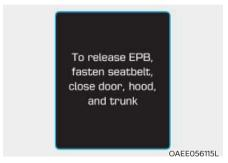
To release EPB, fasten seatbelt, close door, hood and trunk
