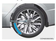
Loosen the wheel lug nuts counterclockwise one turn each in the order shown above, but do not remove any lug nuts until the tire has been raised off of the ground.
