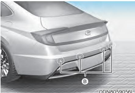
[A] : Front sensor, [B] : Rear sensor
