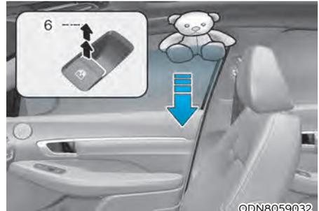
If a window senses any obstacle while it is closing automatically, it will stop and lower approximately 12 inches (30 cm) to allow the object to be cleared.
