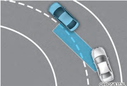
Blind-Spot Collision Avoidance Assist may not operate properly when driving on a curved road. In certain instances, Blind-Spot Collision Avoidance Assist may recognize a vehicle in the same lane.
