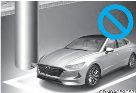
If you want to park your vehicle in the blind spot or near a circular pillar and narrow pillar or a pillar surrounded by objects such as fire extinguisher and the parking distance warning chime sounds three times continuously, the vehicle should not be parked in the area.
