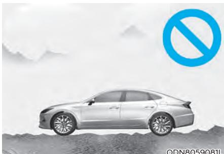
Remote Smart Parking Assist may cancel when the vehicle slips or the vehicle could not move due to road condition such as pebbles or fragmented stones.
