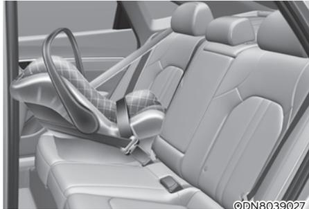
A rear-facing child seat provides restraint with the seating surface against the back of the child. The harness system holds the child in place, and in an accident, acts to keep the child positioned in the seat and reduce the stress to the neck and spinal cord.
