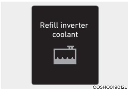
This message is displayed when the inverter coolant is nearly empty. You should refill the inverter coolant.
