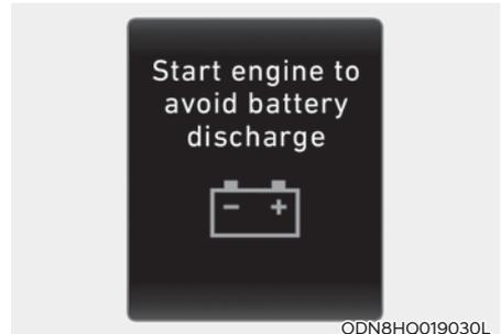
If the engine is not turned on with the Engine Start/Stop button in ACC or ON for a while, the battery can be discharged. Please turn on the engine to prevent 12V battery from discharge.
