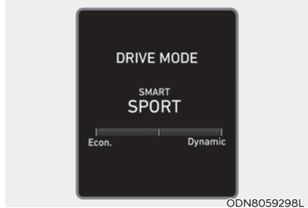
With the standard driving style in the center, the left side of the gauge is 'Econ.' and right side is 'Dynamic' style.
