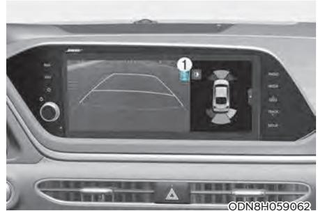
When you touch the icon (1), the top view is displayed on the screen and shows the distance from the vehicle in the back of your vehicle. Touch the icon (1) again, to switch back to the previous screen.
