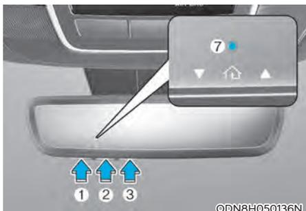
1. Press and release the HomeLink button (1), (2) or (3), you would like to program. The HomeLink indicator light (7) will flash orange slowly (if not, perform the steps of “Erasing HomeLink Buttons” section, and start over).
