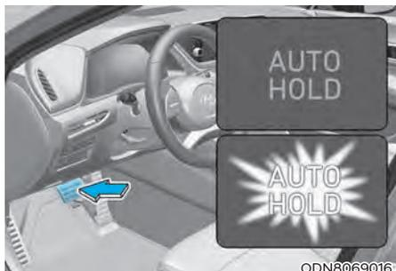
2. When you stop the vehicle completely by depressing the brake pedal, the Auto Hold maintains the brake pressure to hold the vehicle stationary. The indicator changes from white to green.
