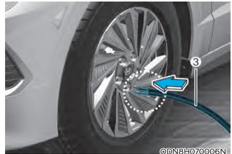
4. Remove the valve cap from the air valve of the damaged tire and connect filling hose (3) of the sealant bottle onto the valve.
