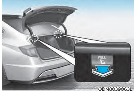
3. Pull on the seatback folding lever located in the trunk.
