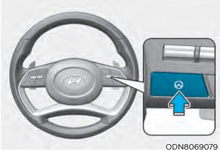
With the Engine Start/Stop button is in the ON or START position, Lane Following Assist can be activated by pressing the button.
