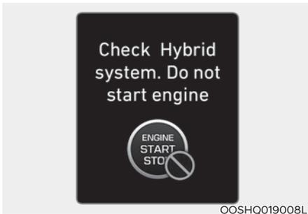
This message is displayed when the hybrid battery power (SOC) level is low. A warning chime will sound until the problem is solved. Refrain from driving when the warning message is displayed. If this occurs, you have the vehicle inspected by an authorized HYUNDAI dealer.
