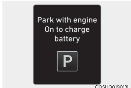
This message is displayed when the hybrid battery power (SOC) level is low. If this occurs, park the vehicle in a safe location and wait until the hybrid battery is charged.
