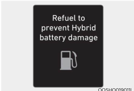
This message is displayed when the fuel tank is nearly empty. You should refill the fuel tank to prevent hybrid battery damage.
