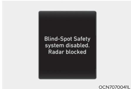
When the rear bumper around the rear corner radar or sensor is covered with foreign material, such as snow or rain, or installing a trailer or carrier, it can reduce the detecting performance and temporarily limit or disable Safe Exit Warning.
