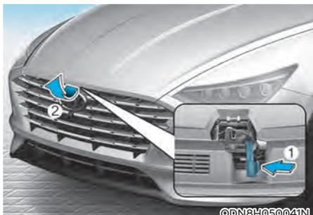
3. Go to the front of the vehicle, raise the hood slightly, push up the secondary latch (1) inside of the hood center and lift the hood (2). After it has been raised about halfway, it will raise completely by itself.
