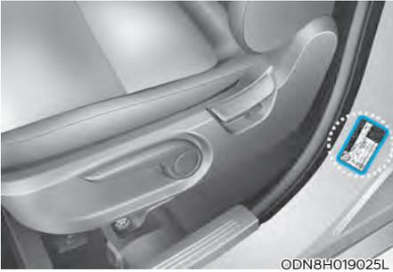
The tires supplied on your new vehicle are chosen to provide the best performance for normal driving. The tire label located on the driver's side center pillar gives the tire pressures recommended for your car.
