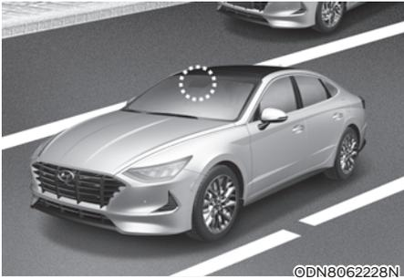
Lane Following Assist helps detect lane markers on the road with a front view camera at the front windshield, and assists the driver's steering to help keep the vehicle between lanes.
