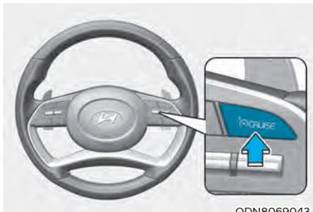
1. Push the CRUISE/
