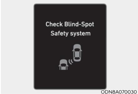
When Safe Exit Warning is not working properly, the 'Check Blind-Spot Safety system' warning message will appear on the cluster, function will turn off automatically function will be limited. Have the vehicle inspected by an authorized HYUNDAI dealer.
