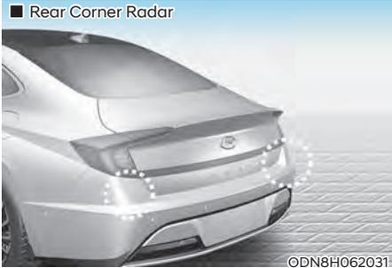
The rear corner radars are the sensors inside the rear bumper for detecting the side and rear areas. Always keep the rear bumper clean for proper operation of Rear Cross-Traffic Collision-Avoidance Assist.
