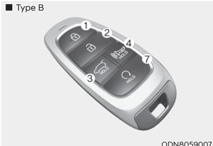
Your HYUNDAI uses a smart key, which you can use to lock or unlock a door (and trunk) and even start the engine even just carrying the key.
