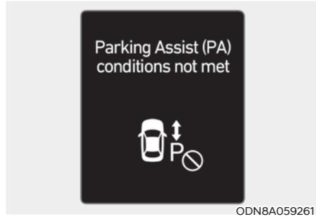
When Remote Smart Parking Assist is not getting ready for activation, the above message will appear when Remote Smart Parking Assist button is pressed.
