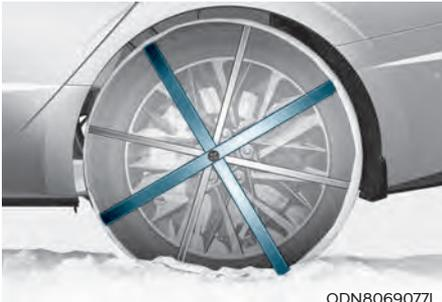
Since the sidewalls of radial tires are thinner than other types of tires, they may be damaged by mounting some types of tire chains on them. Therefore the use of snow tires is preferred over the use of tire chains.
