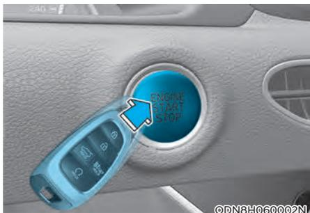
If the smart key battery is weak or the smart key does not work correctly, you can start the engine by pressing the Engine Start/Stop button with the smart key in the direction of the picture above.
