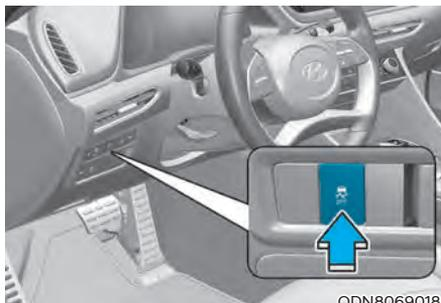
The Electronic Stability Control (ESC) system helps to stabilize the vehicle during cornering maneuvers. ESC checks where you are steering and where the vehicle is actually going. ESC applies braking pressure to any one of the vehicle's brakes and intervenes in the engine management system to assist the driver with keeping the vehicle on the intended path. It is not a substitute for safe driving practices. Always adjust your speed and driving to the road conditions.
