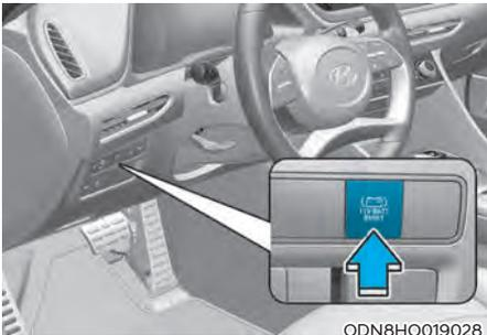
7. Press the 12V Battery Reset switch.
