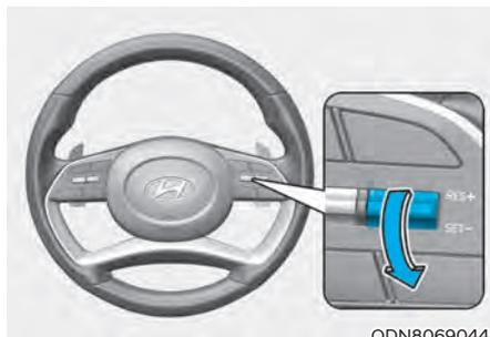
3. Push the SET- switch down. The Set Speed and Headway on the LCD display will illuminate.
