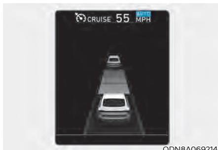
If the vehicle decelerates in a curve, the **AUTO** symbol on the cluster will illuminate green.
