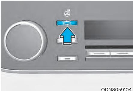
When the ignition switch is in the ON position or when the engine is running, press the heated steering wheel button to warm the steering wheel. The indicator on the button will illuminate.
