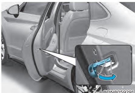
If the electrical power door lock switch is not operating (ex. dead car battery) the only way to lock the door(s) is with the mechanical key from the outside key hole.
