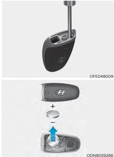
If the Smart Key is not working properly, try replacing the battery with a new one.
