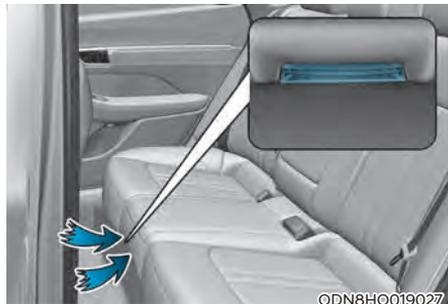
The hybrid battery cooling duct is located on the left side of the rear seats. The cooling duct cools down the hybrid battery. When the hybrid battery cooling duct is blocked, the hybrid battery may be overheated.
