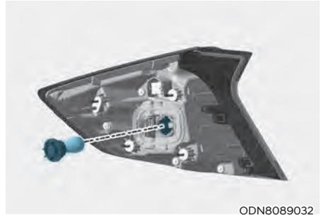
3. Remove the socket from the assembly by turning the socket counterclockwise until the tabs on the socket align with the slots on the assembly.
