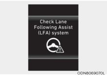
Check LFA (Lane Following Assist) system If there is a problem with the system a message will appear for a few seconds. If the problem continues LFA system failure indicator will illuminate.
