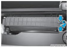
3. Remove the climate control air filter case while pressing the lock on the right side of the cover.
