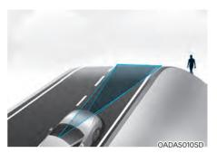
The performance of Forward Collision-Avoidance Assist system may be decreased while driving upward or downward on a slope.
