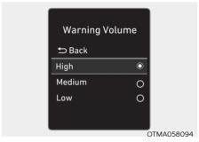
The driver can select the warning volume of Forward Collision Warning in the User Settings in the
