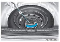
If it is hard to loosen the tire hold-down wing bolt by hand, you can loosen it easily using the wheel nut wrench. Turn the tire hold-down wing bolt counterclockwise with the wheel nut wrench.
