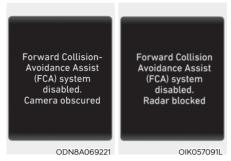
Forward Collision-Avoidance Assist (FCA) system disabled. Camera obscured / Radar blocked
