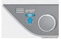
If you press the DRIVER ONLY button (\$\mathbb{G}^{DRIVER}\)) and the indicator light illuminates, air mostly blows in the direction of the driver's seat.
