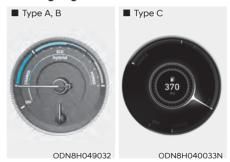
The power gauge indicates whether the current driving condition is fuel efficient or not.
