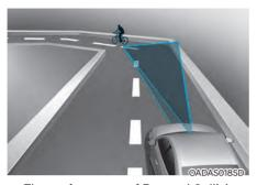
The performance of Forward Collision-Avoidance Assist system may be limited when driving on a curved road.
