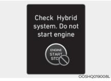
This message is displayed when the hybrid battery power (SOC) level is low. A warning chime will sound until the problem is solved. Refrain from driving when the warning message is displayed.
