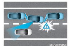
Blind-Spot Collision-Avoidance Assist system detects the front lane through the front view camera installed on the upper front windshield and detects the side/ rear areas through rear corner radars. Blind-Spot Collision-Avoidance Assist system may activate the Electronic Stability Control (ESC) in accordance with a colliding possibility with an approaching vehicle while changing lanes. It is to lower the colliding risk or help mitigate the colliding damage.
