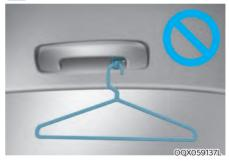
Do not hang other objects such as hangers or hard objects except clothes. Also, do not put heavy, sharp or breakable objects in the clothes pockets. In an accident or when the curtain air bag is inflated, it may cause vehicle damage or personal injury.
