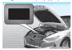
You can find out which air conditioning refrigerant is applied to your vehicle on the label located in front of the engine compartment.
