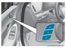
The Driver Position Memory System is provided to store and recall the following memory settings with a simple button operation.
