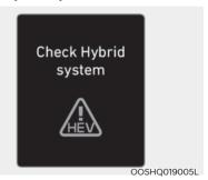
This message is displayed when there is a problem with the hybrid control system. Refrain from driving when the warning message is displayed.
