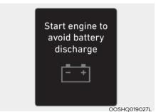
This message is displayed to inform the driver the 12V battery may be discharged if the ignition switch is in ON position (without the findicator ON).
