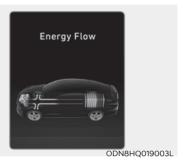
Both the motor and the engine power are used to drive the vehicle.
