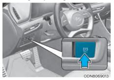
To release the EPB (Electronic Parking Brake):
