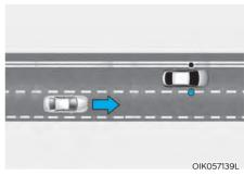
BCW system will alert you when a vehicle is detected approaching in an adjacent lane at a high rate of speed. If the driver activates the turn signal when the system detects an oncoming vehicle, the system sounds an audible alert.
