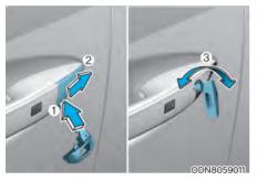
If you lock or unlock the driver's door with a mechanical key, you can open and close the driver's door only.
