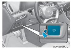
To apply the EPB (Electronic Parking Brake):
