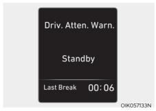
Driver Attention Warning system enters the ready status and displays the 'Standby' screen in the following situations.
