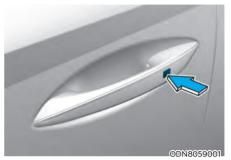
Press the button on the driver's outside door handle or touch the touch sensor on the door handle (the engraved part) while carrying the Smart Key with you or press the Door Unlock button on the Smart Key, the driver's door will unlock.
