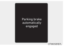
Parking brake automatically engaged When the EPB is applied from Auto Hold, a warning will sound and a message will appear.
