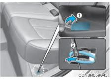
Open the cable cover(1) under the rear seat with a mechanical key and pull the cable (2) for unlocking the trunk.
