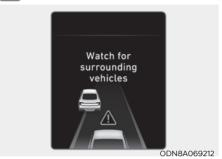
If the vehicle ahead (vehicle speed: less than 20 mph (30 km/h)) disappears to the next lane, the warning chime will sound and a message "Watch for surrounding vehicles" will appear. Adjust your vehicle speed for vehicles or objects that can suddenly appear in front of you by depressing the brake pedal.
