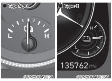
This gauge indicates the remaining hybrid battery power. If the SOC is near the "0 or L (Low)" level, the vehicle automatically operates the engine to charge the battery.
