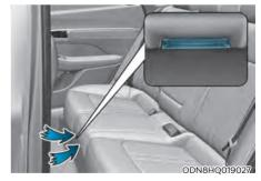
The hybrid battery cooling duct is located on the left side of the rear seats. The cooling duct cools down the hybrid battery. When the hybrid battery cooling duct is blocked, the hybrid battery may be overheated.
