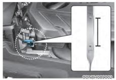
6. Pull the dipstick out again and check the level. The level should be between F (Full) and L (Low).
