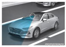
Lane Keeping Assist system detect lane markers on the road with a camera at the front windshield, and assists the driver's steering to help keep the vehicle between lanes.
