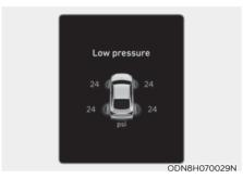
When the tire pressure monitoring system warning indicators are illuminated and a warning message displayed on the cluster LCD display, one or more of your tires is significantly under-inflated. The Low Tire Pressure Position Telltale will indicate which tire is significantly underinflated by illuminating the corresponding position light.
