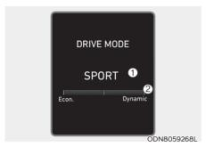
The drive mode selected by the driver (1) and the driving style gauge (2) showing the driver's driving style are displayed on the screen.
