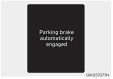
Parking brake automatically engaged If the EPB is applied while Auto Hold is activated, a warning will sound and a message will appear.
