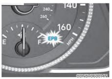
This warning light illuminates if the ignition switch is set to the ON position and goes off in approximately 3 seconds if the system is operating normally.
