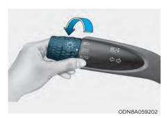
Parking lamp position (-)0(-) The parking lamp, license plate lamp and instrument panel lamp are turned ON.
