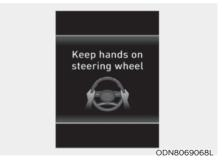
Keep hands on steering wheel If the driver takes their hands off the steering wheel for several seconds while LKA system is activated, the system will warn the driver.
