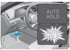
2. When you stop the vehicle completely by depressing the brake pedal, the Auto Hold maintains the brake pressure to hold the vehicle stationary. The indicator changes from white to green.
