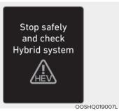
This message is displayed when there is a problem with the hybrid control system. The "\(\frac{1}{4}\)" indicator will blink and a warning chime will sound until the problem is solved. Refrain from driving when the warning message is displayed.
