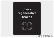
This message is displayed when the brake performance is low or the regenerative brake does not work properly due to a problem in the brake system.
