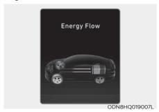
The high-voltage battery is charged up by the regenerative brake system.
