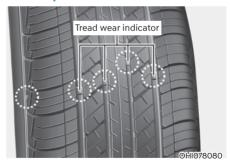
If the tire is worn evenly, a tread wear indicator will appear as a solid band across the tread. This shows there is less than 1/16 inch (1.6 mm) of tread left on the tire. Replace the tire when this happens.
