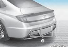
[A]: Front sensor, [B]: Rear sensor
