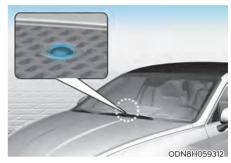
When the solar roof is on, the lamp installed in the upper part of the crash pad illuminates.
