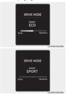
With the standard driving style in the center, the left side of the gauge is 'Econ.' and right side is 'Dynamic' style.
