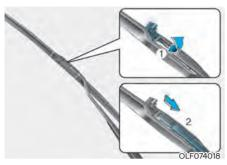
3. Lift up the wiper blade clip. Then pull down the blade assembly and remove it.
