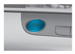
Whenever the front door is opened, the Push Button Start ignition switch illuminates and goes off 30 seconds after the door is closed. (if equipped)
