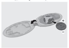
Reinstall the rear cover of the smart key. If you suspect your smart key might have sustained some damage, or you feel your smart key is not working correctly, contact an authorized HYUNDAI dealer.
