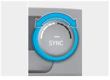
The temperature will increases by turning the knob to the right.
