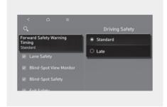
With the ignition switch ON, go to User Settings > Driver Assistance > Driving Safety > Forward Safety Warning Timingfrom the settings menu in the instrument cluster or Settings > Vehicle > Driver Assistance > Driving Safety > Forward Safety Warning Timing settings menu in the infotainment system to change the initial warning activation time. Warning Timing is set to Standard at the factory.
