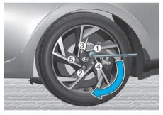
13.Use the wheel lug wrench to tighten the wheel nuts in the order shown. Double-check each wheel nuts until they are tight. After changing tires, have an authorized HYUNDAI dealer tighten the wheel nuts to their proper torque as soon as possible. Tighten the wheel nuts to 79-94 lbf.ft (11-13 kgf.m).
