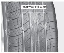
If the tire is worn evenly, a tread wear indicator appears as a solid band across the tread. This shows there is less than 1/16 in. (1.6 mm) of tread left on the tire. Replace the tire when this happens.
