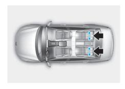
LATCH anchors have been provided in the left and right outboard rear seating positions. Their locations are shown in the illustration. There are no LATCH anchors provided for the center rear seating position.
