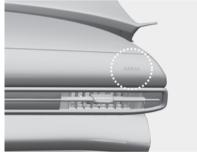
The SRS consists of advanced airbags located in the center of the steering wheel and the passenger's side front panel pad above the glove box.
