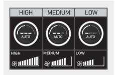
You can control the blower strength in three stages by pressing the AUTO button during automatic operation.
