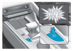
Press the AUTO HOLD switch. The white AUTO HOLD indicator comes on and the system is in standby.
