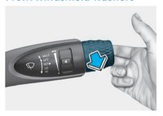
In the OFF position, pull the lever gently toward you to spray washer fluid on the windshield and to run the wipers 1-3 cycles. The spray and wiper operation continues until you release the lever. If the washer does not work, you may need to add washer fluid to the washer fluid reservoir.
