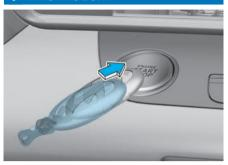
If the smart key battery is weak or the smart key does not work correctly, press the Push Button Start ignition switch with the smart key.
