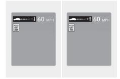
If the speed limit changes when using Manual Speed Limit Assist or Smart Cruise Control, an arrow in the direction of up or down appears to inform you to change the set speed by pushing the + or - switch.
