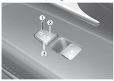
When pressing the  $(\frac{1}{1})$  portion (1) on the switch, all vehicle doors are locked.
