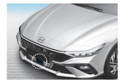
The front radar is mounted behind the front grill.
