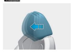
The head restraint can be adjusted forward to 3 different positions by pulling the head restraint forward to the desired detent. To adjust the head restraint to it's furthest rearwards position, pull it fully forward to the farthest position and release it.
