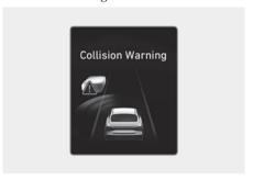
If Forward Collision-Avoidance Assist judges that a collision may occur, the message may appear on the instrument cluster and an audible warning is heard and the steering wheel may vibrate when:
