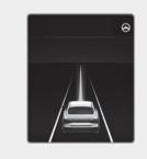
If both the lane markings and/or the vehicle ahead are detected and your vehicle speed is below 120 mph (200 km/h), Lane Following Assist helps center your vehicle in the lane by assisting with steering. The green indicator light illuminates on the instrument cluster.
