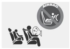
Even though your vehicle is equipped with the OCS, never install a Child Restraint System in the front passenger's seat. An inflating airbag may forcefully strike a child or child restraint resulting in serious or fatal injury.
