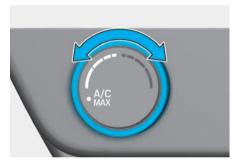
The temperature increases by turning the knob to the right.
