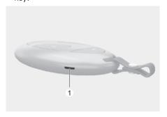
Remove the old battery and insert a new battery. Make sure the battery position is correct. An improperly positioned battery may discharge the battery, causing smart key failure.
