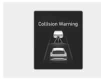
If Forward Collision-Avoidance Assist judges that a collision may occur, the message may appear on the instrument cluster and an audible warning is heard and the steering wheel may vibrate when:
