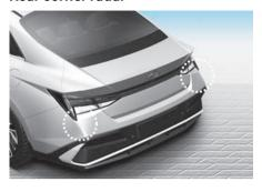
The rear corner radars are mounted near the rear corners of your vehicle above the bumper.
