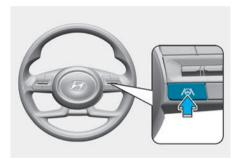
With the engine ON, press and hold the Driving Assist button located on the steering wheel to turn on and off. The grey or green indicator light illuminates on the instrument cluster when the function is on.
