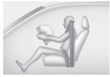
When the SRSCM detects a sufficiently severe impact to the front of the vehicle, it automatically deploys the front airbags.
