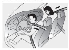
Your vehicle is equipped with Pretensioner seat belts (retractor pretensioner). The pretensioner helps the driver's, front passenger's, and outboard rear seat belt fit tightly against your body in certain frontal or side collision(s).
