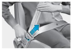
Press the release button (1) in the locking buckle.
