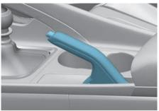
Check the stroke of the parking brake by counting the number of "clicks" heard while fully applying it from the released position. Also, the parking brake alone should securely hold the vehicle on a fairly steep grade. If the stroke is more or less than specified, have the system be inspected by an authorized HYUNDAI dealer.
