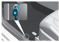
The fuel filler door must be opened from inside the vehicle by pulling up the fuel filler release lever.
