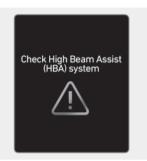
When High Beam Assist is not working properly, the "Check High Beam Assist (HBA) system" warning message may appear, and the \( \bar{\Lambda} \) warning light may illuminate on the instrument cluster. Contact an authorized HYUNDAI dealer.
