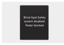
If the rear corner radar is blocked or covered, or when the rear bumper around the rear corner radar or sensor is covered by any foreign material, such as snow, rain, or dirt, or when a trailer or hitch mounted carrier is installed, the detecting performance may decrease and temporarily limit or disable Blind-Spot Collision-Avoidance Assist.
