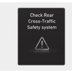
When the Rear Cross-Traffic Collision-Avoidance Assist is not working properly, the "Check Rear Cross-Traffic Safety system" warning message may appear, and the \(\text{\Lambda}\) warning light may illuminate on the instrument cluster. Have the vehicle inspected by an authorized HYUNDAI dealer.
