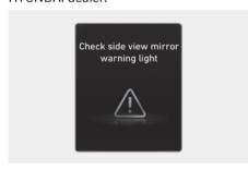
When the side view mirror warning light is not working properly, the "Check side view mirror warning light" warning message may appear, and the \(\begin{align\*}\) warning light may illuminate on the instrument cluster. Have the vehicle inspected by an authorized HYUNDAI dealer.
