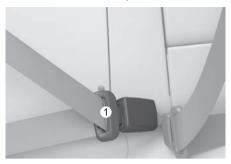
Insert the tongue plate (1) into the buckle until an audible "click" is heard, indicating the latch is locked. Pull the shoulder portion of the belt to snug the belt across your hips and remove slack. Make sure the seat belt is not twisted.
