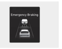
If Forward Collision-Avoidance Assist judges avoiding a collision may be difficult, it applies higher brake force that may help avoid a collision with the vehicle, pedestrian, or cyclist detected ahead.
