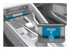
While the engine is running, press the switches to warm the driver's seat or front passenger's seat.
