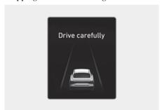
After your vehicle has stopped following an Emergency Braking event, the "Drive carefully" warning message may appear on the instrument cluster.
