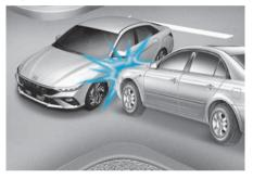
Front airbags may not inflate in side impact collisions, because occupants move in the direction of the collision. Side and curtain airbags may inflate depending on the severity of impact.
