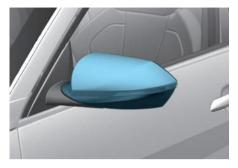
Your vehicle is equipped with both left-hand and right-hand side view mirrors. The mirrors can be adjusted remotely with the remote switch. The side view mirrors can be folded to help prevent damage when going through an automatic car wash or when passing through a narrow street.
