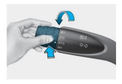
High Beam Assist automatically adjusts the headlights between high beam and low beam depending on the light detected from oncoming vehicles or vehicles in front using the front view camera.
