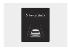
After your vehicle is stopped following an Emergency Braking event, the "Drive carefully" warning message may appear on the instrument cluster.
