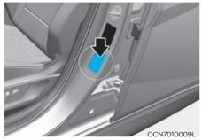
All specifications (sizes and pressures) can be found on a label attached to the driver's side center. nillar.
