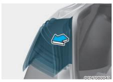
Remove the rear combination light assembly from the body of the vehicle.
