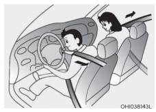
Your vehicle is equipped with driver's and front passenger's and rear passenger's Pre-tensioner Seat Belts (Retractor Pre-tensioner). The purpose of the pretensioner is to make sure the seat belts fit tightly against the occupant's body in certain frontal or side collision(s).
