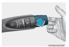
In the OFF position, pull the lever gently toward you to spray washer fluid on the windshield and to run the wipers 1-3 cycles. The spray and wiper operation will continue until you release the lever. If the washer does not work, you may need to add washer fluid to the washer fluid reservoir.
