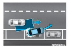
When you are driving forward out of a parking space, if Blind-Spot Collision-Avoidance Assist judges that there is a collision risk with an approaching vehicle in the blind spot, Blind-Spot Collision-Avoidance Assist will help avoid collision by applying the brake.
