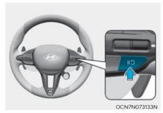
Press the II S switch to temporarily pause the set speed limit. The set speed limit will turn off but the Manual Speed Limit Assist (© LIMIT) indicator will stay on.
