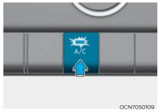
Press the A/C button to turn the air conditioning system on (indicator light will illuminate). Press the button again to turn the air conditioning system off.
