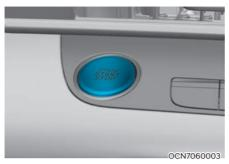
Whenever the front door is opened, the Engine Start/Stop button will illuminate and will go off 30 seconds after the door is closed.
