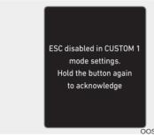
When N1 or N2 button is set to CUSTOM mode, you cannot turn CUSTOM mode on by pressing either N1 or N2 button if ESC OFF setting is saved within CUSTOM mode. If N1 or N2 button is pressed, a message "ESC disabled in CUSTOM 1 (or 2) mode settings. Hold the button again to acknowledge" appears on the cluster display. To turn on CUSTOM mode with ESC OFF setting, press and hold N1 or N2 button.
