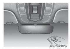
Position the garage door opener remote 1 – 3 inches (2 – 8cm) away from the HoleLink buttons.
