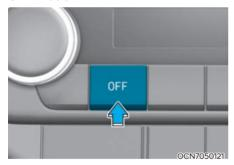
Push the OFF button of the front to turn off the air climate control system. However, you can still operate the mode and air intake buttons as long as the Engine Start/Stop button is in the ON position.
