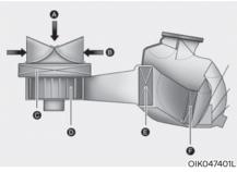
[A]: Outside air, [B]: Recirculated air [C]: Cabin air filter, [D]: Blower [E]: Evaporator core, [F]: Heater core
