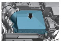
The air cleaner filter can be cleaned for inspection using compressed air. Do not attempt to wash or to rinse it, as water will damage the filter. If soiled, the air cleaner filter must be replaced.
