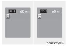
If the speed limit of the road changes during the operation of Manual Speed Limit Assist an arrow in the direction of up or down is displayed to inform the driver that the set speed needs to be changed. At this time, the driver can change the set speed according to the speed limit by using the + or - switch on the steering wheel.
