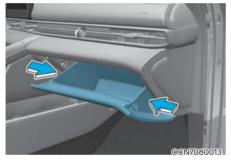
Push in both sides of the glove box as shown. This will ensure that the glove box stopper pins will get released from its holding location allowing the glove box to hang.
