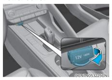
The power outlet is designed to provide power for mobile telephones or other devices designed to operate with vehicle electrical systems. The devices should draw less than 180 W with the engine runnina.
