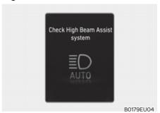
When High Beam Assist is not working properly, the 'Check High Beam Assist system' warning message will appear and A warning light will illuminate on the cluster. Have the vehicle inspected by an authorized HYUNDAI dealer.
