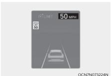
Manual Speed Limit Assist assists the vehicle to adjust its speed according to the speed limit. When the cruising speed is set as same as the speed limit, the vehicle automatically adjusts its speed if the speed limit changes. The function operates on the road which has a speed limit of 44 mph (70 km/h) or higher. When the function is active, the set speed on the instrument cluster appears in green.
