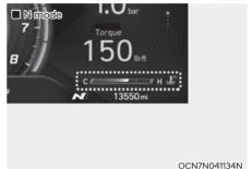
This gauge indicates the temperature of the engine coolant when the Engine Start/Stop button is in the ON position.
