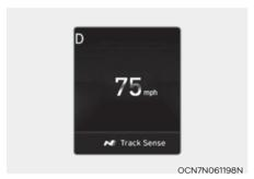
\* When N Track Sense Shift is operating, a message is displayed in the cluster display as shown below.
