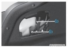
3. Loosen the assembly retaining nuts.
