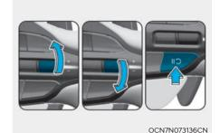
Operate the +, - switch or II button. If you push the + switch up or - switch down, vehicle speed will be set to the current speed on the instrument cluster.
