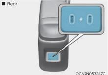
The USB charger is located inside the console box between the driver's seat and the front passenger's seat. Insert the USB charger into the USB port, and recharge a smartphone or a tablet PC.
