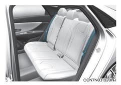
3. Route the seat belt webbing through the rear seat belt guides to prevent the belts from being trapped behind or under the seats.
