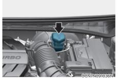
Check the fluid level in the reservoir periodically. The fluid level should be between MAX and MIN marks on the side of the reservoir.
