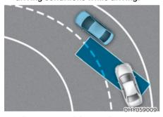
Blind-Spot Collision-Avoidance Assist may not operate properly when driving on a curved road. Blind-Spot Collision-Avoidance Assist may recognize a vehicle in the same lane.
