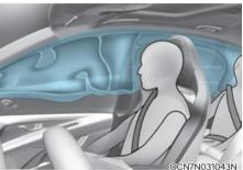
Curtain air bags are located along both sides of the roof rails above the front and rear doors.
