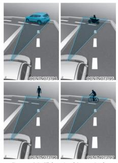
Forward Collision-Avoidance Assist may detect a vehicle, a powered two-wheeler, a pedestrian or a cyclist in the next lane or outside the lane when driving on a curved road. If this occurs, Forward Collision-Avoidance Assist may unnecessarily warn the driver and control the brake. Always check the traffic conditions around the vehicle.
