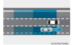
Blind-Spot Collision-Avoidance Assist helps detect and inform the driver that a vehicle is in the blind spot.
