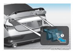
4. Pull on the seatback folding lever (1) located in the trunk.
