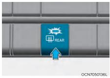
The defroster heats the window to remove frost, fog and thin ice from the interior and exterior of the rear window, while engine is running.
