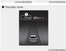
Highway Driving Assist indicator, whether there is a vehicle ahead and the selected distance level are displayed.
