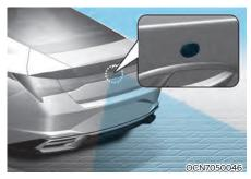
The rear view camera is used as a detecting sensor to detect pedestrians. If the camera lens is covered with foreign material, such as snow or rain, it may adversely affect camera performance and Reverse Parking Collision-Avoidance Assist may not operate properly. Always keep the camera lens clean.
