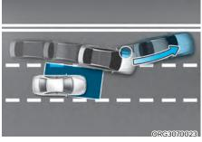
When changing lanes by detecting the lane ahead, if the system judges that there is a collision risk with an approaching vehicle in the blind spot, the function can help avoid a collision by applying the brake.
