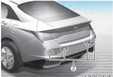
[1]: Rear view camera, [2]: Rear ultrasonic sensors
