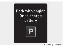
This message is displayed when the hybrid battery power (SOC) level is low. If this occurs, park the vehicle in a safe location and wait until the hybrid battery is charged.
