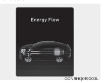
Both the motor and the engine power are used to drive the vehicle.
