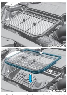
2. Replace the air cleaner filter. Insert (2) completely into (3).
