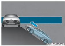
Rear Cross-Traffic Safety system may be limited when the vehicle is on a uphill or downhill slope, or near it, and may not detect the vehicle approaching from the left or right. If this occurs, the system may not warn the driver or control the brakes when necessary.
