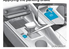
To apply the EPB (Electronic Parking Brake):
