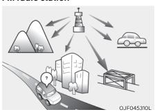
FM broadcasts are transmitted at high frequencies and do not bend to follow the earth's surface. Because of this, FM broadcasts generally begin to fade at short distances from the station. Also, FM signals are easily affected by buildings, mountains, or other obstructions.
