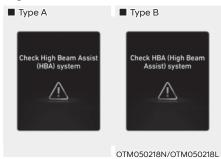
When High Beam Assist is not working properly, the 'Check High Beam Assist (HBA) system' or 'Check HBA (High Beam Assist) system' warning message will appear and \( \ulder \) warning light will illuminate on the cluster. Take your vehicle to an authorized HYUNDAI dealer and have the function checked.
