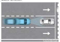
Forward Collision-Avoidance Assist is designed to help detect and monitor the vehicle ahead or detect a pedestrian in the roadway and warn the driver that a collision is imminent with a message, audible warning and apply emergency braking.
