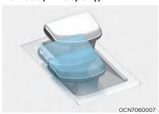
To shift into Ds mode, move the shift lever from D (Drive) to the center of the manual shift mode. The engine and transmission control logic is automatically optimized for sporty driving.
