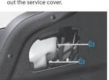
3. Loosen the assembly retaining nuts.
