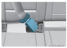
When using the rear center seat belt, the buckle with the "CENTER" mark must be
