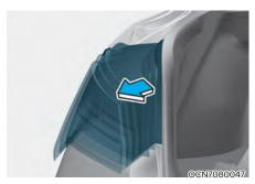
4. Remove the rear combination light assembly from the body of the vehicle.
