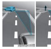
Forward Collision-Avoidance Assist may not detect other vehicles or pedestrians in front of you when driving on curved roads adversely affecting the performance of the sensors. This may result in no warning or braking assist when necessary.
