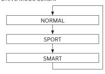
When NORMAL mode is selected, it is not displayed on the instrument cluster.
