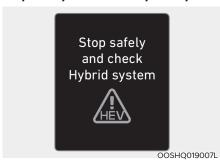
This message is displayed when there is a problem with the hybrid control system. The "#" indicator will blink and a warning chime will sound until the problem is solved. Refrain from driving when the warning message is displayed.
