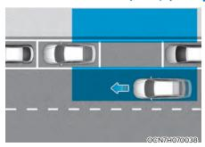
After the vehicle stops, when an approaching vehicle from the rear area is detected after a passenger opens the door, Safe Exit Assist will warn the driver with a warning message and an audible warning to help prevent a collision.
