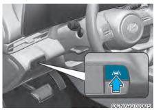
With the engine on, press the Lane Safety button located on the instrument panel to turn on Lane Keeping Assist. The white Aniocator light will illuminate on the cluster.
