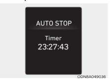
This mode displays the Auto Stop accumulated time within ISG vehicles.
