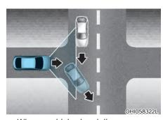
When a vehicle ahead disappears at an intersection, your vehicle may accelerate.
