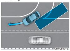
Blind-Spot Safety system may not operate properly when driving where the road merges or divides. The system may not detect the vehicle in the next lane.
