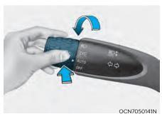
High Beam Assist will automatically adjust the headlamp range (switches between high beam and low beam) depending on the brightness of detected vehicles and certain road conditions.
