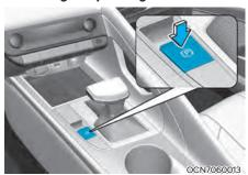
To release the EPB (Electronic Parking Brake):
