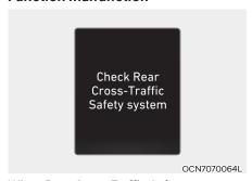
When Rear Cross-Traffic Safety system is not working properly, the 'Check Rear Cross-Traffic Safety system' warning message will appear on the cluster for several seconds, and the master (A) warning light will illuminate on the cluster. If this occurs, have the vehicle inspected by an authorized HYUNDAI dealer.
