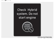
This message is displayed when the hybrid battery power (SOC) level is low. A warning chime will sound until the problem is solved. Refrain from driving when the warning message is displayed.
