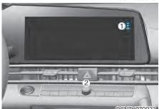
The driver is able to check the rear view on the screen while driving, it is to assist with backing up.
