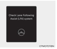
When Lane Following Assist is not working properly, the 'Check Lane Following Assist (LFA) system' warning message will appear on the cluster for several seconds, and the master (A) warning light will illuminate on the cluster. If this occurs, have the vehicle inspected by an authorized HYUNDAI dealer.
