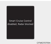
When the front radar cover or sensor is covered with snow, rain, or foreign material, it can reduce the detecting performance and temporarily limit or disable Smart Cruise Control.
