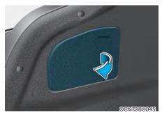
2. Remove the service cover by pulling out the service cover.
