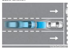
Forward Collision-Avoidance Assist is designed to help detect and monitor the vehicle ahead or help detect a pedestrian or cyclist in the roadway and warn the driver that a collision is imminent with a message, and an audible message, emergency braking.
