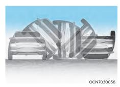
Front air bags may not inflate in rollover accidents because air bag deployment may not provide protection to the occupants.
