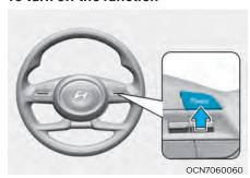
Press the Driving Assist button to turn Cruise Control off. The Cruise (\*\*CRUISE) indicator will go off.
