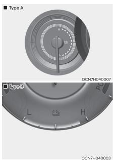
This gauge indicates the remaining hybrid battery power. If the SOC is near the "0 or L (Low)" level, the vehicle automatically operates the engine to charge the battery.
