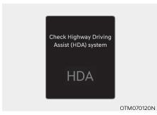
When Highway Driving Assist is not working properly, the 'Check Highway Driving Assist (HDA) system' warning message will appear, and the \( \triangle \) warning light will illuminate on the cluster. Have the vehicle inspected by an authorized HYUNDAI dealer.
