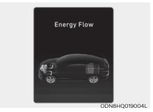
Only the engine power is used to drive the vehicle.
