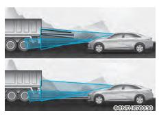
In the following cases, the vehicle in front cannot be detected by the sensor:
