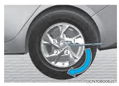
13. Use the wheel lug nut wrench to tighten the lug nuts in the order shown. Double-check each lug nut until they are tight. After changing tires, have an authorized HYUNDAI dealer tighten the lug nuts to their proper torque as soon as possible. The wheel lug nut should be tightened to 79~94 lbf-ft (11~13 kgf-m).
