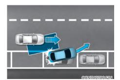
When you are driving forward out of a parking space, if the system detects that there is a collision risk with an approaching vehicle in the blind spot, the function can help avoid a collision by applying the brake.
