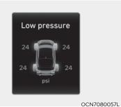
When the tire pressure monitoring system warning indicators are illuminated and a warning message displayed on the cluster LCD display, one or more of your tires is significantly under-inflated. The Low Tire Pressure Position Telltale will indicate which tire is significantly underinflated by illuminating the corresponding position
