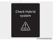
This message is displayed when there is a problem with the hybrid control system. Refrain from driving when the warning message is displayed.
