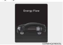
When the vehicle is stopped, the highvoltage battery is charged up by the engine.
