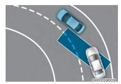
Blind-Spot Safety system may not operate properly when driving on a curved road. The system may recognize a vehicle in the same lane.
