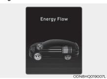
The high-voltage battery is charged up by the regenerative brake system. (Wheel → Battery)
