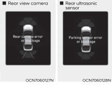
The 'Rear camera error or blockage' or 'Parking sensor error or blockage' warning message will appear on the cluster if the following situations occur:
