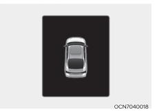
If the driver turns off the engine when the sunroof is not fully closed, the warning chime will sound for several seconds and the sunroof open warning will appear on the cluster LCD display.
