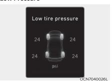
This warning message is displayed if the tire pressure is low. The corresponding tire on the vehicle will be illuminated.
