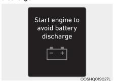
This message is displayed to inform the driver the 12V battery may be discharged if the ignition switch is in ON position (without the indicator ON).
