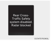
When the rear bumper around the rearside radar or sensor is covered with foreign material, such as snow or rain, or installing a trailer or carrier, it can reduce the detecting performance and temporarily limit or disable Rear Cross-Traffic Safety system.
