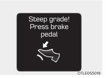
This warning message is displayed when vehicle is driven slowly on a grade and the vehicle detects that the brake pedal is not applied.
