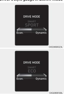
With the standard driving style in the center, the left side of the gauge is 'Econ.' and right side is 'Dynamic' style.
