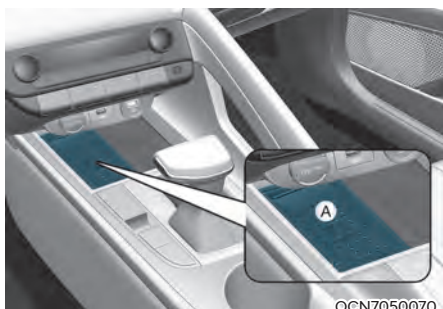
[A] : Charging pad
