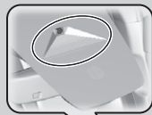
■ Front Sensor Camera Monitors the lane lines
