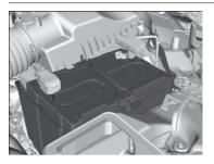
Check the battery terminals for corrosion monthly.
