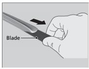
**3.** Slide the wiper blade out from its holder by pulling the tabbed end out.
