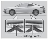
**1.** Place the jack under the jacking point closest to the tire to be changed.
