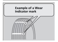
The groove where the wear indicator is located is 1/16 inch (1.6 mm) shallower than elsewhere on the tire. If the tread has worn so that the indicator is exposed, replace the tire. Worn out tires have poor traction on wet roads.
