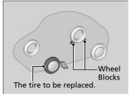
**4.** Place a wheel block or rock in front and rear of the wheel diagonal to the flat tire.
