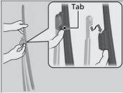
**2.** Press and hold the tab, then slide the blade from the wiper arm.
