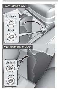
The floor mats for the driver, and the rear passenger on the passenger's side hook over the floor anchors, which keep the mats from sliding forward. To remove a mat for cleaning, turn the anchor knobs to the unlock position. When reinstalling the mat after cleaning, turn the knobs to the lock position.
