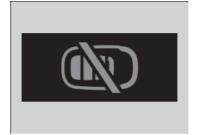
When the power mode is set to any mode other than OFF and you remove the keyless remote from the vehicle and shut the door, an alarm will sound. If the alarm continues to sound, place the keyless remote in another location.
