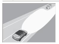
When driving at night, the front wide view camera detects light sources such as street lights or the lights of an oncoming or preceding vehicle. The system automatically switches the headlights between low and high beam depending on the situation. In addition, the system automatically adjusts the light distribution of the high beams in order to reduce glare for preceding and oncoming vehicles.
