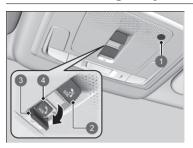
If you need to make an emergency call, you can establish a connection manually: Press the **SOS** button and hold it for more than 0.5 seconds.
