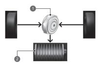
When decelerating without the accelerator being depressed or the brake pedal being applied, or while driving downhill, the electric motor acts as a generator that recovers a portion of the electrical energy that was used to accelerate the vehicle. This regenerative braking slows the vehicle in a manner similar to engine braking in a petrol-powered vehicle. You can control the rate of deceleration by using the deceleration paddle selector.
