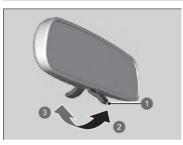
Flip the tab to switch the position.
