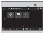
**2.** A notification icon is continuously displayed in the header area until the new message is read.
