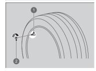
**4.** Remove the valve cap from the tyre valve stem.
