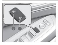
Press the master door lock switch in as shown to lock or unlock all the doors and the tailgate.
