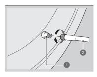
**5.** Attach the air hose onto the tyre valve stem. Screw it until it is tight.
