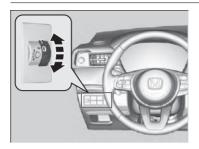
You can adjust the vertical angle of the low beam headlights when the position lights or headlights are on.
