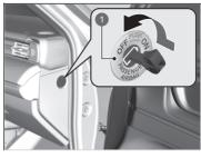
Passenger Front Airbag ON/ OFF Switch
