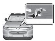
When finished, close the bonnet and make sure it is firmly locked in place.
