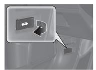
2 Locate the bonnet latch lever, push it to the side, and then raise the bonnet. Once you have raised the bonnet slightly, you can release the lever.
