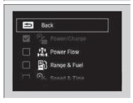
**3.** Roll the left selector wheel to scroll between icons, then press the left selector wheel to check or uncheck them.
