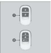
Use the keys to turn on and off the power system, and to lock and unlock all the doors and tailgate.
