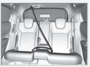
If a Child Restraint System is installed in one of the outer seats, it may cover the centre seat belt buckle or anchorage buckle.
