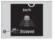
Your vehicle also stops, automatically. The **Stopped** message appears on the gauge. When the vehicle ahead of you starts again, if you press the **RES/+** or **SET/-** button, or depress the accelerator pedal, ACC with Low Speed Follow operates again within the previously set speed.
