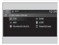
Select **Audio Source** in the header area, then select an icon on the source list to switch the audio source.
