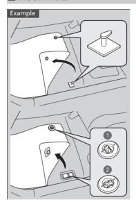
The driver's floor mat hooks over the floor anchorages, which keep the mat from sliding forward.
