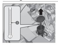
Check the amount of window washer fluid using the washer fluid level gauge on the cap.
