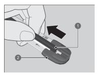
**3.** Pull the end of the wiper blade in the direction of the arrow in the image until it is out of the holder's end cap.
