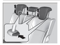
A passenger sitting in the rear seat seating position should adjust the height of their head restraint to an appropriate position before the vehicle begins moving.
