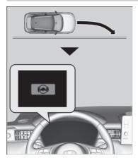
The front wide view camera behind the rearview mirror monitors left and right lane markings in white or yellow, the outer edge of the pavement (bordered by grass or gravel) or a detected oncoming vehicle.
