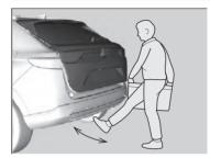
Use a forward and back kicking motion for about 1 second under the centre of the rear bumper to open or close the power tailgate while carrying the keyless remote.
