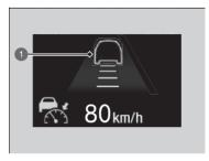
1 A vehicle icon with line contour appears on the gauge.
