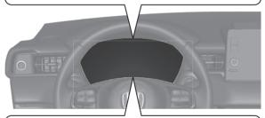
**Shift Position Indicator** The shift position indicator indicates the current shift selection.
