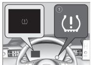
This will cause the low tyre pressure/deflation warning system indicator to come on and a message to appear on the gauge.
