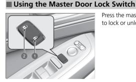
Press the master door lock switch in as shown to lock or unlock all the doors and the tailgate.
