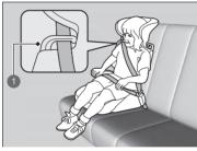
and adjust it to the vehicle seat according to the booster seat manufacturer's instructions. Make sure the seat belt is properly routed through the guide at the shoulder of the backrest and the belt does not touch and cross the child's neck.
