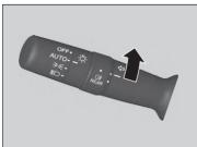
**To turn the rear fog lights on:**Rotate the switch to ()‡. The ()‡ indicator comes on.
