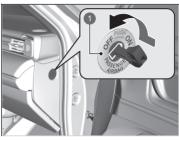
Passenger Front Airbag ON/ OFF Switch
