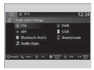
Select **Audio Source** on the header area, then select an icon on the source list to switch the audio source.
