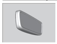
When you are driving after dark, the automatic dimming rearview mirror reduces the glare from headlights behind you, based on inputs from the mirror sensor. This feature is always active.
