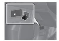
2 Turn the fuel fill cap slowly to remove the cap.
