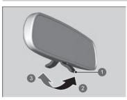
Flip the tab to switch the position.
