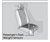
The front passenger's advanced airbag system has weight sensors. The sensors are used for occupant classification to activate or deactivate the front passenger's airbag.
