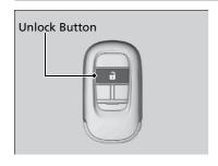
Press the unlock button, and then within 10 seconds, press it again and hold it.
