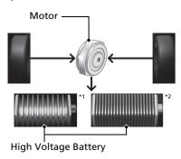
When decelerating without the accelerator being depressed or the brake pedal being applied, or while driving downhill, the electric motor acts as a generator that recovers a portion of the electrical energy that was used to accelerate the vehicle. This regenerative braking slows the vehicle in a manner similar to engine braking in a gasoline-powered vehicle. You can control the rate of deceleration by using the deceleration paddle selector.
