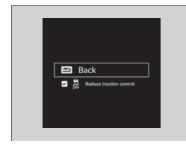
Roll the left selector wheel to scroll to select **Reduce traction control**, then press the left selector wheel to check or uncheck it.
