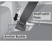
latch plate and anchor buckle. Make sure the seat belt is not twisted. Attach the belt to the anchor buckle.
