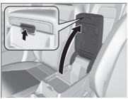
Pull the handle to open the console compartment.
