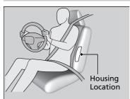
The side airbags are housed in the outside edge of the driver's, passenger's, and rear outer passenger's seat-backs.
