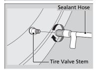
**3.** Attach the sealant hose onto the tire valve stem. Screw it until it is tight.
