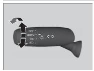
The lights will turn on automatically depending on the ambient brightness. They can also be switched on and off manually.
