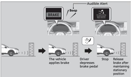
If only the rear parking sensors are turned off, the assistive braking will not work when reversing.
