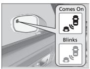
Blind spot information system alert indicator: Located on the outside door mirror on both sides.
