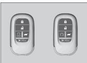
Use the keys to turn on and off the power system, lock and unlock all the doors, tailgate, and fuel fill door.
