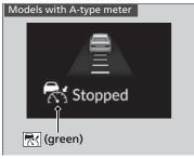
Your vehicle also stops automatically. The **Stopped** message appears on the gauge. When the vehicle ahead of you starts again, if you press the **RES/+/SET/-** switch up or down, or depress the accelerator pedal, ACC with Low Speed Follow will operate again within the previously set speed.
