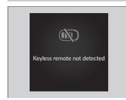
When the power mode is set to any mode other than OFF and you remove the keyless remote from the vehicle and shut the door, an alarm will sound. If the alarm continues to sound, place the keyless remote in another location.
