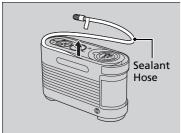
2. Remove the sealant hose from the kit.
