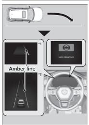
The front camera behind the rearview mirror monitors left and right lane markings in white or yellow, the outer edge of the pavement (bordered by grass or gravel road shoulder) or a detected oncoming vehicle.
