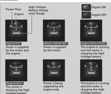
▶ Power Flow/Engine Status Display/High Voltage Battery Charge Level Gauge
