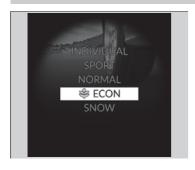
Facilitates fuel-efficient driving.
