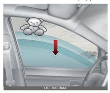
If the upward movement of the window is blocked by an object or part of the body, the window will detect the resistance and will stop upward movement. The window will then lower approximately 30 cm (11.8 inches) to allow the object to be cleared.
