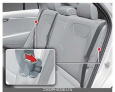
Pull on the seatback folding lever, then fold the seat toward the front of the vehicle.
