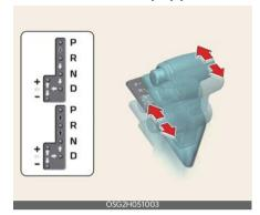
Depress the brake pedal and press the shift button while moving the shift lever.
