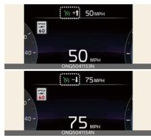
If the speed limit of the road changes during the operation of Manual Speed Limit Assist or Smart Cruise Control, an arrow in the direction of up or down is displayed to inform the driver that the set speed needs to be changed. At this time, the driver can change the set speed according to the speed limit by using the (+) or (-) switch on the steering wheel.
