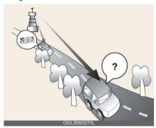
Flutter/Static - Weak FM signals or large obstructions between the transmitter and your radio can disturb the signal causing static or fluttering noises to occur. Reducing the treble level may lessen this effect until the disturbance clears.  Station Swapping - As an FM signal weakens, another more powerful signal near the same frequency may begin to play. This is because your radio is designed to lock onto the clearest signal. If this occurs, select another station with a stronger signal.
