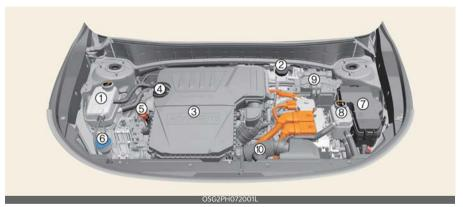
\* The actual engine room in the vehicle may differ from the illustration. 1. Engine coolant reservoir 9-17 2. Brake fluid reservoir 9-21 3. Air cleaner 9-13 4. Engine oil filler cap 9-15 5. Engine oil dipstick 9-15 6. Windshield washer fluid reservoir 9-23 7. Fuse box 9-40 8. Inverter coolant reservoir 9-18 9. Electric Control Unit (ECU) 8-5 9-22 10.Engine actuator reservoir tank
