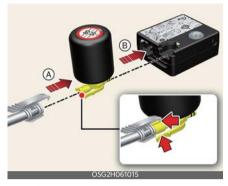
Make sure the compressor valve on the filling hose is locked.
