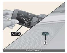
When the light switch is in the AUTO light position, the taillamps and head-lamps will turn ON or OFF automatically depending on the amount of light outside the vehicle.
