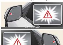
The warning light on the outside rear view mirror (side view mirror) and head-up display (if equipped) will appear when the vehicle on both lanes is detected from the rear.
