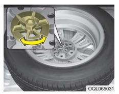
Turn the tire hold-down wing bolt counterclockwise.
