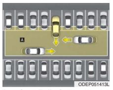
Rear Cross-Traffic Collision Warning uses radar sensors to monitor the approaching cross traffic from the left and right side of the vehicle when your vehicle is in reverse.
