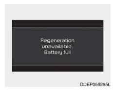
If SOC(State of High voltage battery Charge) is high, it is not possible to enable Regen B mode. Use the function again after normal driving.
