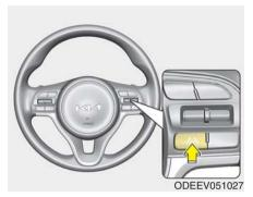
Lane Following Assist status is remembered by the function and therefore does not need to be enabled again for each new journey. Once the function starts working, the indicator light ((a)) comes on the instrument panel.
