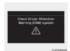
When the "Check Driver Attention Warning (DAW) system" warning message appears, the function is not working properly. If this occurs, have the system checked by an authorized Kia dealer.
