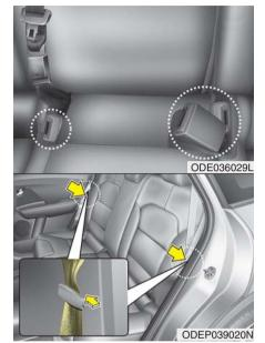
3. When folding the seat back, insert the rear seat belt buckle in the pocket between the rear seatback and cushion then make sure both seatbelts do not interfere with stowed luggage and cargo. Then insert the seat belt into the two webbing guide (or holder) located on both sides.
