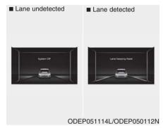
If the speed of the vehicle is over 60 km/h (40 mph) and the function detects lane markers, the color changes from gray to white.
