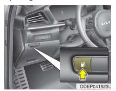
The fuel filler door must be opened from inside the vehicle by pushing the fuel filler door button.
