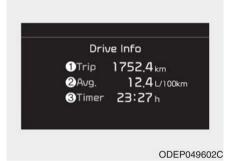
This display shows the trip distance (1), the average fuel efficiency (2), and the total driving time (3) information once per one ignition cycle.
