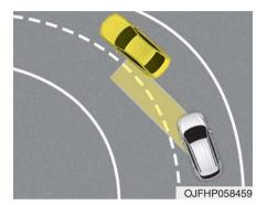
Blind-Spot Collision Warning may not operate properly when driving on a curved road. In certain instances the function may recognize a vehicle in the same lane.
