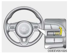
If any method other than the Driving Assist button was used to cancel cruising speed and the function is still activated, the cruising speed will automatically resume when you move the switch up (to RES+).
