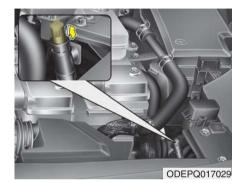
If the charging connector does not unlock for some reason, open the hood and slightly pull the emergency cable as shown above. The charging door will then open.
