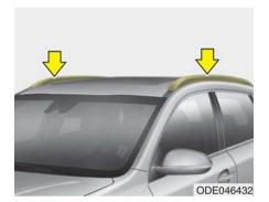
If the vehicle has a roof rack, you can load cargo on top of your vehicle.
