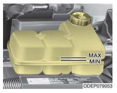
The coolant level should be filled between MAX and MIN marks on the side of the coolant reservoir when the engine is cool.
