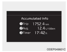
This display shows the accumulated trip distance (1), the average fuel efficiency (2), and the total driving time (3).
