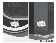
This warning light illuminates if the ignition switch or ENGINE START/STOP button is changed to the ON position and goes off in approximately 3 seconds if the system is operation normally.
