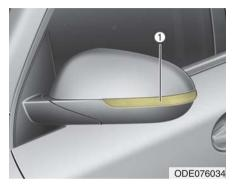
If the side repeater lamp (LED type) (1) does not operate, have the vehicle checked by an authorized Kia dealer.
