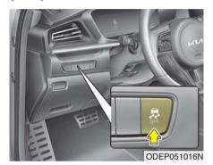
The Electronic Stability Control (ESC) system is designed to stabilize the vehicle during cornering maneuvers. ESC checks where you are steering and where the vehicle is actually going. ESC applies the brakes on individual wheels and intervenes with the engine management system to stabilize the vehicle. Electronic stability control (ESC) will not prevent accidents. Excessive speed in turns, abrupt maneuvers and hydroplaning on wet surfaces can still result in serious accidents.
