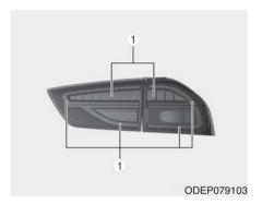
If the stop and tail lamp (LED type) (1) does not operate, have the vehicle checked by an authorized Kia dealer.
