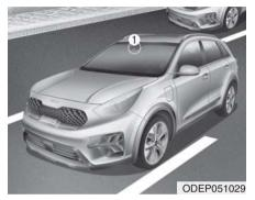
Front view camera (1) is a sensor for detecting lanes and the front vehicles.
