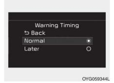
The driver can select the initial warning activation time on the LCD display.
