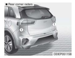
The rear corner radars (1) are the sensors inside the rear bumper for detecting the side/rear areas. Always keep the rear bumper clean for proper operation of the function.
