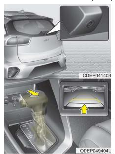
Rear View Monitor will activate with the ignition switch ON and the shift lever in the R (Reverse) position.
