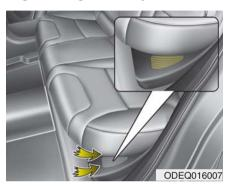
The hybrid battery air intake is located on bottom and side of the rear seats. The air intake cools down the hybrid battery. When the hybrid battery air intake is blocked, the hybrid battery may be overheated. Do not obstruct the air intake with any other objects.
