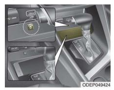
A wireless smart phone charging system is located in front of the center console
