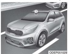
Lane Keeping Assist detects the lane markers on the road with a front view camera (1) at the front windshield, and assists the driver's steering to help keep the vehicle in the lanes. When the function detects the vehicle straying from its lane, it warns the driver with a visual and audible warning, while applying a slight countersteering torque, trying to prevent the vehicle from moving out of its lane.
