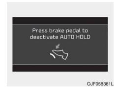
If you did not apply the brake pedal when you release the Auto Hold by pressing the [AUTO HOLD] switch, a warning will sound and a message will appear.
