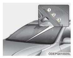
When charging the high voltage battery, the charge level can be checked from outside the vehicle.
