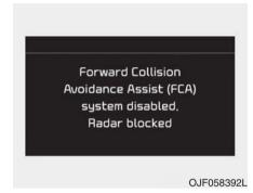
If the sensor or sensor cover is covered by bad weather or foreign objects, dust, etc., v operation may temporarily stop. In this case, the warning message appears to warn the driver.
