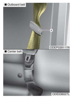
If the center seat belt is not in use, always lock the latch plate into the buckle as above illustration
