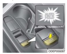
With the driver's door, engine hood closed, fasten the driver's seat belt or depress the brake pedal and then press the Auto Hold button. The white AUTO HOLD indicator will come on and the system will be in the standby position.
