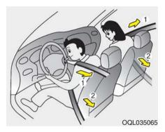
Your vehicle is equipped with driver's and front passenger's pre-tensioner seat belts (retractor pe-tensioner and EFD (Emergency Fastening Device)). The pre-tensioner seat belts may be activated, when a frontal collision is severe enough, together with the air bags.
