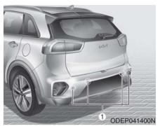
Reverse Parking Distance Warning assists the driver during backward movement of the vehicle by chiming if any object is sensed within a distance of 120 cm (48 in) behind the vehicle.
