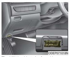
The VIN is able to be found by a professional diagnostic equipment from the ECU. The diagnostic equipment is connected to OBD connector on the inner fuse panel. For more information, we recommend that you contact an authorized Kia dealer.
