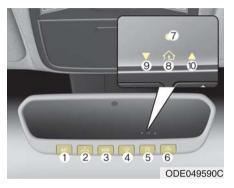
Your vehicle may be equipped with a Gentex Automatic-Dimming Mirror and an Integrated HomeLink® Wireless Control System.
