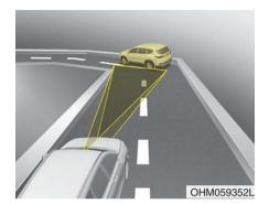
Your vehicle speed can be reduced due to a vehicle in the adjacent lane. Adjust your vehicle speed by depressing the brake pedal according to the road condition ahead and driving condition. Apply the accelerator pedal and select the appropriate set speed. Check to be sure that the road conditions permit safe operation of Smart Cruise Control.
