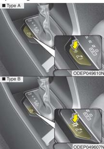
Press the Parking Distance Warning Off button to turn off the Reverse Parking Distance Warning. The indicator light on the button will turn on.
