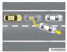
• When vehicles are at a standstill and the vehicle in front of you changes to the next lane, be careful when your vehicle starts to move because it may not recognize the stopped vehicle in front of you. In this case, you must maintain a safe braking distance, and if necessary, depress the brake pedal to reduce your driving speed in order to maintain a safe distance.
