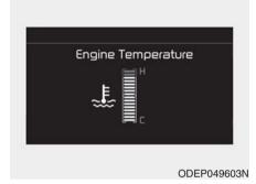
This gauge indicates the temperature of the engine coolant when the engine is running.
