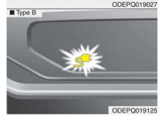
Check if the charging cable connection indicator of the high voltage battery in the instrument cluster is turned ON. Charging does not occur when the indicator is OFF. When the charging connector is not connected properly, reconnect the charging cable to charge.
