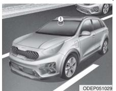
Lane Following Assist is designed to center the vehicle in the chosen lane by using a front view camera (1) on top of the windshield.
