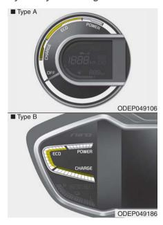
The hybrid system gauge indicates whether the current driving condition is fuel efficient or not
