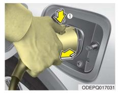
While holding the charging connector, pressing the locking release button (1) and then pull it out. To prevent charging cable theft, the charging connector cannot be disconnected from the inlet when the doors are locked. Unlock all doors to disconnect the charging connector from the inlet.
