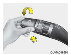
High Beam Assist is a function that automatically adjusts the headlamp range (switches between high beam and low beam) according to the brightness of other vehicles and road conditions.
