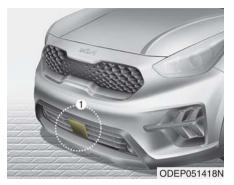
Front radar (1) detects the distance to the vehicle ahead.
