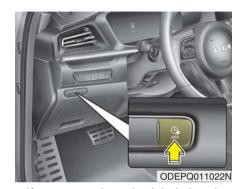
If you press the scheduled charging deactivation (9) button to immediately charge the battery, charging must be initiated 3 minutes after the charging cable has been connected. When you press the scheduled charging deactivation ( b) button for immediate charging, the scheduled charge setting is not completely deactivated. If you need to completely deactivate the scheduled charge setting, use the Infotainment System to finalize the deactivation
