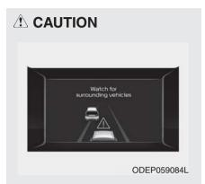
If the vehicle ahead (vehicle speed: less than 30 km/h (20 mph) disappears to the next lane, the warning chime will sound and a message will appear. Adjust your vehicle speed for vehicles or objects that can suddenly appear in front of you by depressing the brake pedal according to the road condition ahead and driving condition.
