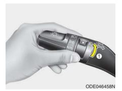
Fog lights are designed to provide improved visibility when visibility is poor due to fog, rain or snow, etc. The fog lights will turn on when the fog light switch (1) is turned to the on position after the headlight is turned on.
