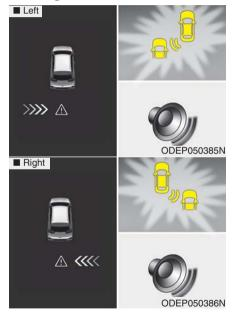
If the vehicle detected by the sensors approaches from the rear left/right side of your vehicle, the warning chime will sound, the warning light on the outside rearview mirror will blink and a message will appear on the LCD display. If the rear view camera function is in activation, a message will also appear on the 'Infortainment System'.
