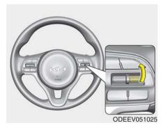
If any method other than the Driving Assist button was used to cancel cruising speed and the function is still activated, the most recent set speed will automatically resume when the RES+ switch is pushed.
