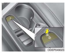
With the ignition switch or ENGINE START/STOP button is ON position, pressing the heated steering wheel button warms the steering wheel. The indicator on the button will illuminate.
