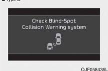
If there is a problem with Blind-Spot Collision Warning, a warning message will appear and the light on the switch will turn off. The function will turn off automatically.
