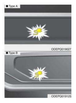
Check if the charging cable connection indicator of the high voltage battery in the instrument cluster is turned ON
