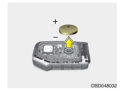
The transmitter uses a 3 volt lithium battery which will normally last for several years. When replacement is necessary, use the following procedure.
