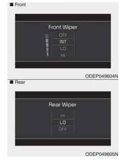
This indicator displays which wiper speed is selected using the wiper control.
