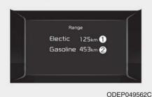
The range is the estimated distance the vehicle can be driven with the remaining high-voltage (hybrid) battery (1, Electric) and fuel in the fuel tank (2, Gasoline).
