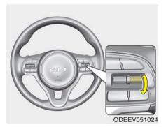
Push the switch down (to SET-), and release it at the desired speed. The cruise set indicator light will illuminate. Release the accelerator pedal at the same time. The desired speed will automatically be maintained.
