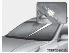
When scheduled charging is set and the AC Charger or the portable charging cable (ICCB: In-Cable Control Box) is connected for charging, the indicator lamp blinks (for 3 minutes) to indicate that scheduled charging is set.
