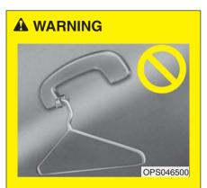
Do not hang other objects such as hangers or hard objects from the clothes hanger. Also, do not put heavy, sharp or breakable objects in the clothing's pockets. In an accident or when the curtain air bag is inflated, it may cause vehicle damage or personal injury.
