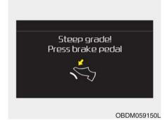
This warning message is displayed when the vehicle is driven slowly on a grade and the vehicle detects that the brake pedal is not applied.
