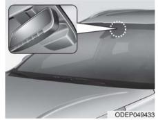
Auto defogging reduces the probability of fogging up the inside of the windshield by automatically sensing the moisture of inside the windshield.
