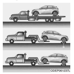
If emergency towing is necessary, we recommend having it done by an authorized Kia dealer or a commercial tow-truck service. Proper lifting and towing procedures are necessary to prevent damage to the vehicle. The use of wheel dollies (1) or flathed is recommended
