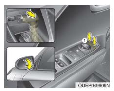
When you shift the shift lever to the R (Reverse) position, the outside rearview mirror(s) will move downward to aid reverse parking. According to the position of the outside rearview mirror switch (1), the outside rearview mirror(s) will operate as follows:
