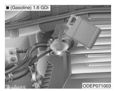
Use a funnel to help prevent oil from being spilled on engine components.
