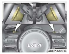
The paddle shift function is available when the shift lever is in the sport/manual mode.
