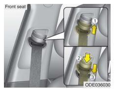
Height adjustment (For Front seat) You can adjust the height of the shoulder belt anchor to one of the 4 positions for maximum comfort and safety.
