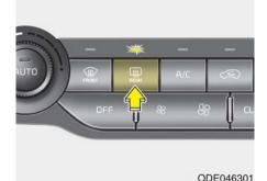
The defroster heats the window to remove frost, fog and thin ice from the rear window, while the engine is running.
