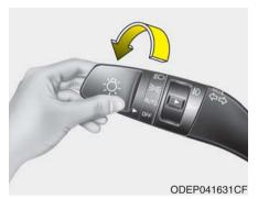
The parking lamp and headlamp will be turned ON or OFF automatically depending on the amount of daylight as measured by the ambient light sensor on the center dash when the parking brake is not engaged.
