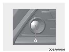
If the front fog lamp (Bulb/LED type) (1) does not operate, have the vehicle checked by an authorized Kia dealer.
