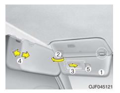
Use the sun visor to shield direct light through the front or side windows.
