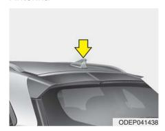
The roof antenna transmits and receives wireless signals such as AM/FM, Sirius XM, GNSS, etc.
