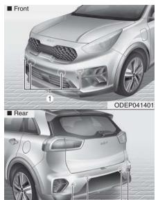
[1] : Front ultrasonic sensors[2] : Rear ultrasonic sensors
