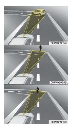
Forward Collision-Avoidance Assist may recognize a vehicle or pedestrian or cyclist in the next lane or outside the lane when driving on a curved road.
