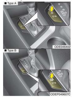
This function activates when Parking Safety button is pressed with the ignition switch ON.
