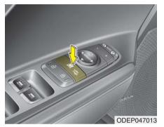
The driver can disable the power window switches on the rear passenger doors by pressing the power window lock button located on the driver's door to the LOCK position (pressed).
