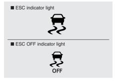
When ignition switch or the ENGINE START/STOP button is turned to ON, the indicator light illuminates, then goes off if the ESC system is operating normally.
