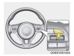
Press the Driving Assist button. (the CRUISE indicator in the instrument cluster will go off).
