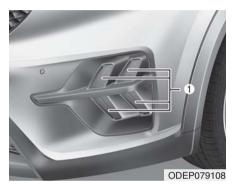
If the daytime running lamp/position lamp (LED type) (1) does not operate, have the vehicle checked by an authorized Kia dealer
