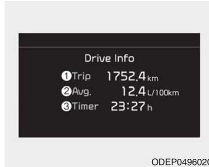
This display shows the trip distance (1), the average fuel efficiency (2), and the total driving time (3) information once per one ignition cycle.
