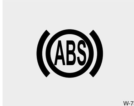
The ABS warning light will stay on for approximately 3 seconds after the ignition switch or the ENGINE START/STOP button is ON. During that time, the ABS will go through self-diagnosis and the light will go off if everything is normal. If the light stays on, you may have a problem with your ABS. Contact an authorized Kia dealer as soon as possible.
