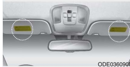
Air bag warning labels, some required by the Canada Motor Vehicle Safety Standards (CMVSS), are attached to the sunvisor to alert the driver and passengers of potential risks of the air bag system.
