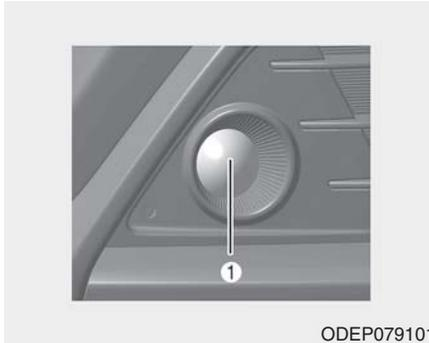
If the front fog lamp (Bulb/LED type) (1) does not operate, have the vehicle checked by an authorized Kia dealer.
