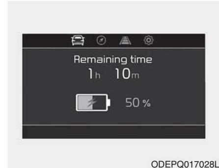
11. After charging has started, the estimated charging time is displayed on the instrument cluster for about 1 minute. It is also displayed, when the driver's door is opened with charging in progress. When scheduled charging is set, the estimated charging time is displayed as "--".
