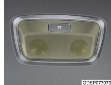
If the room lamp (LED type) (1) does not operate, have the vehicle checked by an authorized Kia dealer. The LED lamp cannot be replaced as a single component because it is an integrated unit. The LED lamp has to be replaced with the unit.
