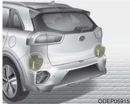
The rear radars are located inside the rear bumper for detecting the side and rear areas.
