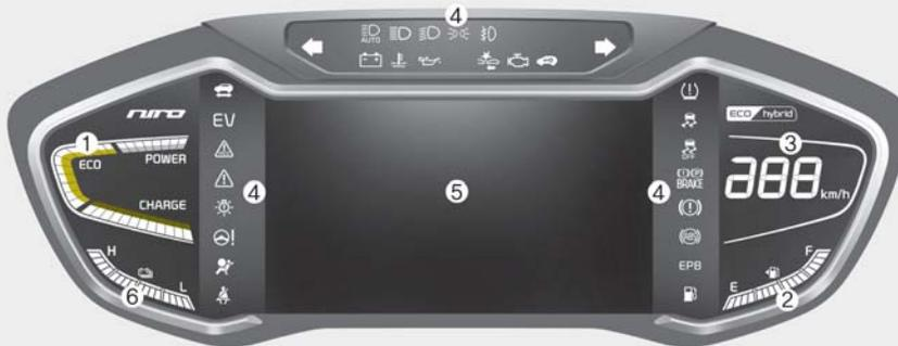
6. Battery SOC (State of Charge) gauge
