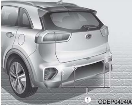
Reverse Parking Distance Warning system assists the driver during backward movement of the vehicle by chiming if any object is sensed within a distance of 48 in (120 cm) behind the vehicle.
