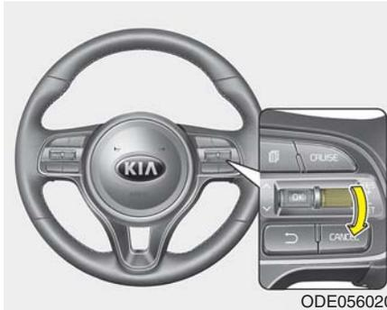
3. Move the switch down (to SET-), and release it at the desired speed. The cruise set indicator light will illuminate. Release the accelerator pedal at the same time. The desired speed will automatically be maintained.
