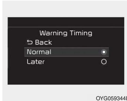
The driver can select the initial warning activation time in the Cluster by selecting “User Settings → Driver Assistance → Warning Timing”. The options for the initial Rear Cross-Traffic Collision Warning includes the following:
