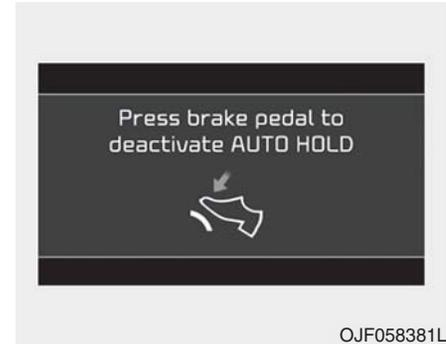
If you did not apply the brake pedal when you release the Auto Hold by pressing the [AUTO HOLD] switch, a warning will sound and a message will appear.
