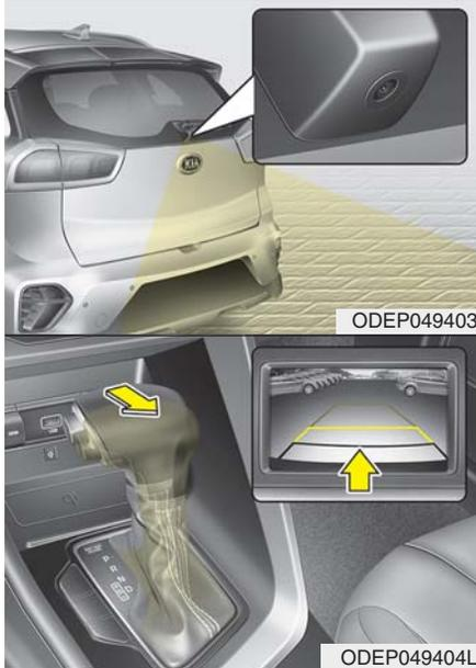
Rear View Monitor system will activate with the ignition switch ON and the shift lever in the R (Reverse) position.
