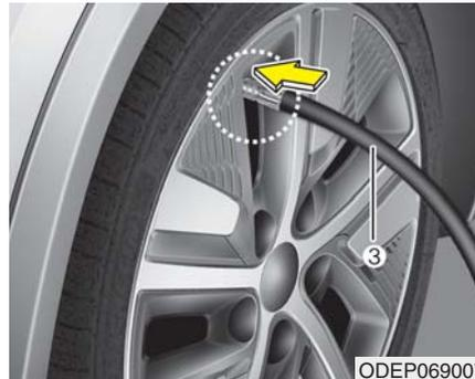
4. Unscrew the valve cap from the valve of the defective wheel and screw filling hose (3) of the sealant bottle onto the valve.
