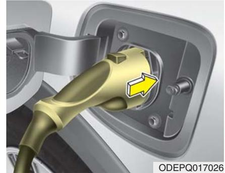
5. Remove any dust on the charging connector and charging inlet.
