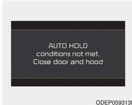
When you press the [AUTO HOLD] switch, if the driver's door, engine hood are not closed, a warning will sound and a message will appear on the LCD display. At this moment, press the [AUTO HOLD] button after closing the driver's door and hood.
