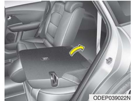
5. To use the rear seat, lift and pull the seatback backward by lifting up seat back. Pull the seatback firmly until it clicks into place. Make sure the seatback is locked in place.
