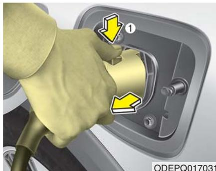
2. While holding the charging connector, pressing the locking release button(1) and then pull it out.
