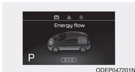
This mode means the vehicle is at a stop. (There is no energy flow.)
