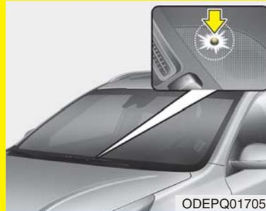
**The Aux. Battery Saver+ relies on the high voltage battery to charge the 12V battery. The charging indicator lamp will blink rapidly when this is occurring. To reduce the risk of electrical shock, do not touch any high voltage components (orange-colored) or other electrical devices while charging is occurring.**
