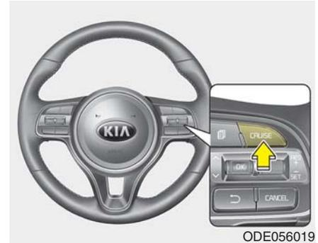
1. Press the CRUISE button on the steering wheel, to turn the system on. The cruise indicator light will illuminate.
