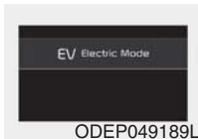
: The high-voltage (hybrid) battery is used to drive the vehicle.
