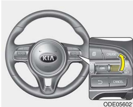
If any method other than the CRUISE button was used to cancel cruising speed and the system is still activated, the most recent set speed will automatically resume when the RES+ switch is pushed.
