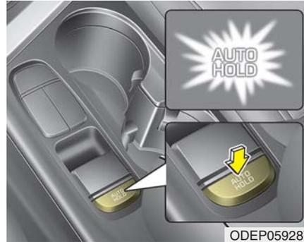
1. With the driver's door, engine hood closed, fasten the driver's seat belt or depress the brake pedal and then press the Auto Hold button. The white AUTO HOLD indicator will come on and the system will be in the standby position.
