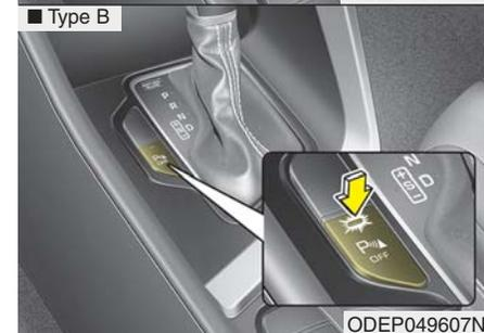
Push the button to turn off the Parking Distance Warning (Reverse) system. The indicator light on the button will turn on.
