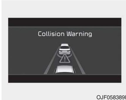
If there is a high risk of collision due to sudden braking of the front vehicle or lack of safety distance with the vehicle ahead during SCC driving, so that if the driver's brake or steering wheel operation is required, the Distance Step with the vehicle ahead will blink on the cluster and a collision warning will sound.
