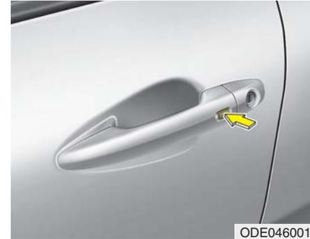
With a smart key, you can lock or unlock a door (and liftgate) and start the engine.
