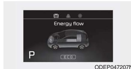
The engine and regenerative braking system charge the hybrid battery driving deceleration.
