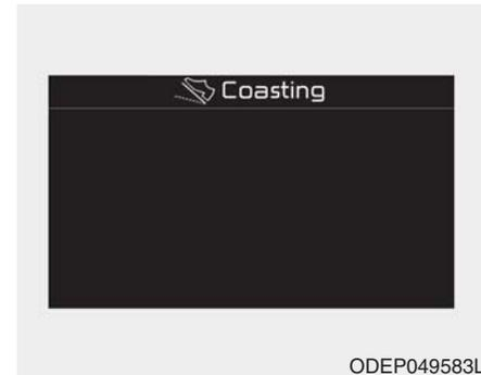
A chime will sound and the coasting guide indicator will blink four times to inform the driver when to take the foot off the accelerator by anticipating a decelerating event\* based on an analysis of driving routes and road conditions based on the navigation. It encourages the driver to remove foot from the pedal and allow coasting down the road with EV motor only. This helps prevent unnecessary fuel consumption and may increase fuel efficiency.
