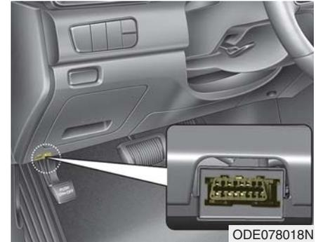
The VIN is able to be found by a professional diagnostic equipment from the ECU. The diagnostic equipment is connected to OBD connector on the inner fuse panel. For more information, we recommend that you contact an authorized Kia dealer.
