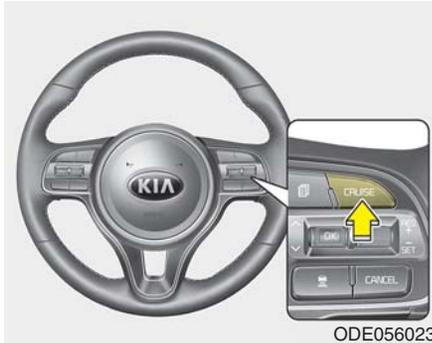
1. Press the CRUISE button, to turn the system on. The Cruise indicator (Ⓢ CRUISE) in the instrument cluster will illuminate.
