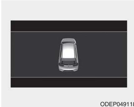
The warning message will appear on the LCD display when hood is open. The warning chime will operate when the vehicle is being driven at or above 3 km/h (2 mph) with the hood open.
