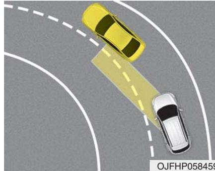
BCW system may not operate properly when driving on a curved road. In certain instances the system may recognize a vehicle in the same lane. Always pay attention to road and driving conditions, while driving.
