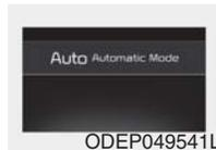
: The drive mode will be automatically selected from either Electric (CD) mode or Hybrid (CS) mode by the system according to the driving condition.
