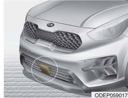
Front radar detects the distance to the vehicle ahead.
