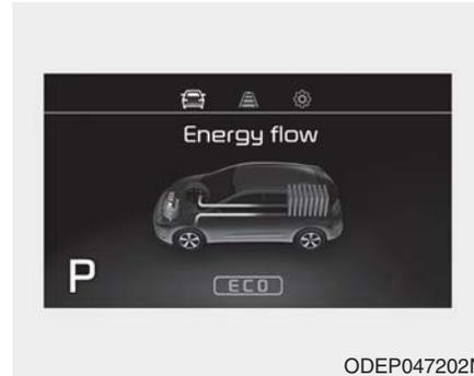
The hybrid system informs the driver its energy flow in various operating modes. While driving, the current energy flow is specified in 11 modes.
