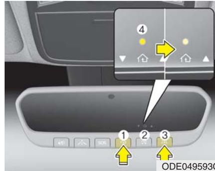
1. Press and hold the button (1) and (3) simultaneously.
