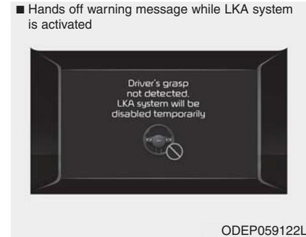
If the driver takes hands off the steering wheel for several seconds while LKA system is activated, the system will warn the driver.
