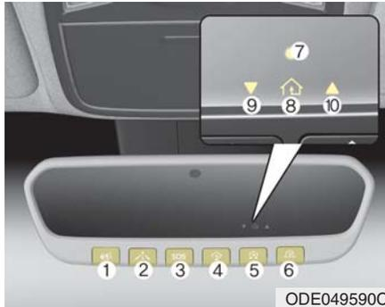
Your vehicle may be equipped with a Gentex Automatic-Dimming Mirror and an Integrated HomeLink® Wireless Control System.
