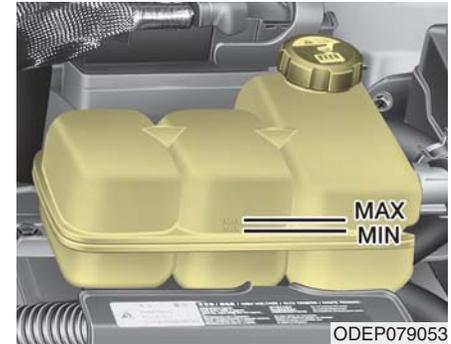
The coolant level should be filled between MAX and MIN marks on the side of the coolant reservoir when the engine is cool.
