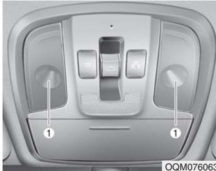
If the map lamp (LED type) (1) does not operate, have the vehicle checked by an authorized Kia dealer. The LED lamp cannot be replaced as a single component because it is an integrated unit. The LED lamp has to be replaced with the unit.
