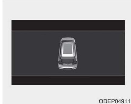
If the driver removes the ignition key (smart key: turns off the engine) when the sunroof is not fully closed, the warning chime will sound for a few seconds and a warning image will appear on the LCD display.
