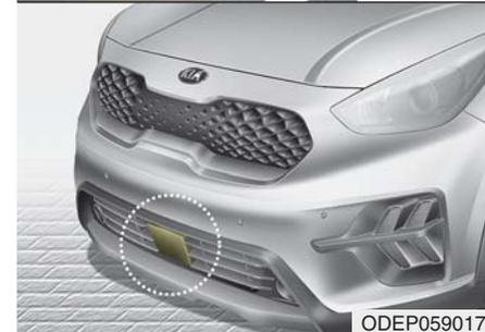
The sensors are that detecting the distance to vehicles ahead, pedestrian or cyclist.
