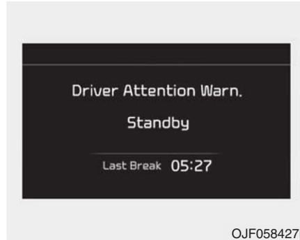
Driver Attention Warning system enters the ready status and displays the 'Standby' screen in the following situations.
