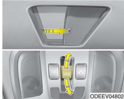
To open or close the sunroof (manual slide feature), push the sunroof control lever backward or forward to the first detent position.
