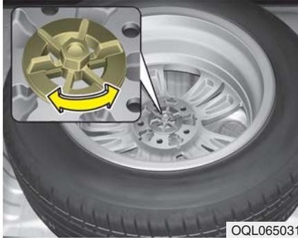
Turn the tire hold-down wing bolt counterclockwise.
