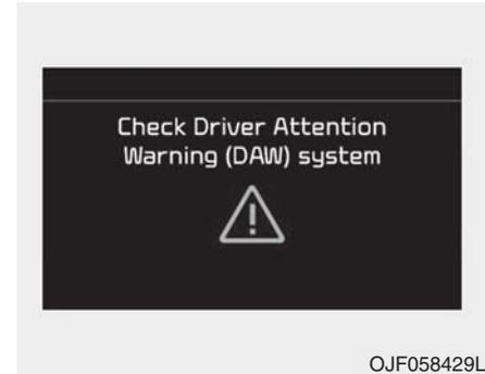
When the "Check Driver Attention Warning (DAW) system" warning message appears, the system is not working properly. If this occurs, have the system checked by an authorized Kia dealer.
