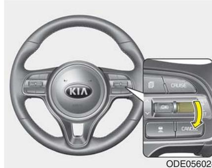
3. Move the switch down (to SET-), and release it at the desired speed. The set speed and vehicle to vehicle distance on the LCD screen will illuminate.
