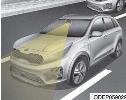
Lane Following Assist system is designed to center the vehicle in the chosen lane by using a front mounted camera on top of the windshield.
