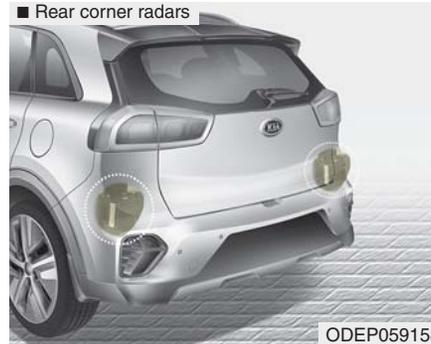
The rear corner radars are the sensors inside the rear bumper for detecting the side/rear areas. Always keep the rear bumper clean for proper operation of the system.
