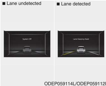
If the speed of the vehicle is over 60 km/h (40 mph) and the system detects lane markers, the color changes from gray to white.
