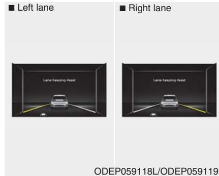
If the vehicle leaves a lane, the lane marker you cross will blink on the LCD display and the warning sound is provided.
