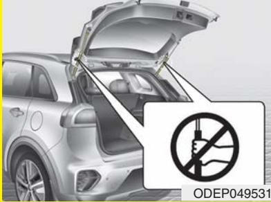
**Do not grasp the part supporting the liftgate (gas lifter), as this may cause serious injury.**
