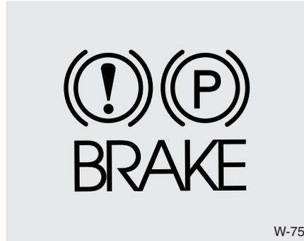
Check the brake warning light by turning the ignition switch or ENGINE START/STOP button ON (do not start the engine). This light will be illuminated when the parking brake is applied with the Ignition switch or ENGINE START/STOP button in the START or ON position.
