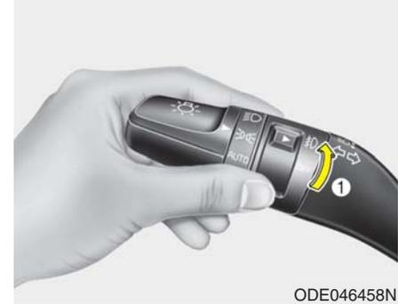
Fog lights are designed to provide improved visibility when visibility is poor due to fog, rain or snow, etc. The fog lights will turn on when the fog light switch (1) is turned to the on position after the headlight is turned on.
