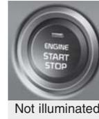
To turn off the engine (START/RUN position) or vehicle power (ON position), press the ENGINE START/STOP button with the shift lever in the P (Park) position. When you press the ENGINE START/STOP button without the shift lever in the P (Park) position, the ENGINE START/STOP button will not change to the OFF position but to the ACC position.
