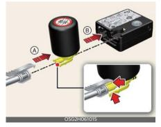
Make sure the compressor valve on the filling hose is locked.
