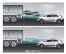
In the following cases, among other circumstances, the vehicle in front cannot be detected by the sensor. Always pay attention to the road and driving conditions and drive safely. If necessary, adjust your vehicle speed.
