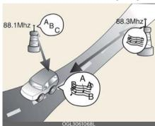
Multi-Path Cancellation - Radio signals being received from several directions can cause distortion or fluttering. This can be caused by a direct and reflected signal from the same station, or by signals from two stations with close frequencies. If this occurs, select another station until the condition has passed. ing. These should never be used during the operation of the vehicle.
