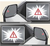
The warning light on the outside rear view mirror and head-up display (if equipped) will appear when a vehicle is detected from the rear.
