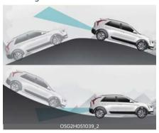
Blind-Spot Collision-Avoidance Assist may not operate properly when driving on a slope. The function may not detect the vehicle in the next lane or may incorrectly detect the ground or structure.
