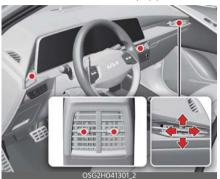
The outlet vents can be opened or closed by moving the vent left or right. Also, you can adjust the direction of air delivery from these vents using the vent control lever as shown.
