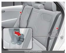
4. Pull on the seatback folding lever, then fold the seat toward the front of the vehicle.
