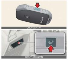
When the liftgate is closed, press the power liftgate open/close button for 1 second. The power liftgate opens with a warning sound.
