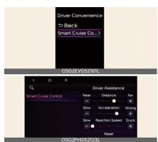
With the vehicle on, touch Settings → Driver Assistance → Driving Convenience → Smart Cruise Control on the instrument cluster or Settings → Vehicle → Driver Assistance → Driving Convenience → Smart Cruise Control on the infotainment system to set the distance, acceleration and the reaction speed.
