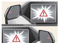
The warning light on the outside rear view mirror and head-up display (if equipped) will appear when the vehicle on both lanes is detected from the rear. A vehicle is detected in the following conditions.
