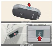
When the liftgate is closed, press the power liftgate open/close button for 1 second. The power liftgate opens. While the liftgate is opening, press the button to stop liftgate operation.
