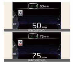
If the speed limit of the road changes during the operation of Manual Speed Limit Assist or Smart Cruise Control, an arrow in the direction of up or down is displayed to inform the driver that the set speed needs to be changed. At this time, the driver can change the set speed according to the speed limit by using the (+) or (-) switch on the steering wheel.
