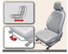
Adjust the seat before driving, and make sure the seat is locked securely by trying to move forward and backward without using the lever. If the seat moves, it is not locked properly.
