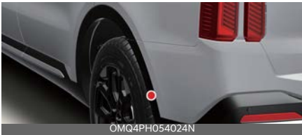
Rear side ultrasonic sensors
