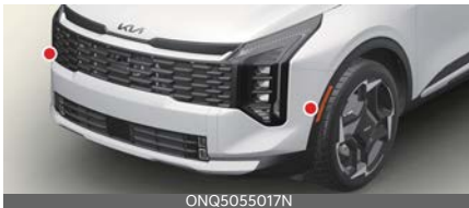
Front corner radar (if equipped)
