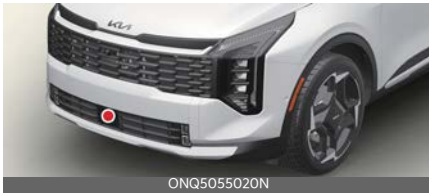
Front corner radar (if equipped)
