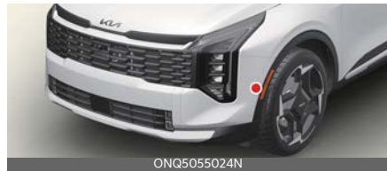
Front side ultrasonic sensors (if equipped)
