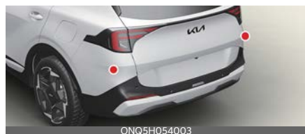
Rear corner radar (if equipped)
