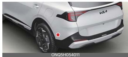
Rear side ultrasonic sensors (if equipped)
