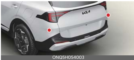
Rear corner radar (if equipped)
