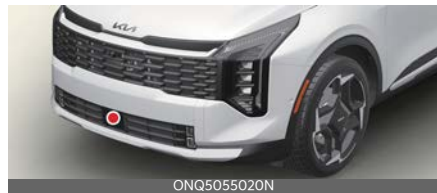
Front corner radar (if equipped)
