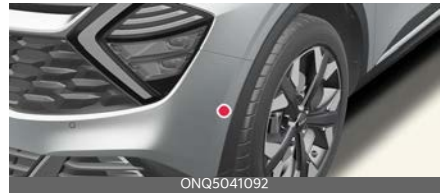
Rear side ultrasonic sensors
