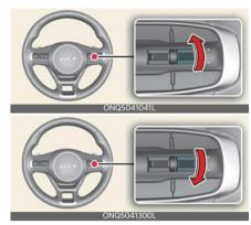
The set speed limit (1) will be displayed on the cluster. If you would like to drive over the preset speed limit, depress the accelerator pedal beyond the pressure point to activate the kickdown mechanism.
