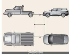
Use a towing cable or chain less than 16 feet (5 m) long. Attach a white or red cloth (about 12 inches (30 cm)
