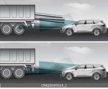
If the vehicle in front of you has cargo that extends beyond its bumper, or when the vehicle in front of you has an unusually high ground clearance, additional special attention is required. Forward Collision-Avoidance Assist may not be able to detect the cargo extending from the vehicle. Maintain a safe braking distance from the rearmost object. By steering, slowing, and braking as needed.
