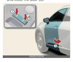
If you lock the door with the central door lock button (2), all vehicle doors will lock automatically.
