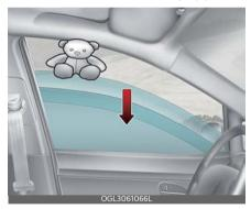
If the upward movement of the window is blocked by an object or part of the body, the window will detect the resistance and will stop upward movement. The window will then lower approximately 12 inches (30 cm) to allow the object to be cleared.
