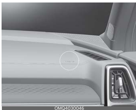
Passenger's front air bag
