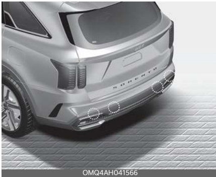
Rear ultrasonic sensors
