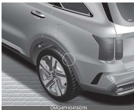
Rear corner ultrasonic sensors
