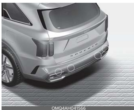
Rear ultrasonic sensors
