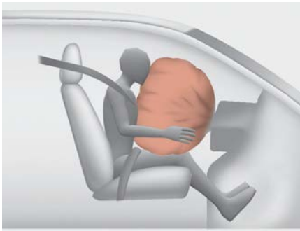
Passenger's front air bag
