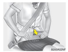
The seat belt automatically adjusts to the proper length only after the lap belt portion is adjusted manually so that it fits snugly around your hips. If you lean forward in a slow, easy motion, the belt will extend and let you move around. If there is a sudden stop or impact, however, the belt will lock into position. It will also lock if you try to lean forward too quickly.
