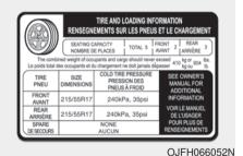
The label located on the driver's door sill gives the original tire size, cold tire pressures recommended for your vehicle, the number of people that can be in your vehicle and vehicle capacity weight.
