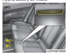
The hybrid battery air intake is located on bottom the rear seats. The air intake cools down the hybrid battery. When the hybrid battery air intake is blocked, the hybrid battery may be overheated. Do not obstruct the air intake with any other objects.
