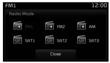
Pressing the **[RADIO]** button will change the operating mode in order of FM1 → FM2 → AM → SAT1 → SAT2 → SAT3
