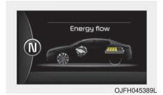
The mode means the vehicle at stop. (There is no energy flow.)
