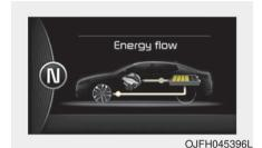
The engine and regenerative braking system charge the hybrid battery driving deceleration.
