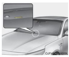
You can monitor the charging status outside of the vehicle when charging the high-voltage battery.
