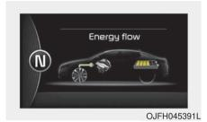
Engine power is used to move the vehicle. (Engine → Wheel)
