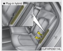
Do not put objects on the left side of rear seat. This could block the battery cooling duct causing battery degradation.
