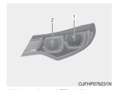
If the head lamp (LED) (1,2) does not operate, have the vehicle checked by an authorized Kia dealer. The LED lamps cannot be replaced as a single unit because it is an inte grated unit. The LED lamps has to be replaced with the unit. A skilled technician should check or repair the head lamp (LED), for it may damage related parts of the vehicle.
