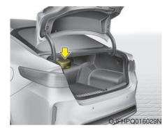
We recommend that the trickle charger cable should be put in a storage box after use. Keep the storage box above the main battery pack inside the trunk.
