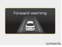
The warning message appears on the LCD display with the warning alarms.
