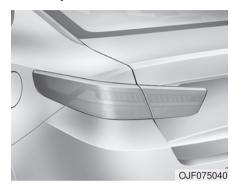
If the stop and tail lamp (LED) does not operate, have the vehicle checked by an authorized Kia dealer. The LED lamps cannot be replaced as a single unit because it is an integrated unit. The LED lamps has to be replaced with the unit. A skilled technician should check or repair the stop and tail lamp (LED), for it may damage related parts of the vehicle.
