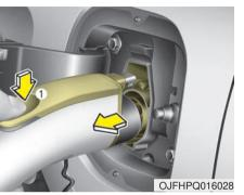
2. Hold the charging connector handle and pull it while pressing the release button(1).
