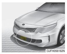
The sensor is to maintain a certain distance from the vehicle in front. However, the smudged sensor lens with foreign substances, such as snow and rain, adversely affects the sensing performance. It may even temporarily cancel the AEB. Always keep the sensor lens clean.
