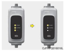
3. Check if all LED lamps on the control box blinks for 0.5 seconds. Then, check if the power lamp (green) turns ON.
