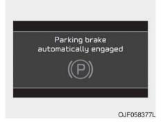
If the EPB is applied while Auto Hold is activated because of an ESC (Electronic Stability Control) signal, a warning will sound and a message will appear.
