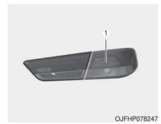
If the stop lamp (LED type) (1) does not operate, have the vehicle checked by an authorized Kia dealer. The LED lamps cannot be replaced as a single component because they are part of an integrated unit. The LED lamps have to be replaced with the unit. A skilled technician should check or repair the stop lamp (LED), to avoid damage to related parts of the vehicle.
