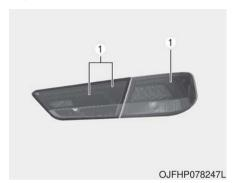
If the tail lamp (LED type) (1) does not operate, have the vehicle checked by an authorized Kia dealer. The LED lamps cannot be replaced as a single component because they are part of an integrated unit. The LED lamps have to be replaced with the unit. A skilled technician should check or repair the tail lamp (LED), to avoid damage to related parts of the vehicle
