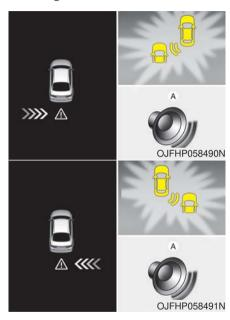
If the vehicle detected by the sensors approaches from the rear left/right side of your vehicle, the warning chime will sound, the warning light on the outside rearview mirror will blink and a message will appear on the LCD display.
