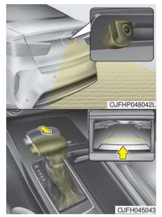
The rear view monitor will activate when the back-up light is ON with the ignition switch ON and the shift lever in the R (Reverse) position.
