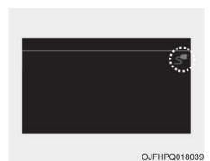
Check if the charging cable connection indicator of the high voltage battery in the instrument cluster is turned ON
