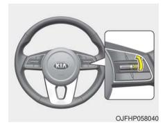
If any method other than the CRUISE ON-OFF switch was used to cancel cruising speed and the system is still activated, the most recent set speed will automatically resume when you move the lever up.
