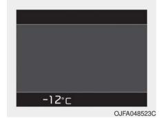
This gauge indicates the current outside air temperatures by 1°C (1°F).
