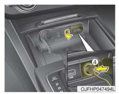
9. Connect between compressor and the vehicle power outlet using the cable and connectors (4).
