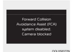
When the sensor is blocked with dirt, snow, or debris, the FCA system operation may stop temporarily.
