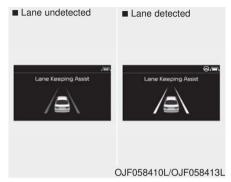
If the speed of the vehicle is over 60 km/h (37 mph) and the system detects lane markers, the color changes from gray to white
