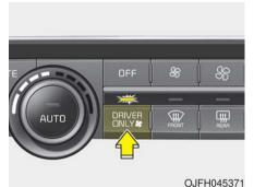
If you press the DRIVER ONLY button( ) and the indicator light illuminates, cold air mostly blows in the direction of the driver's seat. However, some of the cold air may come out of other seats' ducts to keep indoor air pleasant.
