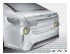
The sensors are located inside the rear bumper for detecting rear / side areas.
