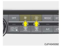
The fan speed can be set to the desired speed by operating the fan speed control button.
