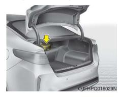
We recommend that the trickle charger cable be put in a storage box after use. Keep the storage box above the main battery pack inside the trunk.
