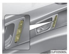
A driver position memory system is provided to store and recall the driver seat and outside rearview mirror position with a simple button operation. By saving the desired position into the system memory, different drivers can reposition the driver seat and outside rearview mirror based upon their driving preference. If the battery is disconnected, the desired seat position memory will need to be re-saved.
