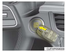
If the battery is weak or the smart key does not work correctly, you can start the hybrid system by pressing the engine start/stop button with the smart key.
