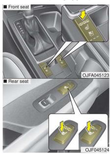
The seat warmer is provided to warm the front seats during cold weather. With the ignition switch in the ON position, push either of the switches to warm the driver's seat or the front passenger's seat.
