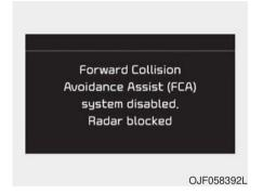
When the cover is covered with dirt, snow, or debris, the FCA system operation may not be able to detect vehicles.
