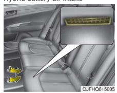
The hybrid battery air intake is located at the bottom the rear seats.
