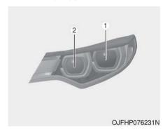
If the head lamp (Low (1), High (2)) does not operate, have the vehicle checked by an authorized Kia dealer. The LED lamps cannot be replaced as a single component because they are part of an integrated unit. The LED lamps have to be replaced with the unit. A skilled technician should check or repair the head lamp (LED), to avoid damage to related parts of the vehicle.
