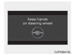
If the driver takes hands off the steering wheel for several seconds while the LKA is activated, the system will warn the driver.
