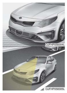
In order for the FCA system to operate properly, always make sure the sensor or sensor cover are clean and free of dirt, snow, and debris.
