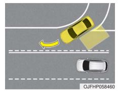
The BCW systems may not operate properly when driving on a curved road. In certain instances the system may recognize a vehicle in the same lane.
