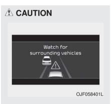
If the vehicle ahead (vehicle speed: less than 30 km/h (20 mph) disappears to the next lane, the warning chime will sound and a message will appear. Adjust your vehicle speed for vehicles or objects that can suddenly appear in front of you by depressing the brake pedal according to the road and driving conditions ahead.
