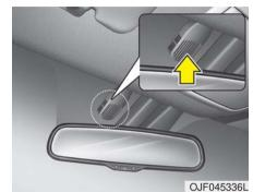
Auto defogging reduces the probability of fogging up the inside of the windshield by automatically sensing the moisture of inside the windshield. The auto defogging system operates when the heater or air conditioning is
