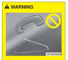
Do not hang other objects such as hangers or hard objects except clothes. Also, do not put heavy, sharp or breakable objects in the clothing's pockets. In an accident or when the curtain air bag is inflated, it may cause vehicle damage or personal injury.
