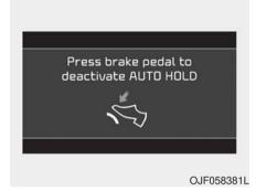
If you do not apply the brake pedal when you release the Auto Hold by pressing the [AUTO HOLD] switch, a warning will sound and a message will appear.
