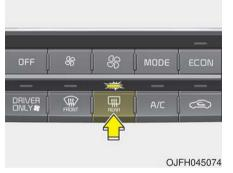
The defroster heats the window to remove frost, fog and thin ice from the rear window, while the engine is runnina.
