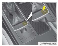
Pressing the HEV button changes the plug-in hybrid system modes, between Electric (Charge Depleting/CD) mode and Hybrid (Charge Sustaining/CS) mode.
