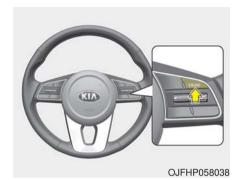
When the Smart Cruise Control System is not needed, press the [CRUISE] switch and deactivate the system.
