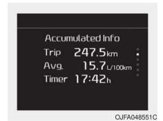
Displays accumulated information starting from mileage/fuel efficiency/time default point.
