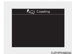
A chime will sound and the coasting guide indicator will blink four times to inform the driver when to take the foot off the accelerator by anticipating a decelerating event\* based on the analysis of driving routes and road conditions according to the navigation system. It encourages the driver to remove the foot from the pedal and allow coasting down the road with EV motor only. This helps preventing unnecessary fuel consumption and increases fuel efficiency.
