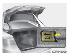
Your vehicle is equipped with an emergency trunk release lever located inside the trunk. Moving the handle in the direction of the arrow will release the trunk latch mechanism and open the trunk.
