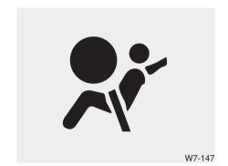
If the air bag warning light is illuminated for more than 6 seconds after engine start/stop button has been changed to ON, or of it illuminates during vehicle operation, an SRS component may not be functioning properly and you should have your
