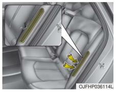
The high-voltage battery air intake is located on the left side of the rear seats. The air intake cools down the high-voltage battery.
