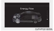
The vehicle is slowed down by engine compression.
