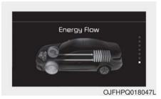
Hybrid battery is being charged by regenerative braking.
