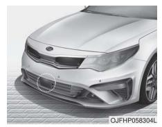
The sensor detects the distance to the vehicle ahead.
