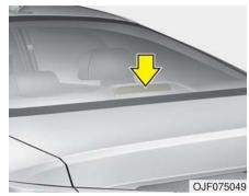
If the high mounted stop lamp (LED type) does not operate, have the vehicle checked by an authorized Kia dealer.
