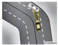
Your vehicle speed can be reduced due to a vehicle in the adjacent lane. Adjust your vehicle speed by depressing the brake pedal according to the road and driving conditions ahead. Apply the accelerator pedal and select the appropriate set speed. Check to be sure that the road conditions permit safe operation of the smart cruise control.
