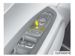
The driver can disable the power window switches on the passenger doors by pressing the power window lock button located on the driver's door to the LOCK position (pressed).
