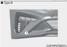
If the front fog lamp (Bulb and LED type) (1) does not operate, have the vehicle checked by an authorized Kia dealer.
