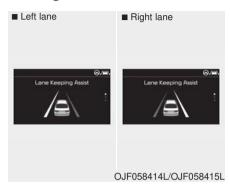
If the vehicle leaves a lane, the lane marker you cross will blink on the LCD display.
