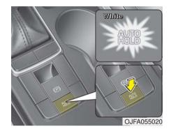
1.Depress the brake pedal, start the engine and then press the Auto Hold button. The white AUTO HOLD indicator will come on indicating the system is in standby. Before the Auto Hold will engage, the driver's door and engine hood must be closed and the driver's seat belt must be fastened.
