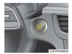
Whenever the front door is opened, the ENGINE START/STOP button will illuminate for your convenience. The light will go off after about 30 seconds when the door is closed.
