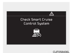
The message will appear when the vehicle to vehicle distance control system is not functioning normally.
