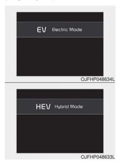
A corresponding message is displayed when a mode is selected by pressing the HEV button.
