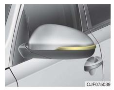
If the side repeater lamp (LED type) does not operate, have the vehicle checked by an authorized Kia dealer.
