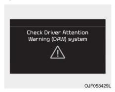
When the "Check Driver Attention Warning (DAW) system" warning message appears, the system is not working properly. In this case, take your vehicle to an authorized Kia dealer and have the system checked.
