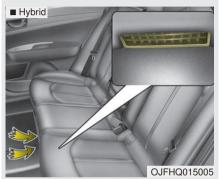
Do not put objects in the center lower part of rear seats. This could block the battery cooling duct causing battery degradation.
