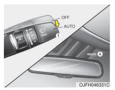
The rain sensor (A) located on the upper end of the windshield glass senses the amount of rainfall and controls the wiping cycle for the proper interval. The more it rains, the faster the wiper operates. When the rain stops, the wipers stop.
