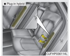
Do not put objects on the left side of rear seat. This could block the battery cooling duct causing battery degradation.
