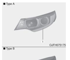
The LED lamps cannot be replaced as a single component because they are part of an integrated unit. The LED lamps have to be replaced with the unit.
