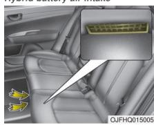
The hybrid battery air intake is located on the bottom of the rear seats. The air intake cools down the hybrid battery.
