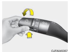
The High Beam Assist is a system that automatically adjusts the head-lamp range (switches between high beam and low beam) according to the brightness of other vehicles and road conditions.
