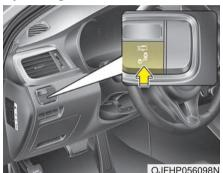
The indicator on the switch will illuminate when the BCW (Blind-Spot Collision Warning) system switch is pressed with the ignition switch ON. If the vehicle speed exceeds 30 km/h (20 mph), the system will activate.
