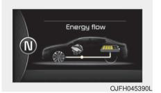
Electric power is used to move the vehicle. (Battery → Wheel)
