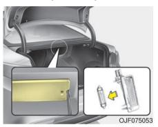
If the trunk lamp (LED) (1) does not operate, have the vehicle checked by an authorized Kia dealer.
