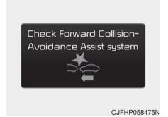
When the FCA is not working properly, the FCA warning light (>=>) will illuminate and the warning message will appear for a few seconds.
