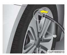
6. Unscrew the valve cap from the valve of the defective wheel and screw filling hose (3) of the sealant bottle onto the valve.
