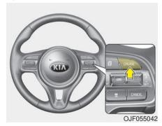
Press the CRUISE button, to turn the system on. The CRUISE indicator in the instrument cluster will illuminate. 2. Accelerate to the desired speed.
