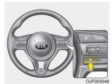
This function allows you to program the vehicle to maintain relative distance to the vehicle ahead without depressing the accelerator pedal or brake pedal.
