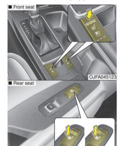
The seat warmer is provided to warm the front seats during cold weather. With the ignition switch in the ON position, push either of the switches to warm the driver's seat or the front passenger's seat.
