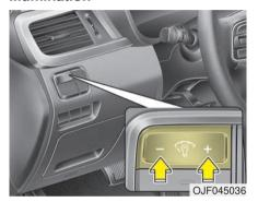
The brightness of the instrument panel illumination is changed by pressing the illumination control button ("+" or "-") when Engine Start/Stop button is ON, or the taillights are turned on.
