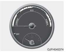
The hybrid system gauge indicates whether the current driving condition is fuel efficient or not.
