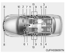
The SRS consists of the following components:
