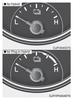
This gauge indicates the remaining hybrid battery power. If the SOC is near the "L (Low)" level, the vehicle automatically operates the engine to charge the battery.
