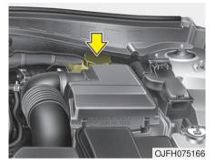
Check the fluid level in the reservoir periodically. The fluid level should be between MAX (Maximum) and MIN (Minimum) marks on the side of the reservoir.
