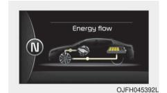
Electric and Engine power are used to move the vehicle.
