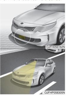
In order for the FCA system to operate properly, always make sure the sensor or sensor cover is clean and free of dirt, snow, and debris. Dirt, snow, or foreign substances on the sensor or its external parts may adversely affect the sensing performance of the sensor.
