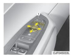
The electric remote control mirror switch allows you to adjust the position of the left and right outside rearview mirrors. To adjust the position of either mirror, press the R or L button (1) to select the right side mirror or the left side mirror, then press a corresponding point (▲) on the mirror adjustment control to position the selected mirror up, down, left or right. After adjustment, press the R or L button again to prevent the inadvertent adjustment.
