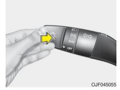
To turn on the high beam headlamp, push the lever away from you. The lever will return to its original position.
