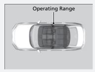
The engine may also start if the remote key is close to the door or window, even if it is outside the vehicle.
