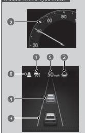
You can see the current state of Adaptive Cruise Control (ACC) with Low Speed Follow, Lane Keeping Assist System (LKAS) and Traffic Jam Assist.
