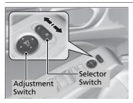
You can adjust the door mirrors when the power mode is in ON.
