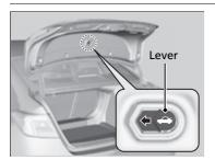
The trunk release lever allows you to open the trunk from inside for your safety.
