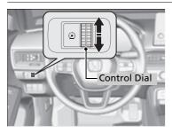
When the power mode is in ON, you can use the brightness control dial to adjust instrument panel brightness.
