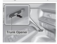
Press and hold the trunk opener on the driver's door to unlock and open the trunk.
