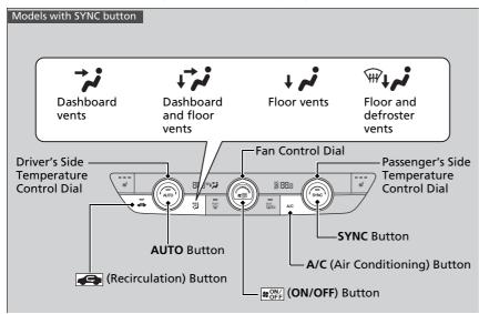
Use the system when the engine is running.
