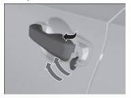
Insert the built-in key into the key cylinder from below the handle and then turn it.
