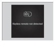
When the power mode is set to any mode other than OFF and you remove the remote key from the vehicle and shut the door, an alarm will sound. If the alarm continues to sound, place the remote key in another location.
