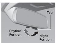
Flip the tab to switch the position. The night position will help to reduce the glare from headlights behind you when driving after dark.
