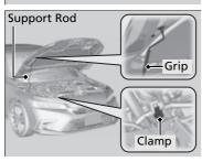
**4.** Remove the support rod from the clamp using the grip. Mount the support rod in the hood.
