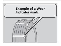
The groove where the wear indicator is located is about 1/16 inch (about 1.6 mm) shallower than elsewhere on the tire. If the tread has worn so that the indicator is exposed, replace the tire. **Worn out tires have poor traction on wet roads.**
