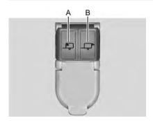
If equipped, trailering camera connectors are available in the bumper trailer receptacle in place of the four-pin connector. The inside trailer auxiliary camera should be installed on the top left hand side (A) and the rear trailer auxiliary camera (B) should be installed on the top right hand side.
