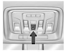
If equipped, the power sliding rear window works when the ignition has been turned on or to accessory mode, or Retained Accessory Power (RAP) must be active. See Retained Accessory Power (RAP) ⇒ 218.
