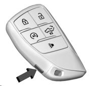
ress and release  $\bigcirc$ , then immediately press and hold  $\bigcirc$  until the turn signal lamps flash or for at least four seconds. The engine may be started from outside the vehicle using the remote key. See *Remote Start*  $\triangleright$  17.
