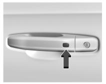
If equipped, the remote key must be within 1 m (3 ft) of the tailgate or door being opened or locked. Press the button on the door handle to open. See "Keyless Access Operation" in Remote Key Operation \$\display\$ 11.
