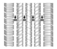
Treadwear indicators are one way to tell when it is time for new tires. Treadwear indicators appear when the tires have only 1.6 mm (1/16 in) or less of tread remaining. See *Tire Inspection* ♀ 391 and *Tire Rotation* ♀ 391.
