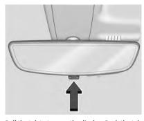
Pull the tab to turn on the display. Push the tab to turn it off. When off the mirror is automatic dimming. Adjust the mirror for a clear view of the area behind the vehicle while the display is off.
