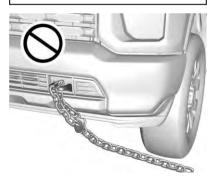
If the vehicle has recovery hooks at the front of the vehicle, use them if the vehicle is stuck off-road and needs to be pulled some place to continue driving.
