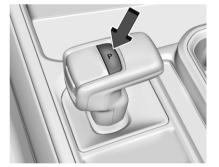
**P:** This position locks the rear wheels. Use P (Park) when starting the engine to prevent the vehicle from moving easily.
