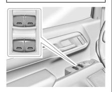
The power windows work when the vehicle is on, in accessory mode, or when Retained Accessory Power (RAP) is active. See *Retained Accessory Power (RAP)* ⇒ 218.
