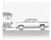
Only dinghy tow four-wheel-drive vehicles with a two-speed transfer case that have an N (Neutral) and a 4 \$\dpsi\$ (Four-Wheel Drive Low) setting.
