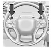
Electronic Range Select (ERS), or Manual Mode, allows for the selection of the range of gear positions. Use this mode when driving downhill or towing a trailer to limit the top gear and vehicle speed. The shift position indicator within the Driver Information Center (DIC) will display a number next to the L indicating the highest available gear.
