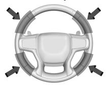
To begin steering manually, hold the steering wheel firmly with both hands using the highlighted regions.
