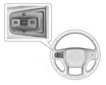
☼ : Press to turn cruise control on or off. A white indicator light comes on in the instrument cluster when cruise control is turned on. See Cruise Control Light \$\DDelta\$ 129. **+RES:** If there is a set speed in memory, press up briefly to resume to that speed or press and hold to accelerate. If cruise control is already engaged, use to increase the vehicle speed.
