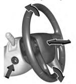
To adjust the steering wheel, if equipped:
