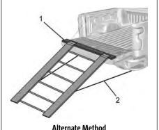
When applying any load to the tailgate, distribute the weight evenly across the width of the tailgate. This applies to all tailgate types.
