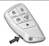
If the vehicle has the Keyless Access system, the remote key has a button on the side of the remote key used to remove the mechanical key. The mechanical key inside the remote key can
