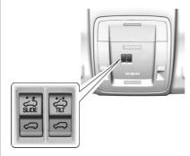
If equipped, the sunroof operates when the ignition is on or in ACC/ACCESSORY, or when Retained Accessory Power (RAP) is active. See *Retained Accessory Power* (RAP) ⇒ 271.
