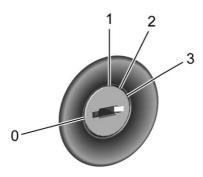
The ignition switch has four different positions.
