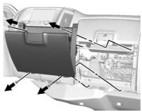
Close the lower glove box door and pull it from its frame to remove the entire unit.
