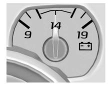
When the ignition is on, this gauge indicates the battery voltage.
