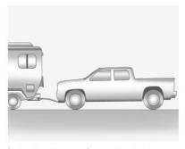
Only dinghy tow four-wheel-drive vehicles with a two-speed transfer case that have an N (Neutral) and a Four-Wheel Drive Low (4 (\$\d\cdot\$) setting.
