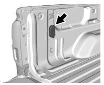
For vehicles with the fifth wheel/ gooseneck trailer package, the harness connector is mounted on the inside of the pickup bed behind the rear wheel.
