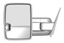
If equipped, adjust trailer-tow mirrors for a clear view of the area behind you. Manually pull out the mirror head to extend it for better visibility when towing a trailer.
