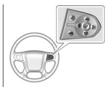
$\triangle$  or  $\nabla$ : Press to move up or down in a list. In the main view, press up and down to move between different info app pages.
