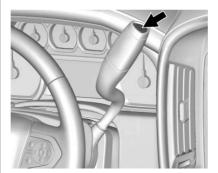
Vehicles with an automatic transmission have a Tow/Haul Mode. The Tow/Haul Mode adjusts the transmission shift pattern to
