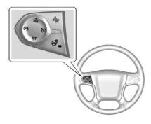
Fress to turn the system on or off. The indicator light is white when cruise control is on and turns off when cruise control is off.
