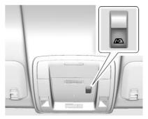
If equipped, the power sliding rear window works when the ignition has been turned to ACC/ACCESSORY or ON/RUN, or when Retained Accessory Power (RAP) is active. See Retained Accessory Power (RAP) ⇒ 271.
