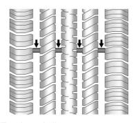
Treadwear indicators are one way to tell when it is time for new tires. Treadwear indicators appear when the tires have only 1.6 mm (1/16 in) or less of tread remaining. Some commercial truck tires may not have treadwear indicators. See *Tire Inspection* ♀ 412 and *Tire Rotation* ♀ 413 for additional information.
