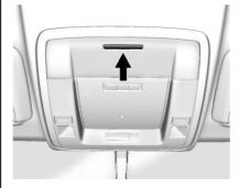
If equipped, sunglasses storage is on the overhead console. Press the fixed button on the cover and release to access.
