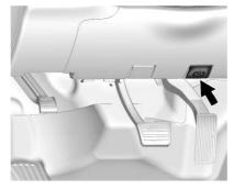
For vehicles with a release handle, set the parking brake by holding the regular brake pedal down, then pushing down the parking brake pedal.
