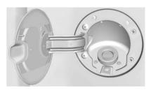
The vehicle has a capless refueling system and does not have a fuel cap. The filling nozzle must be fully inserted and latched prior to starting fuel flow.
