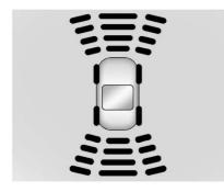
The instrument cluster may have a parking assist display with bars that show "distance to object" and object location information for the Parking Assist system. As the object gets closer, more bars light up and the bars change color from yellow to amber to red.
