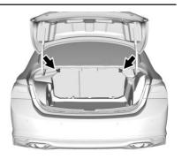
4. Open the trunk and pull the seatback release lever to fold the rear seat.
