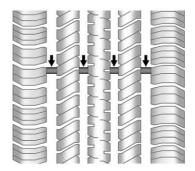
Treadwear indicators are one way to tell when it is time for new tires. Treadwear indicators appear when the tires have only 1.6 mm (1/16 in) or less of tread remaining. See *Tire Inspection* \$ 272 and *Tire Rotation* \$ 272 for additional information.
