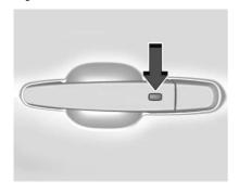
The RKE transmitter must be within 1 m (3 ft) of the trunk or door being opened. Press the button on the door handle to open. See "Keyless Access Operation" in Remote Keyless Entry (RKE) System Operation ⇔ 7.
