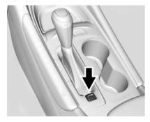
If equipped, the Electric Parking Brake (EPB) can always be applied, even if the vehicle is off. In case of insufficient electrical power, the EPB cannot be applied or released. To prevent draining the battery, avoid unnecessary repeated cycles of the EPB.
