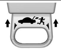
After pulling the emergency trunk release handle, push the handle back into the bezel.
