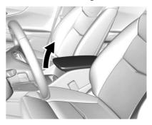
The center console has storage under the armrest. Pull up the latch and lift to open.
