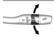
**INT**: Move the lever up to INT for intermittent wipes, then turn the band up for more frequent wipes or down for less frequent wipes.
