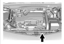
Lift the hood and release the hood prop rod from its retainer, in the front of the engine compartment. Securely insert the rod end into the slot marked with an arrow, on the underside of the hood.
