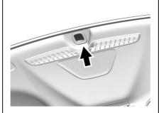
There is a light sensor on top of the instrument panel. Do not cover the sensor, otherwise the headlamps will come on when they are not needed.
