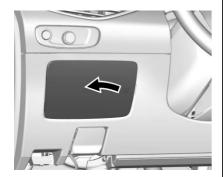
The instrument panel fuse block is on the driver side of the instrument panel. To access the fuses:
