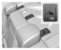
The top tether anchors are under the covers, behind the rear seat, on the filler panel. Be sure to use an anchor located directly behind the seating position where the child restraint will be placed.
