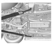
The vehicle is equipped with specific attachment points to be used by the towing provider. These holes may be used to pull the vehicle from a flat road surface onto the flatbed tow truck.
