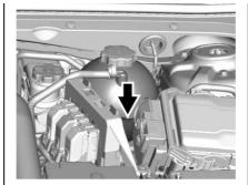
Check to see if coolant is visible in the coolant surge tank. If the coolant inside the coolant surge tank is boiling, do not do anything else until it cools down.
