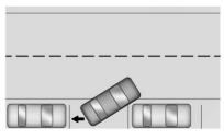
APA will instruct the vehicle to stop once a large enough space is found. Follow the displayed instructions. When instructed, shift to R (Reverse) to engage automatic steering. The steering wheel will briefly vibrate as a reminder to remove hands from the steering wheel. Check surroundings and continue braking or accelerating as needed, and be prepared to stop to avoid vehicles, pedestrians, or objects.
