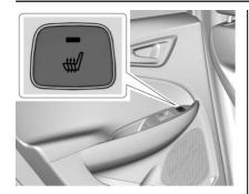
With the engine running, press ## to heat the left or right outboard seat cushion. An indicator light on the button will turn on when the heated seat is on. Press the button again to turn this feature off. The indicator will turn off.
