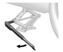
Raise the vehicle by turning the jack handle clockwise. Raise the vehicle far enough off the ground so there is enough room for the road tire to clear the ground.
