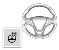
: If equipped with a heated steering wheel, press to turn on or off. A light on the button displays when the feature is turned on.
