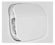
To open the fuel door, push and release the rearward center edge of the door.
