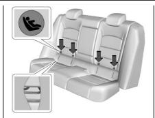
The outboard lower anchors are behind the vertical openings in the seat trim.
