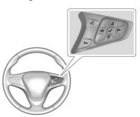
If equipped, some audio controls can be adjusted at the steering wheel.
