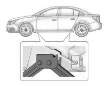
Position the jack lift head at the jack location nearest the flat tire. The location is indicated by a notch in the vertical bottom edge of the body side sheet metal.
