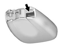
Separate the two halves of the transmitter using a flat tool inserted into the bottom center of the transmitter. Do not use the key slot.
