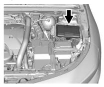
The engine compartment fuse block is on the driver side of the engine compartment.
