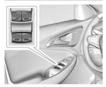
The power windows work when the vehicle is on, in ACC/ACCESSORY, or when Retained Accessory Power (RAP) is active. See Retained Accessory Power (RAP) ⇒ 186.
