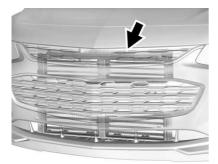
The vehicle may have a shutter system designed to help improve fuel economy. Keep the shutter system clear of debris,
