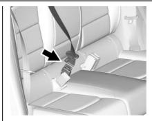
Disconnect the rear seat belt mini-latch, using a key in the slot on the mini-buckle.
