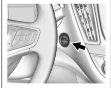
The vehicle has an electronic keyless ignition with pushbutton start.
