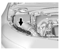
The electrical cord is on the passenger side of the engine compartment, between the fender and the air cleaner.
