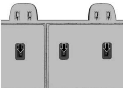
For models with a cargo cover, the top tether anchors are on the back of the rear seatbacks. Remove the cargo cover before installing the top tether. The cargo cover should remain off while the top tether is in
