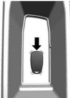
4. Open the center console. Place the transmitter in the backup location with the buttons facing down.
