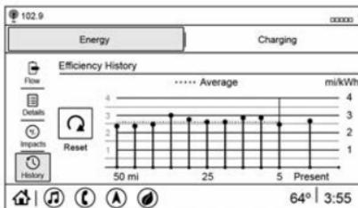
This screen displays a graph showing the energy efficiency that has been used over the last 50 km (50 mi). The Present point provides the average energy efficiency for the current 5 km (5 mi).
