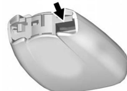
2. Separate the two halves of the transmitter using a flat tool inserted into the area near the key slot.
