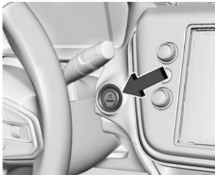
The vehicle has an electronic pushbutton start.
