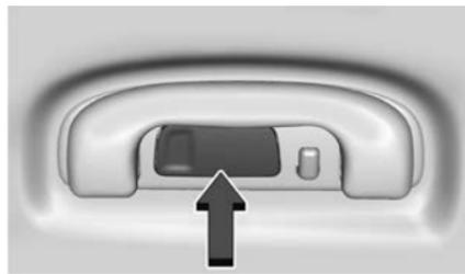
If equipped with sunroof, press the lamp lenses over the rear passenger doors.
