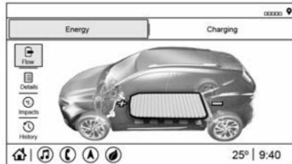
The Power Flow screen indicates the current operating condition. The screen shows energy flow to and from the high voltage battery while the vehicle is being driven. These components will be highlighted when they are active.
