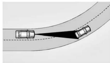
ACC may detect a vehicle that is not in your lane and apply the brakes.
