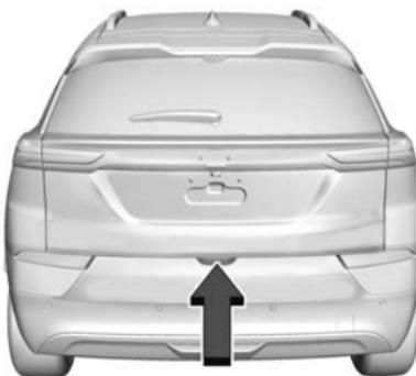
To open the liftgate, press the touch pad and lift up.
