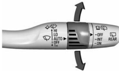
**AUTO** : When enabled, move the windshield wiper lever to AUTO.
