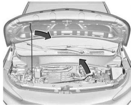
3. Lift the hood and release the hood prop rod from its retainer, in the front of the engine compartment. Securely insert the rod end into the slot marked with an arrow, on the underside of the hood.
