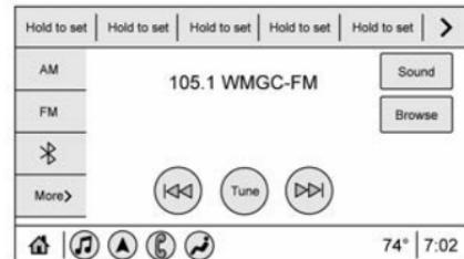
From the AM, FM, or SXM (if equipped) option, press  $\text{DN}$  or  $\text{UP}$  on the center stack to search for the previous or next strong station or channel.
