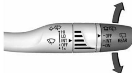
The controls are on the end of the windshield wiper lever.
