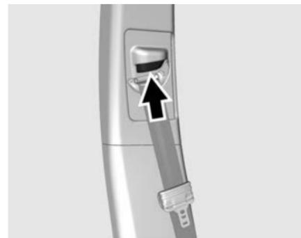
Press and hold the release button while raising or lowering the height adjuster to the desired position.
