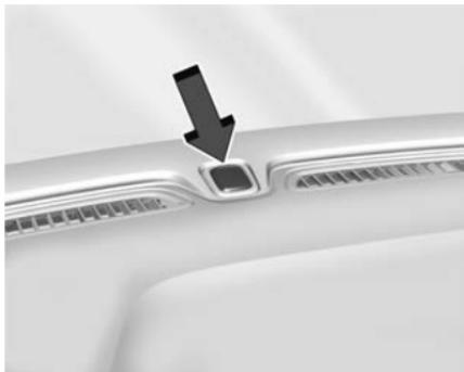
The red indicator light, on the instrument panel near the windshield, indicates the status of the system:
