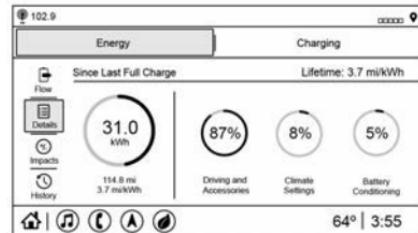
This screen displays how energy is being used since the last time the high voltage battery was fully charged. It includes Driving and Accessories, Climate Settings, and Battery Conditioning. The circle graph displays these percentages. Energy used, distance traveled, efficiency since last full charge, and lifetime efficiency are also displayed.
