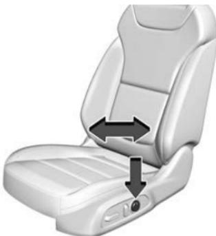
If equipped, press and hold the front or rear of the control to increase or decrease lumbar support.
