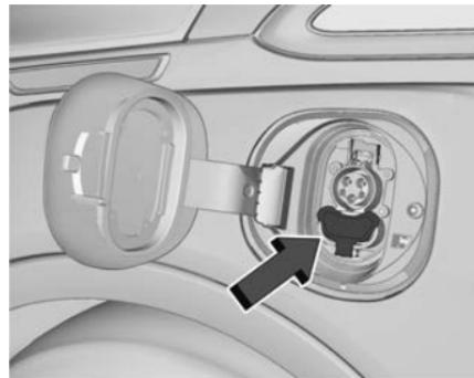
3. Unlatch the DC charging dust cover and lower it fully.
