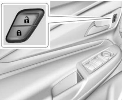
To lock or unlock the liftgate from the inside, press
