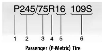
**(1) Passenger (P-Metric) Tire** : The United States version of a metric tire sizing system. The letter "P" as the first character in the tire size means a passenger vehicle tire engineered to standards set by the U.S. Tire and Rim Association.
