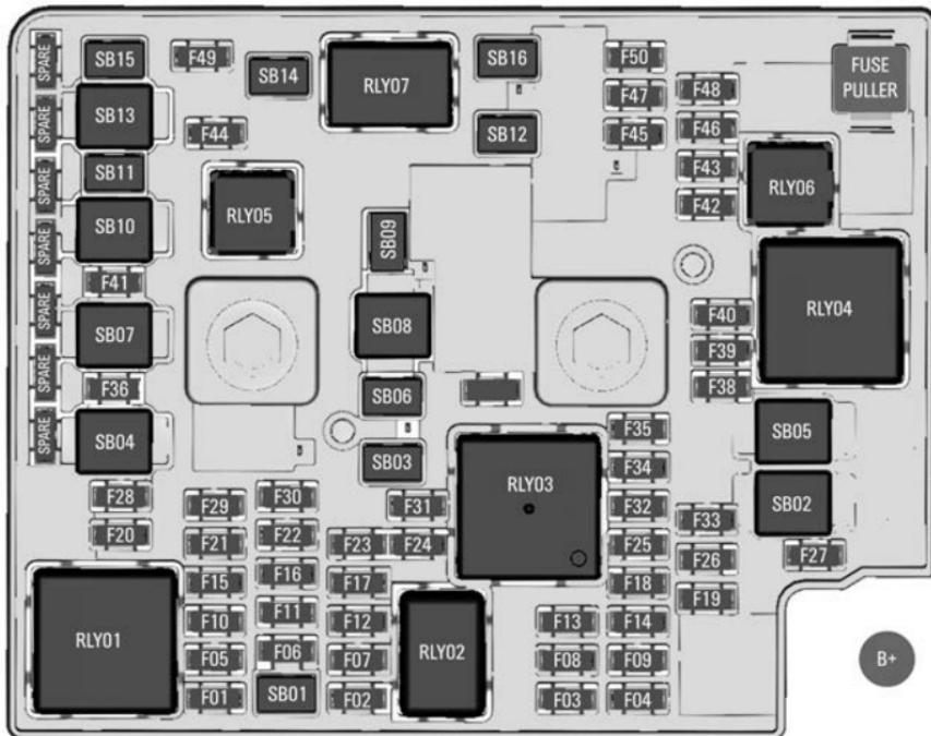
A fuse puller is in the underhood compartment fuse block.
