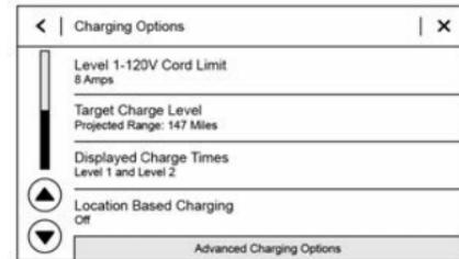
To view and change the Charging Options, touch Energy from the infotainment home screen, touch the Charging tab, and then touch Charging Options on the Charging Status screen. Use the arrows to scroll through the list, or hold and drag the list.
