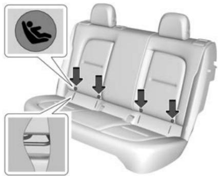
The outboard lower anchors are behind the vertical openings in the rear seat trim.
