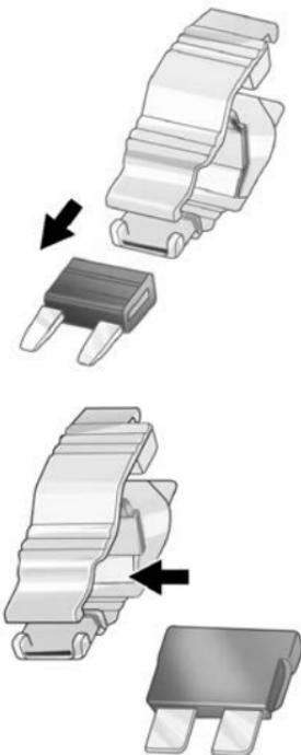
3. Use the fuse puller to remove the fuse from the top or side, as shown above.
