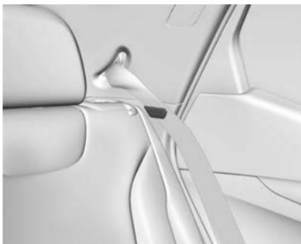
1. Make sure the seat belt is in the seat belt clip on the side trim of the vehicle.
