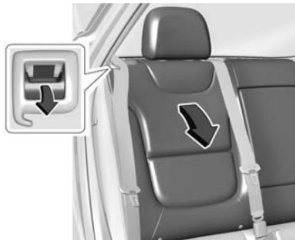
2. Pull the lever on top of the seatback to unlock the seatback.
