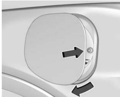
2. Push the rearward edge of the charge port door and release to open the door.
