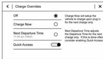
Delayed Charging can be temporarily overridden to an immediate charge for one charge cycle. Also, the next planned departure time can be temporarily overridden for one charge cycle. In addition to the in-vehicle overrides via the infotainment display, there are other ways to temporarily override a delayed charge mode. See *Plug-In Charging* ▷ 229.
