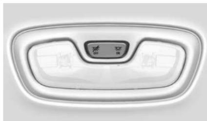
The rear reading lamps are in the headliner.
