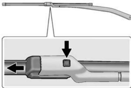
2. Press the button in the middle of the wiper arm connector, and pull the wiper blade away from the arm connector.
