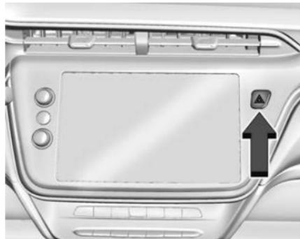
The hazard warning flasher button is on the center stack.
