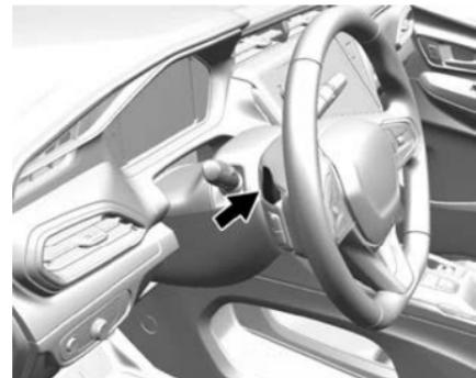
Regen on Demand allows increased deceleration by pressing and holding the steering wheel paddle. It works in D (Drive). Regen on Demand can add additional regenerative braking when One-Pedal Drive mode is enabled. The accelerator pedal can be used to manage deceleration while using Regen on Demand. See "One-Pedal Driving" under *Electric Drive Unit* ▷ 184.
