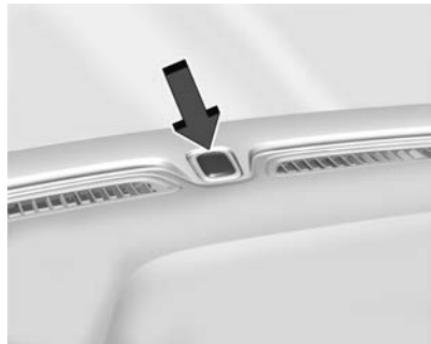
The vehicle has a Charging Status Indicator (CSI) at the center of the instrument panel near the windshield. When the vehicle is plugged in and vehicle power is off, the CSI indicates the following:
