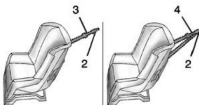
A top tether (3, 4) is used to secure the top of the child restraint to the vehicle. A top tether anchor is built into the vehicle. The top tether attachment hook (2) on the child restraint connects to the top tether anchor in the vehicle in order to reduce the forward movement and rotation of the child restraint while driving or in the event of a crash.
