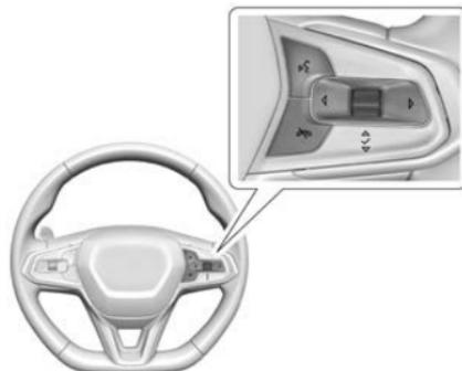
△ or ▽ : Move the thumbwheel up or down in a list.
