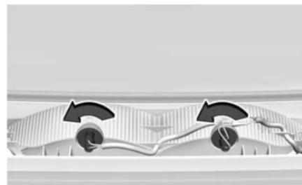
1. Turn the bulb socket counterclockwise and pull the bulb straight out of the socket.
