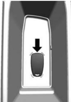
1. Open the center console. Place the two recognized transmitters in the backup location with the buttons facing down.
