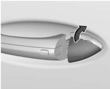
2. Rotate the cap upward and install into place.
