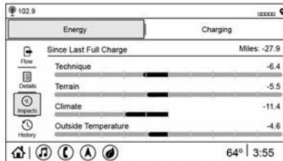
This screen provides an estimate of the factors that influence energy usage since the last full charge of the high voltage battery. Each factor is evaluated for energy gains or losses, and the total equivalent distance is indicated by the value on the upper right side of the screen. All values are reset after a complete charge.
