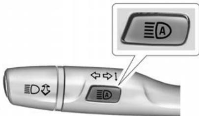
To enable the IntelliBeam system, press
