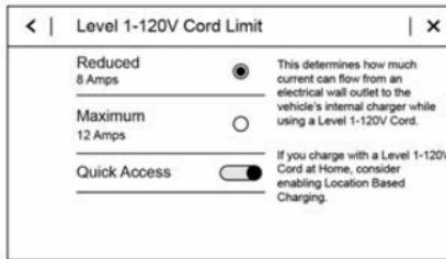
The Level 1-120V Cord Limit should be configured to match the electrical current rating for the electrical outlet that the charge cord is connected to. The Level 1-120V Cord Limit settings are:
