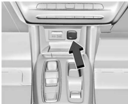
The vehicle has an accessory power outlet on the lower center stack below the climate control.
