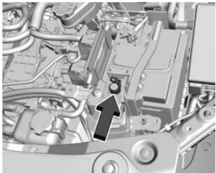
Remove the bracket and open the trim cover to expose the terminal.
