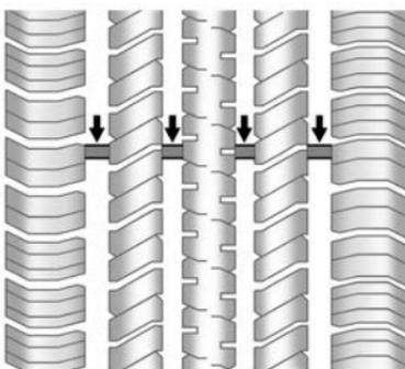
Treadwear indicators are one way to tell when it is time for new tires. Treadwear indicators appear when the tires have only 1.6 mm (1/16 in) or less of tread remaining. See *Tire Inspection* ▷ 270 and *Tire Rotation* ▷ 270 for additional information.
