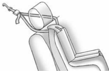
If the position you are using has an adjustable headrest or head restraint, adjust it accordingly to allow proper fitment. If you are using a single tether, route the tether in between the headrest or head restraint posts.
