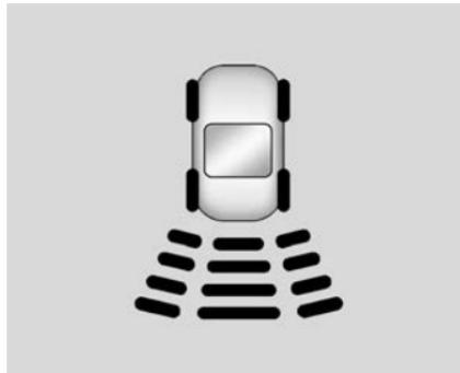
The instrument cluster may have a Park Assist display with bars that show "distance to object" and object location information for RPA. As the object gets closer, more bars light up and the bars change color from yellow to amber to red. When an object is first detected in the rear, one beep will be heard from the rear. When an object is very close, <0.6 m (2 ft) in the vehicle rear, five beeps will sound from the rear depending on object location.
