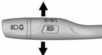
Move the lever all the way up or down to signal a turn.
