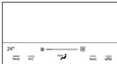
The climate control status display appears briefly when the climate control buttons on the center stack are adjusted. The air delivery mode can be adjusted on the climate control status display.
