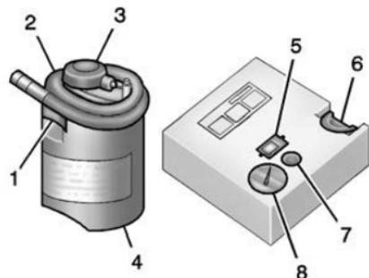
1. Sealant Canister Inlet Valve
