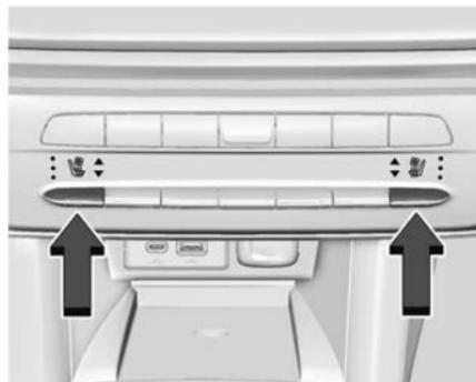
If equipped, the buttons are near the climate controls on the center stack. To operate, the vehicle must be on.
