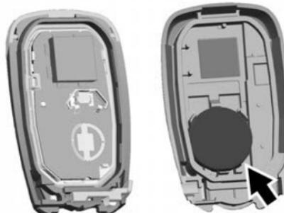
3. Remove the battery by pushing on the battery and sliding it toward the bottom of the transmitter.
