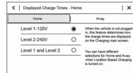
This feature determines how the charge times are displayed on the Charging Status screen. The selections for Home and Away can be different when location based charging is turned on.
