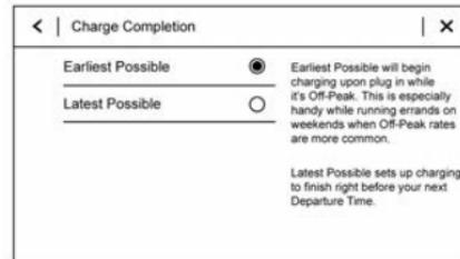
When the cost would be the same, based on utility rates, the earliest or latest possible time for a charge to complete can be selected. For example, if Off-Peak charge time is 12 am to 6 am and only three hours of charge are needed, Earliest Possible would start charging at 12 am and Latest Possible would start charging at 3 am. Use the Earliest Possible setting to charge as soon as possible. Use the Latest Possible setting to optimize energy usage.
