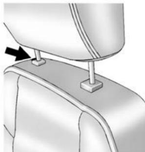
To lower the head restraint, press the button on the top of the seatback and push the head restraint down. Try to move the head restraint after the button is released to make sure it is locked in place.
