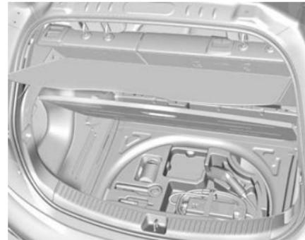
Pull up on the load floor cover to access the cargo management system, if equipped.
