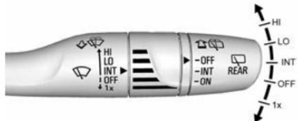
The windshield wiper/washer lever is on the side of the steering column. With the vehicle on, move the windshield wiper lever to select the wiper speed.
