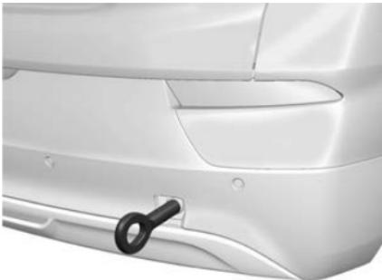
Install the tow eye into the socket and turn it until it is fully tightened. When the tow eye is removed, reinstall the cover with the notch in the original position.
