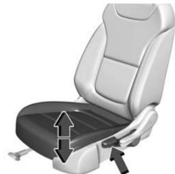
Move the lever on the outboard side of the seat up or down to manually adjust the seat height.
