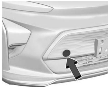
Carefully open the cover in the fascia by using the small notch that conceals the tow eye socket.
