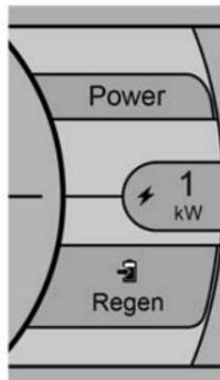
The power indicator gauge is on the right side of the display in the Enhanced layout.
