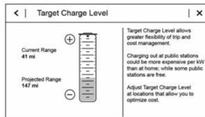
Touch + or – to increase or decrease the charge level, or drag the dark horizontal white line up and down on the graphic to the desired level.
