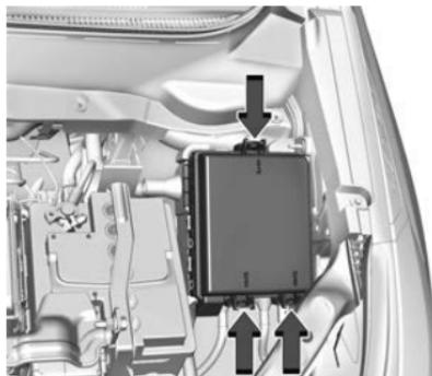
To open the fuse block cover, press the clips at the side and back and pull the cover up.
