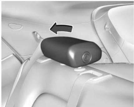
4. Return the head restraint to the full upright position if folded. Pull the head restraint up and forward until it locks into place.
