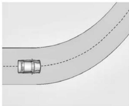
When entering a curve, Super Cruise may not detect the lane markings and may not adjust the steering enough to stay in your lane of travel. When this happens, you will need to steer the vehicle.
