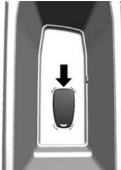
1. Open the center console. Place the transmitter in the backup location with the buttons facing down.
