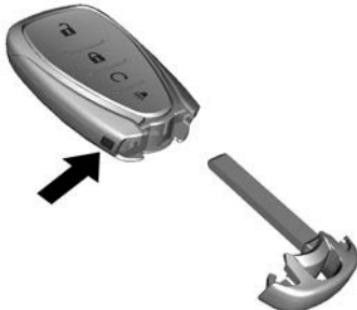
1. Press the button on the side of the transmitter near the bottom and pull the key out. Never pull the key out without pressing the button.
