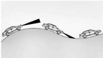
Do not use ACC when driving on steep hills or when towing a trailer. ACC will not detect a vehicle in the lane while driving on steep hills. If the brakes are applied, ACC disengages.
