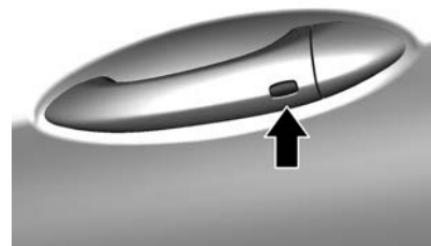
Pressing the lock/unlock button will cause all doors to lock if any of the following occur:
