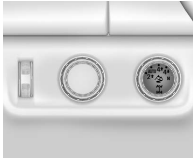
Transfer Case Knob with Off-Road Mode
