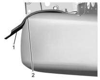
Make sure the tire is stored securely and flush in the radius (2) of the spare tire support bracket (1). Push, pull, and then try to turn the tire. If the tire moves, use the wheel wrench to tighten the cable.
