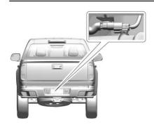
The RVC is disconnected by disconnecting the connector behind the rear license plate.
