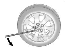
Use the wheel wrench and turn it counterclockwise to loosen the wheel nuts. Do not remove the wheel nuts yet.
