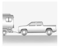
Only dinghy tow four-wheel-drive vehicles that have an N (Neutral) and a Four-Wheel Drive Low (4 (1) setting.
