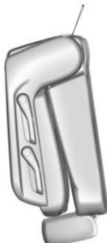
3. Pull the strap again to release the rear of the seat from the floor. The seat will tumble forward.
