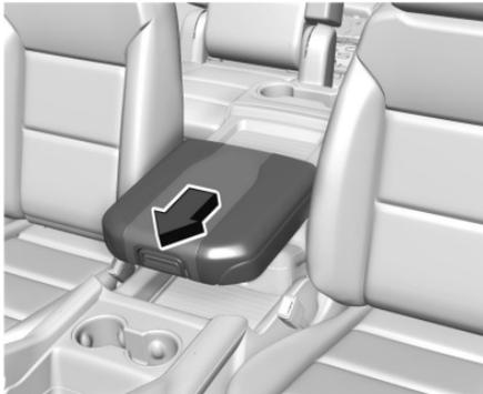
To move the armrest forward, push forward on the center of the armrest with the palm of your hand.
