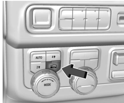
If equipped, select Terrain mode by pressing the
