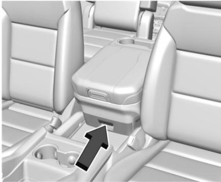
When the center console is all of the way back, there is a storage bin under the armrest. Pull on the handle to open.
