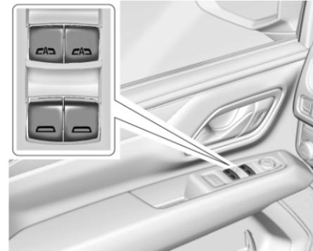
The power windows work when the vehicle is on, in accessory mode, or when Retained Accessory Power (RAP) is active. See *Retained Accessory Power (RAP)* ⇨ 198.
