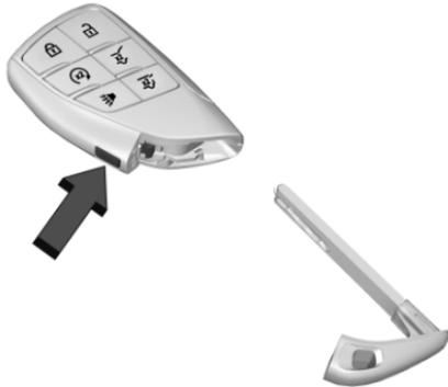
1. Press the button on the side of the remote key and pull the mechanical key out. Never pull the mechanical key out without pressing the button.
