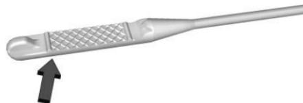
If the oil is below the cross-hatched area at the tip of the dipstick and the engine has been off for at least 15 minutes, add 1 L (1 qt) of the recommended oil and then recheck the level. See “Selecting the Right Engine Oil” later in this section for an explanation of what kind of oil to use. For engine oil crankcase capacity, see *Capacities and Specifications* ⇨ 402.
