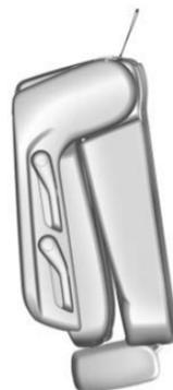
3. Lift the lever again to release the rear of the seat from the floor. The seat will tumble forward.
