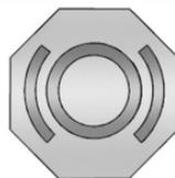
The brake master cylinder reservoir is filled with GM approved DOT 4 brake fluid as indicated on the reservoir cap. See *Engine Compartment Overview* ⇨ 314 for the location of the reservoir.
