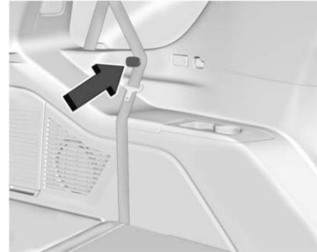
6. Stow the seat belt in the belt stowage clip. Repeat the steps to fold the other seatback, if desired.
