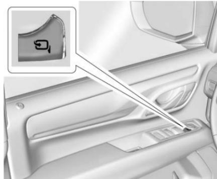
To adjust power folding mirrors, if equipped:
