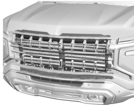
The vehicle may have a shutter system designed to help improve fuel economy. Keep the shutter system clear of debris, snow, and ice. The check engine light may activate if the shutter system is blocked.
