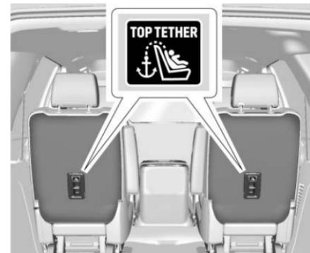
For models with bucket second row seating, the top tether anchors are on the rear of the seatback for each seating position in the second row. Be sure to use an anchor located directly behind the seating position where the child restraint will be placed.
