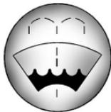
Open the cap with the washer symbol on it. Add washer fluid until the tank is full. See *Engine Compartment Overview* ⇨ 314 for reservoir location.
