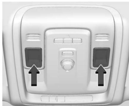
The front reading lamps are in the overhead console. Press the lamp lenses to turn the front reading lamps on or off.
