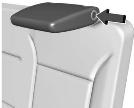
The head restraint will fold forward automatically.
