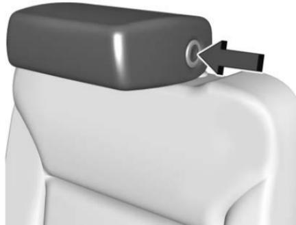
The head restraint will fold forward automatically.
