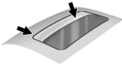
Dirt and debris may collect on the sunroof seal or in the track. This could cause an issue with sunroof operation or noise. It could also plug the water drainage system. Periodically open the sunroof and remove any obstacles or loose
