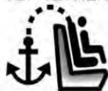
To assist in locating the top tether anchors, the top tether anchor symbol is near the top tether anchors.
