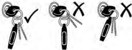
The ignition key and key rings, and RKE transmitter, if equipped, are designed to work together as a system to reduce the risk of unintentionally moving the key out of the RUN position. The ignition key has a small hole to allow attachment of the provided key ring.
