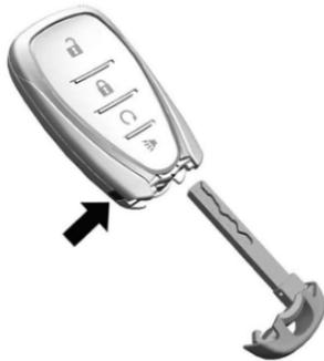
To remove the key, press the button on the side of the RKE transmitter and pull the key out. Never pull the key out without pressing the button.
