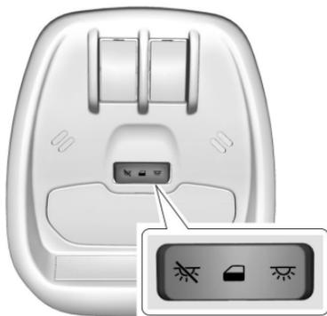
The front dome lamp controls are in the overhead console.
