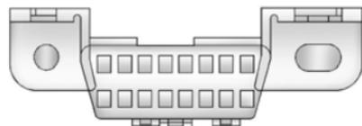
The DLC is under the instrument panel to the left of the steering wheel. Connecting devices that are not used to perform an Emissions Inspection/Maintenance test or to service the vehicle may affect vehicle operation. See *Add-On Electrical Equipment* ⇨ 215. See your dealer if assistance is needed.
