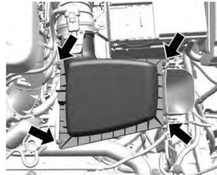
3. Remove four screws, tilt the cover, and slide it out of the assembly.
