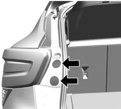
2. Pull the taillamp assembly straight back to detach it from the vehicle body. Take care that the cable duct remains in place.
