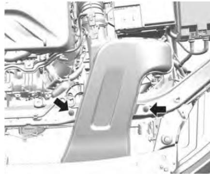
1. Remove the two push pins.
