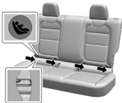
The lower anchors are behind the vertical openings in the seat cushion trim located below the anchor label.
