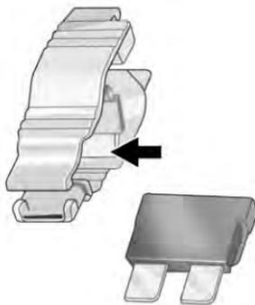
3. Use the fuse puller to remove the fuse from the top or side.
