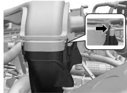
2. Disassemble the duct.
