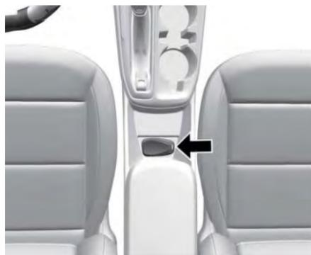
3. Remove the two recognized transmitters from transmitter pocket. Place the new transmitter in transmitter pocket.
