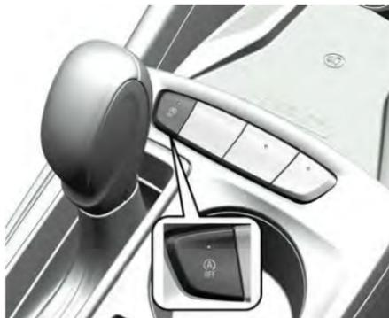
The automatic engine stop/start feature can be disabled and enabled by pressing
