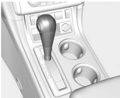
**P (Park):** This position locks the front wheels. It is the best position to use when starting the engine because the vehicle cannot move easily.
