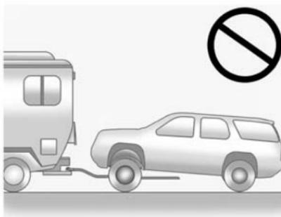
All-wheel-drive vehicles must not be towed with two wheels on the ground. To properly tow these vehicles, they should be placed on
