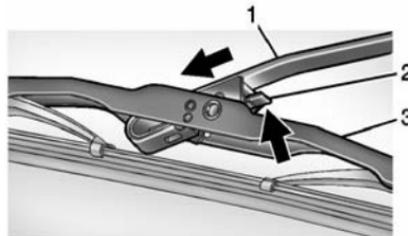
2. Push the release lever (2) to disengage the hook and push the wiper arm (1) out of the blade assembly (3).
