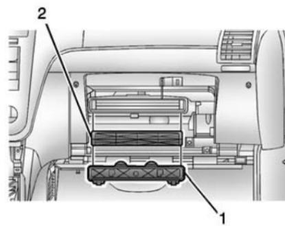
5. Squeeze the housing cover (1) tabs to remove.
