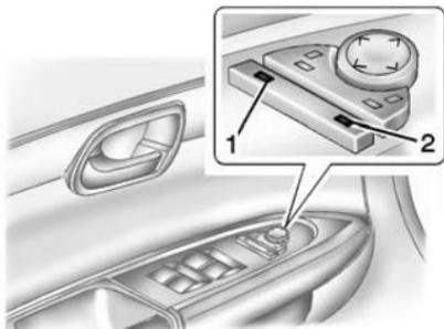
1. Press (1) to fold the mirrors out to the driving position.
