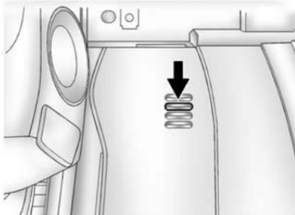
The interior temperature sensor, on the instrument panel to the right of the steering column, measures the temperature of the air inside the vehicle.
