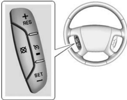
**(On/Off):** Press to turn cruise control on or off. The indicator light on the button comes on when the cruise control is on.
