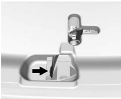
2. At the front of the vehicle, pull up on the center of the hood, and push the secondary hood release to the right.
