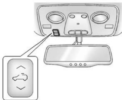
**Vent:** Press the front or rear of the switch to vent or close the sunroof.
