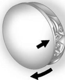
The fuel cap is behind a hinged fuel door on the driver side of the vehicle. To open the fuel door, push and release the rearward center edge of the door.
