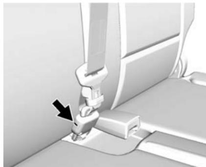
3. Disconnect the rear safety belt mini-latch, using a key in the slot on the mini-buckle, and let the belt retract into the headliner. Stow the mini-latch in the holder in the headliner.
