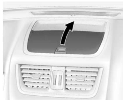
This vehicle has an instrument panel storage area. To open the cover, pull the latch forward.
