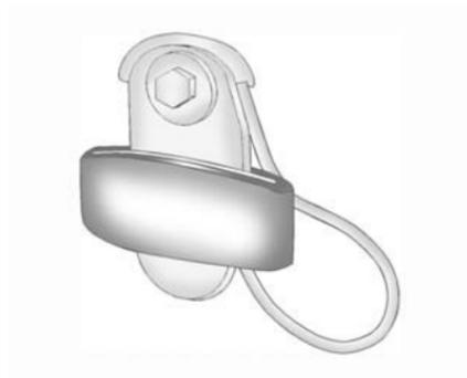
1. Remove the guide from its storage clip on the interior trim next to the outboard seatback.
