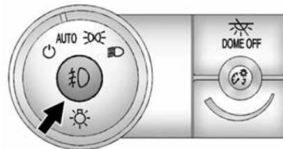
For vehicles with front fog lamps, the fog lamp button is on the exterior lamp control to the left of the steering column.
