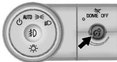
The instrument panel brightness knob is located on the instrument panel to the left of the steering column.
