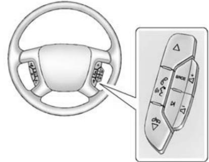
Vehicles with audio steering wheel controls could differ depending on the vehicle's options. Some audio controls can be adjusted at the steering wheel.
