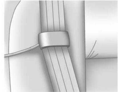
3. Be sure that the belt is not twisted and it lies flat. The elastic cord must be behind the belt with the plastic guide on the front.
