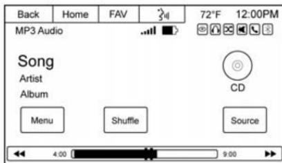
Press the Menu screen button while that source is active to access the MP3 Audio Menu.
