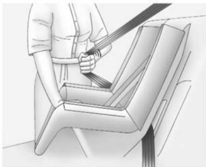
4. Pull the shoulder belt all the way out of the retractor to set the lock. When the retractor lock is set, the shoulder belt can be tightened but not pulled out of the retractor.
