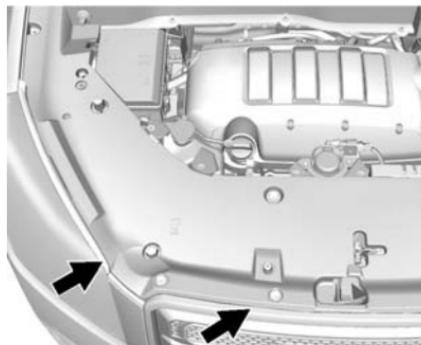
1. Detach the fasteners and lift off the panel that covers the radiator cap.
