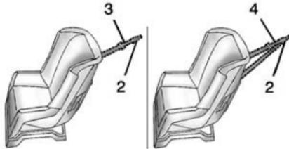
A top tether (3, 4) anchors the top of the child restraint to the vehicle. A top tether anchor is built into the vehicle. The top tether attachment (2) on the child restraint connects to the top tether anchor in the vehicle in order to reduce the forward movement and rotation of the child restraint during driving or in a crash.
