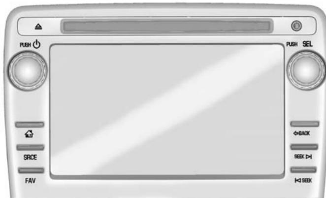
**PUSH/⏻** : Press to turn the system on and off. Turn to adjust the volume.
