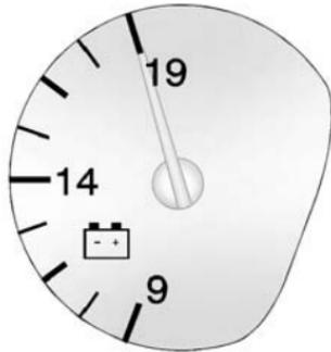
When the engine is not running, but the ignition is on, this gauge displays the battery voltage in DC volts.
