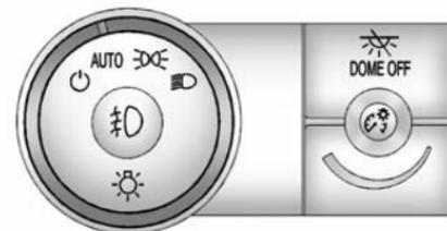
The exterior lamp control is on the instrument panel to the left of the steering wheel.
