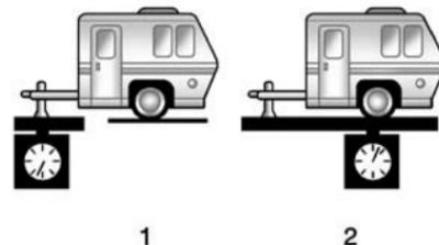
If a weight-carrying hitch or a weight-distributing hitch is being used, the trailer tongue (1) should weigh 10-15 percent of the total loaded trailer weight (2).
