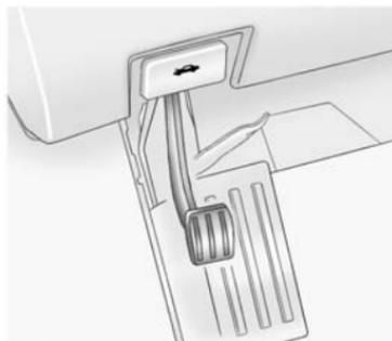
To set the parking brake, hold the regular brake pedal down, then push the parking brake pedal down.
