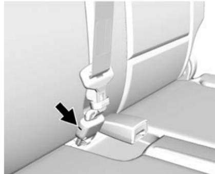
2. Disconnect the rear safety belt mini-latch using a key in the slot on the mini-buckle, and let the belt retract into the headliner. Stow the mini-latch in the holder in the headliner.
