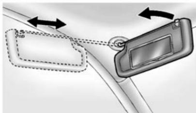
Pull the sun visor down to block glare. Detach the sun visor from the center mount to pivot to the side window or, if equipped, extend along the rod.
