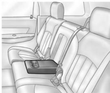
If equipped, the rear seat armrest may have two cupholders. Pull the armrest down to access the cupholders.
