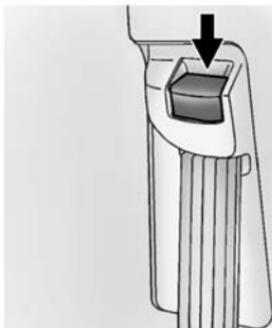
To move it down, push down on the release button and move the height adjuster to the desired position. You can move the height adjuster up by pushing up on the shoulder belt guide.
