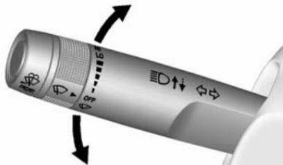
Move the turn signal lever all the way up or down to signal a turn.
