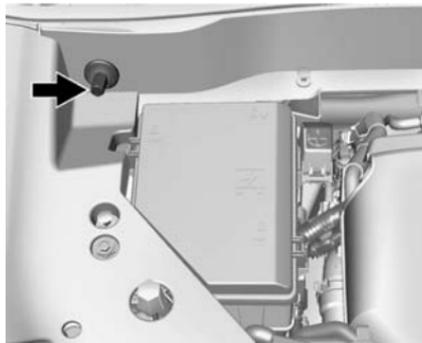
9. Connect the other end of the negative (-) cable to the remote negative (-) terminal of the dead battery.
