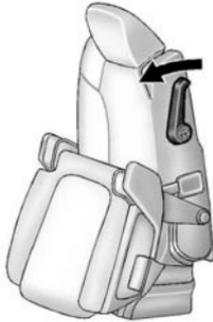
The second row seat can be folded to access the third row. Pull the sliding seat lever forward; the seat cushion folds, and the seat slides forward.
