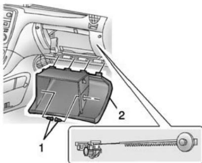
2. Twist the compartment retainers (1) and pull outward to remove.
