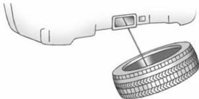
5. Tilt the retainer and slip it through the wheel opening to remove the spare tire from the cable.
