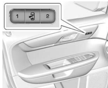
If equipped, the controls on the driver door are used to program and recall memory settings for the driver seat and outside mirrors.
