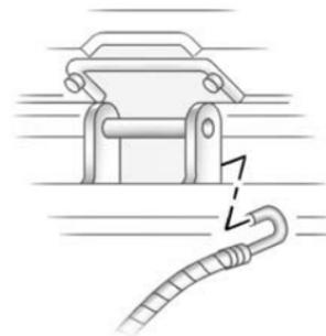
5. Hook the cable onto the outside portion of the liftgate hinges (2).
