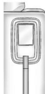
4. Pull up on the release lever on the back of the seat.
