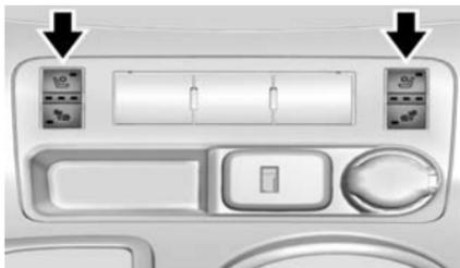
Heated and Cooled Seat Buttons Shown, Heated Seat Buttons Similar
