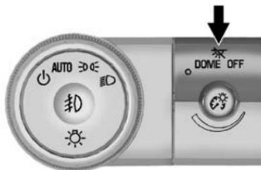
The dome lamp override button is next to the exterior lamps control.
