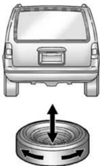
6. Make sure the tire is stored securely. Push, pull, and then try to turn the tire. If the tire moves, use the wrench to tighten the cable.
