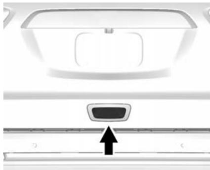
To open the liftgate, press the touch pad under the liftgate handle and lift up. The vehicle must be in P (Park) and the battery must be charged. Use the pull cup or pull strap to lower and close the liftgate.
