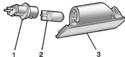
4. Turn the bulb socket (1) counterclockwise to remove it from the lamp assembly (3).
