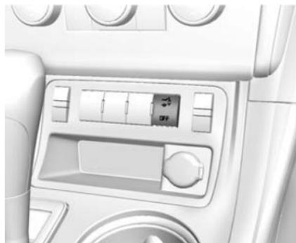
To change the liftgate to manual operation, press OFF on the power liftgate switch. A message displays on the DIC indicating manual operation mode. See *Door Ajar Messages on page 5-35*.
