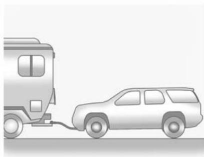
If the vehicle is front-wheel-drive, it can be dinghy towed from the front. These vehicles may also be towed by putting the front wheels on a dolly. See “Dolly Towing” later in this section.
