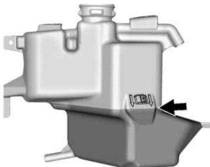
5. Fill the coolant recovery tank to the FULL COLD mark or to the FULL COLD ISO symbol mark.
