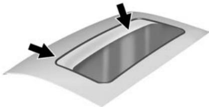
Dirt and debris may collect on the sunroof seal or in the track. This could cause an issue with sunroof operation or noise. It could also plug the water drainage system. Periodically open the sunroof and remove any obstacles or loose debris. Wipe the sunroof seal and roof sealing area using a clean cloth, mild soap, and water. Do not remove grease from the sunroof.
