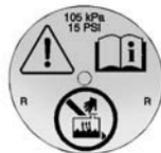
2. Remove the radiator pressure cap when the cooling system, including the upper radiator hose, is no longer hot. Turn the pressure cap slowly counterclockwise about one full turn.
