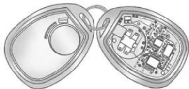
1. Separate the transmitter with a flat, thin object, such as a flat head screwdriver.
