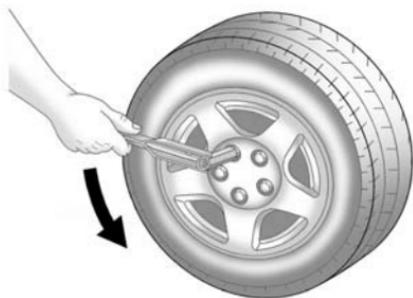
3. Loosen the wheel nuts — but do not remove them — using the wrench. For wheels with a wheel lock key, use the wheel lock key between the lock nut and wrench. The key is supplied in the front passenger door pocket.
