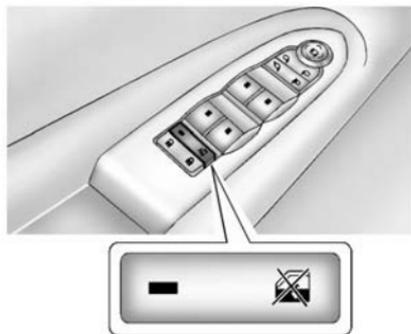
The rear window lockout feature prevents the rear passenger windows from operating, except from the driver position.
