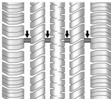
Treadwear indicators are one way to tell when it is time for new tires. Treadwear indicators appear when the tires have only 1.6 mm (1/16 in) or less of tread remaining. See *Tire Inspection on page 10-48* and *Tire Rotation on page 10-49*.
