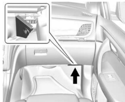
The instrument panel fuse block is under the instrument panel on the passenger side of the vehicle. Pull down on the cover to access the fuse block.
