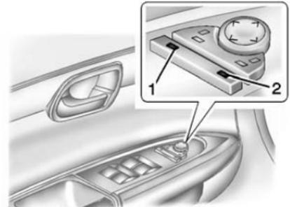
1. Press (1) to fold the mirrors out to the driving position.
