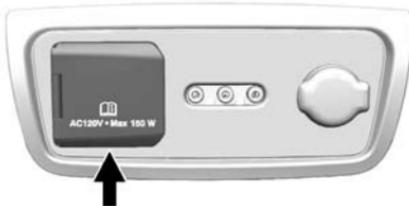
The power outlet is on the rear of the center console.
