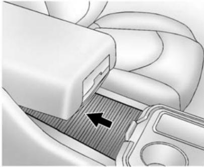
There is additional storage under the armrest. Move the armrest all the way to the rear position, then slide the storage cover back to access.
