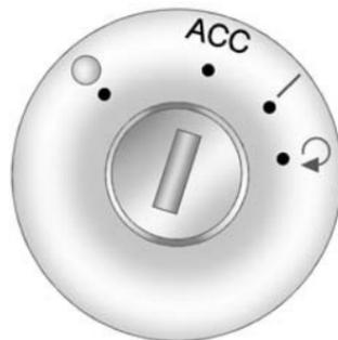
The ignition switch has four different positions.
