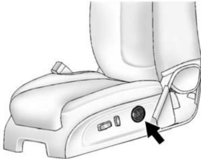
If equipped, press and hold the front or rear of control to increase or decrease lumbar support. Release the control when the seatback reaches the desired level of lumbar support.
