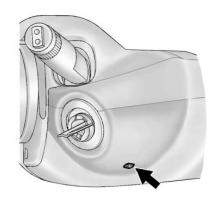
Vehicles with an automatic transmission are equipped with an electronic key lock release system. The key lock release is designed to prevent ignition key removal unless the shift lever is in P (Park).
