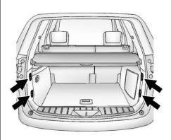
The vehicle may be equipped with four cargo tie-downs located in the rear compartment.
