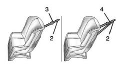
A top tether (3, 4) anchors the top of the child restraint to the vehicle. A top tether anchor is built into the vehicle. The top tether attachment (2) on the child restraint connects to the top tether anchor in the vehicle in order to reduce the forward movement and rotation of the child restraint during driving or in a crash.
