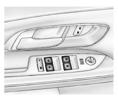
The power windows work when the ignition is in ON/RUN or ACC/ACCESSORY, or in Retained Accessory Power (RAP). See Retained Accessory Power (RAP) on page 9-22.
