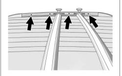
The roof rack cross rails can be locked in four positions along the roof rack side rails. These are the only positions that the cross rails will lock.
