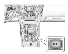
Press the "eco" (economy) button by the shift lever to turn this feature on or off. The "eco" light in the instrument cluster will come on when engaged. See *Fuel Economy Light on page 5-20*. A Driver Information Center (DIC) message "ECO MODE ON" is also displayed. See *Fuel System Messages on* page 5-28 for more information.
