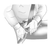
To unlatch the belt, push the button on the buckle.
