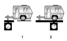
If a weight-carrying hitch or a weight-distributing hitch is being used, the trailer tongue (1) should weigh 10 to 15 percent of the total loaded trailer weight (2).
