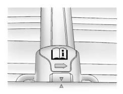
Push the lever down to completely engage into the side rail holes. If the lever is not tight, then the cross rail is not engaged in a side rail hole.
