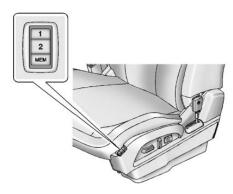
If available, the "1" and "2" buttons on the outboard side of the driver seat are used to manually save and recall the driver seat and outside mirror positions. These manually stored positions are referred to as Button Memory positions.
