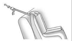
If the position being used does not have a headrest or head restraint and a single tether is being used, route the tether over the seatback.
