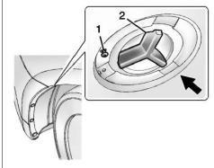
2. Remove screw (1) and turn access port cap (2) counterclockwise to remove.
