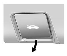
1. Pull the release handle located below the instrument panel to the left of the steering wheel.
