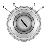
The ignition switch has four different positions.
