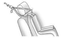
If the position being used has a fixed headrest or head restraint and a dual tether is being used, route the tether around the headrest or head restraint.
