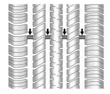
Treadwear indicators are one way to tell when it is time for new tires. Treadwear indicators appear when the tires have only 1.6 mm (1/16 in) or less of tread remaining. See *Tire Inspection on page 10-48* and *Tire Rotation on page 10-49*.
