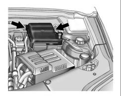
To remove the fuse block cover, squeeze the clips on the cover and lift it straight up. See *Engine* Compartment Overview on page 10-5.
